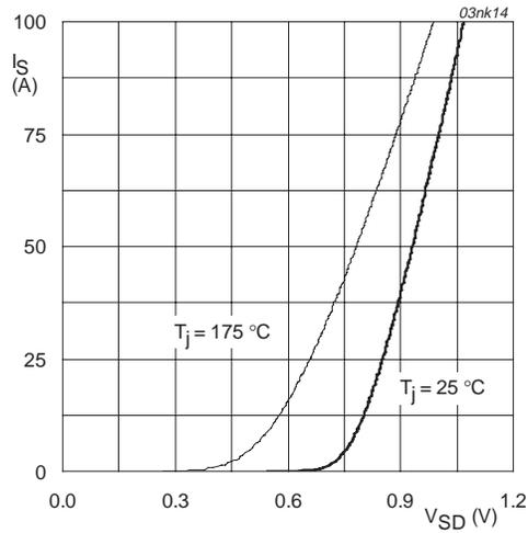
$V_{GS} = 0\text{ V}$
