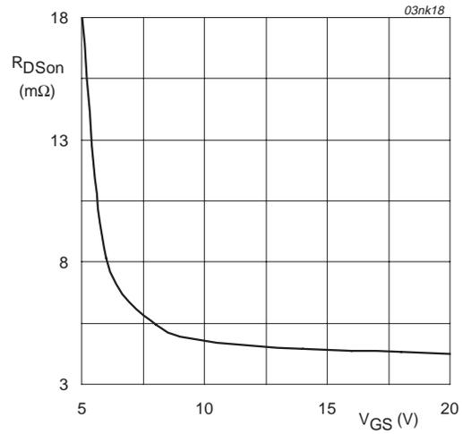
$T_j = 25^\circ\text{C}$ ;  $I_D = 25 \text{ A}$
