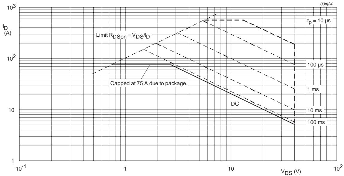
$T_{mb} = 25^{\circ}C$ ;  $I_{DM}$  single pulse.
