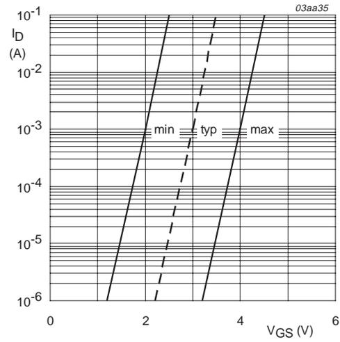
$T_j = 25 \text{ °C}; V_{DS} = V_{GS}$
