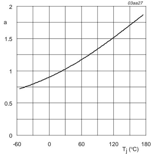
$$a = \frac{R_{DSon}}{R_{DSon}(25^\circ\text{C})}$$
