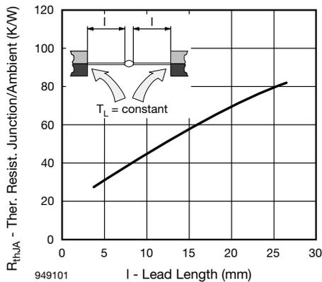
Fig. 1 - Typ. Thermal Resistance vs. Lead Length
