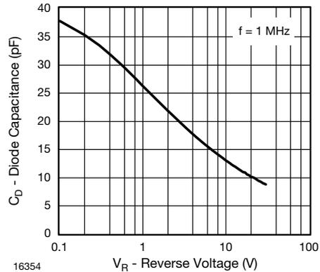
Fig. 6 - Diode Capacitance vs. Reverse Voltage
