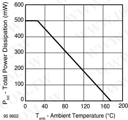
Figure 2. Total Power Dissipation vs. Ambient Temperature
