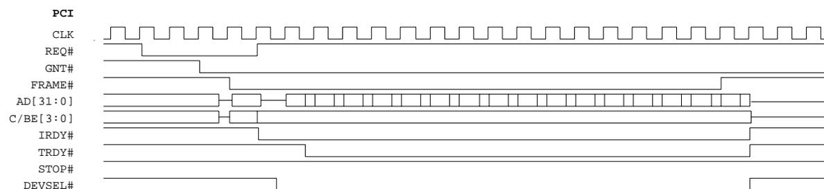
**Figure 41: Multiple PCI Read Transactions During DMA Operation**
