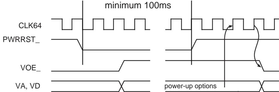
The power-up options are subsequently loaded into their respective registers several PCI clock periods after PWRRST\_, SYSRST\* and RST\_ have all been negated.
