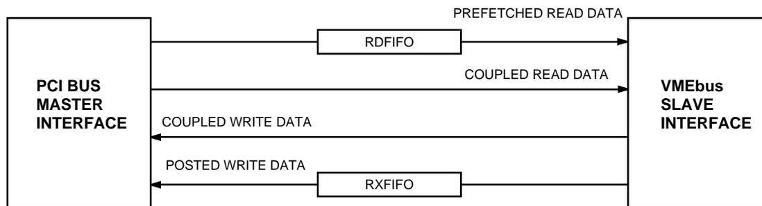
Incoming cycles from the VMEbus can have data widths of 8-bit, 16-bit, 32-bit, and 64-bit. Although the PCI bus supports only two port sizes (32-bit and 64-bit), the byte lanes on the PCI bus can be individually enabled, which allows each type of VMEbus transaction to be directly mapped to the PCI data bus.
