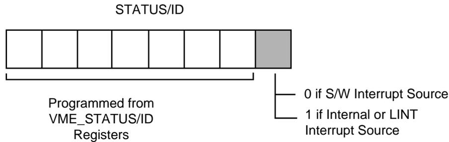
Once the Universe II has provided the STATUS/ID to an interrupt handler during a software initiated VMEbus interrupt, it generates an internal interrupt, SW\_IACK. If enabled, this interrupt feeds back to the PCI bus (through one of the LINT\_ pins) to signal a process that the interrupt started through software has been completed.
