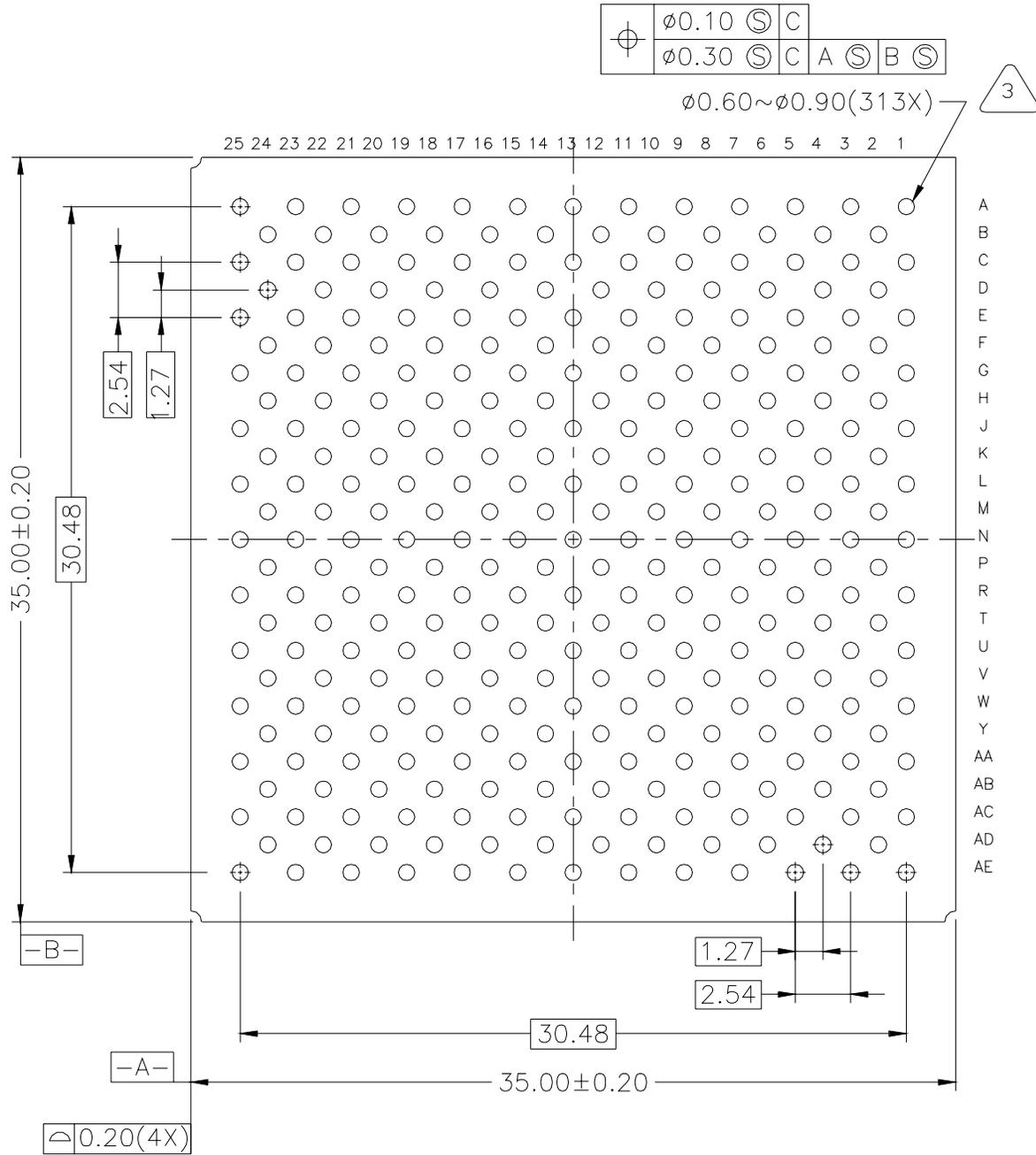
Figure 25: 313 PBGA - Top and Side View
