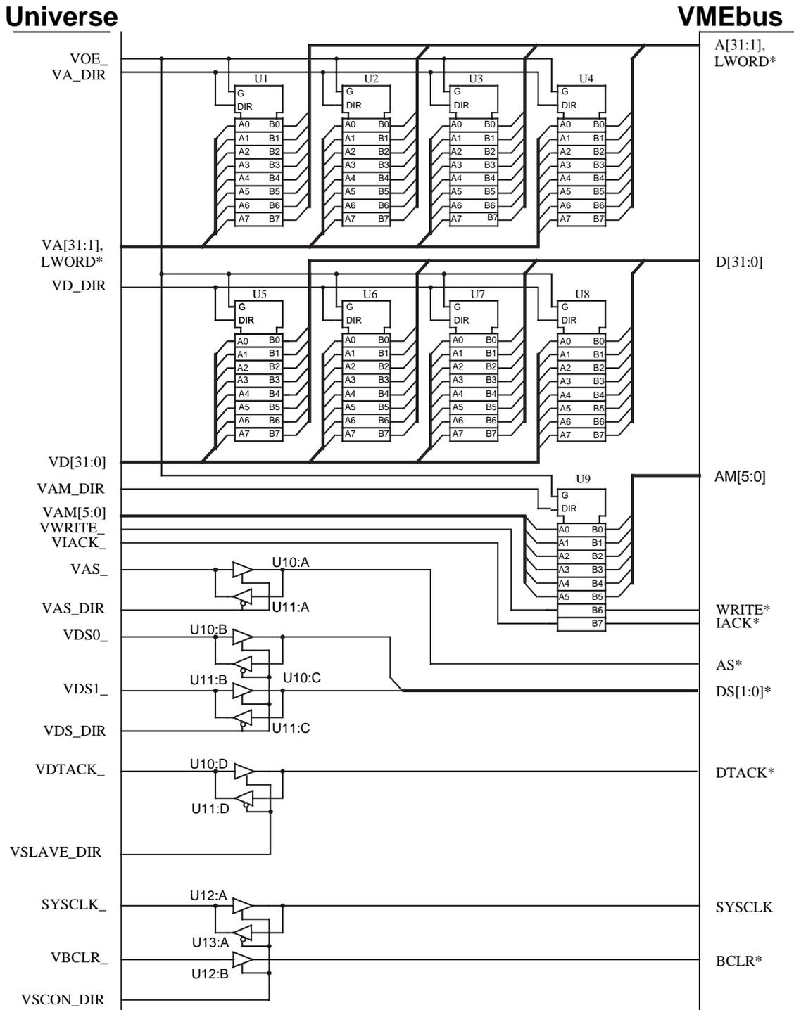
**Figure 43: Universe II Connections to the VMEbus Through TTL Buffers**
