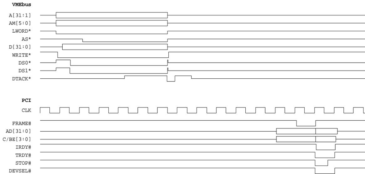
**Figure 37: BLT Decoupled Write Cycle - Universe II as VME Slave**
