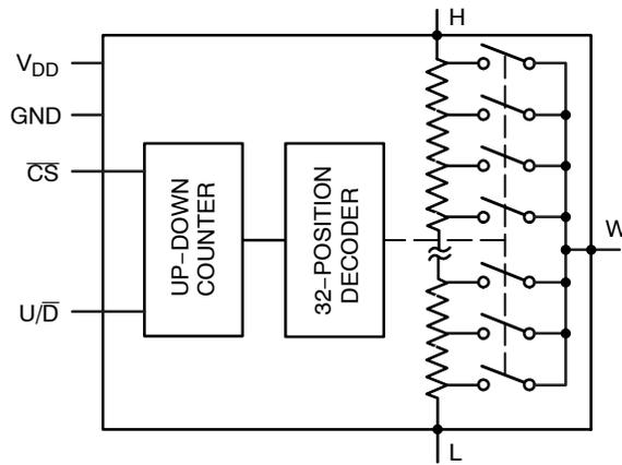
Figure 1. Functional Diagram
