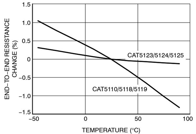
Figure 3. Change in End-to-End Resistance vs. Temperature
