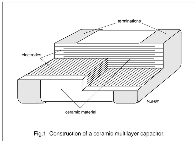
Fig.1 Construction of a ceramic multilayer capacitor.
