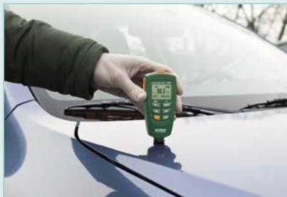
Measuring the thickness of automotive paint
