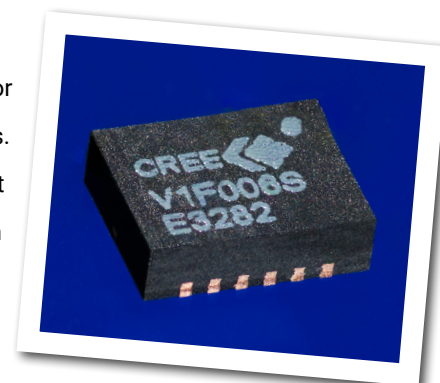
Package Type: 3x4 DFN PN: CGHV1F006S
