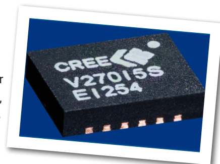
Package Type: 3x4 DFN PN: CGHV27015S
