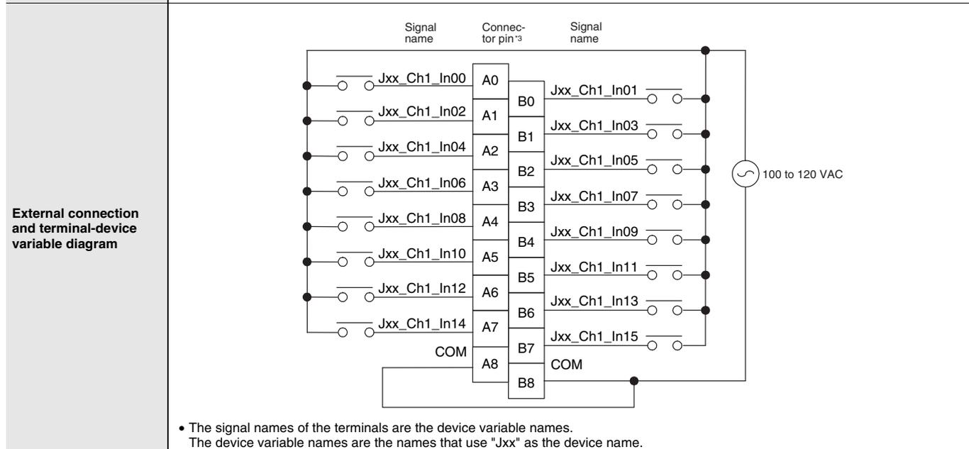
\*1. Can be set to 0 ms, 0.5 ms, 1 ms, 2 ms, 4 ms, 8 ms, 16 ms, or 32ms in the settings. When the response times have been set to 0 ms, the ON response time will be 10 ms maximum and the OFF response time will be 40 ms maximum due to internal element delays.
