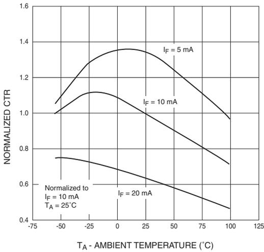
**Fig. 4 Normalized CTR vs. Ambient Temperature (White Package)**
