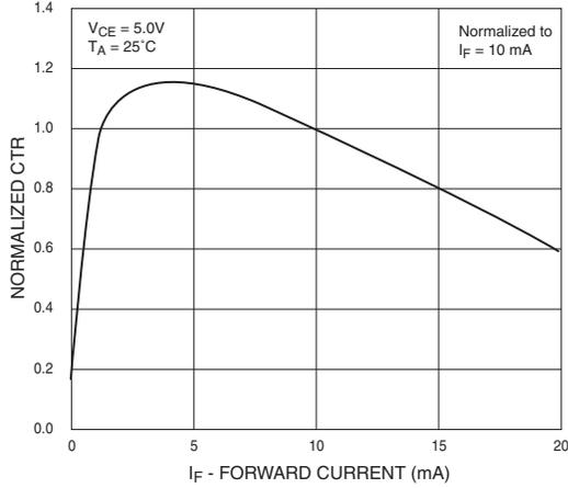
**Fig.2 Normalized CTR vs. Forward Current (White Package)**
