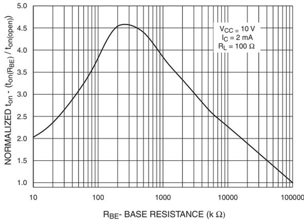
**Fig. 12 Normalized t<sub>on</sub> vs. RBE
