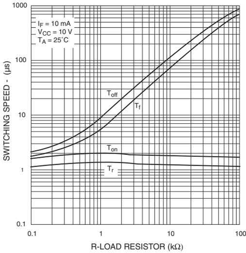
**Fig. 10 Switching Speed vs. Load Resistor
