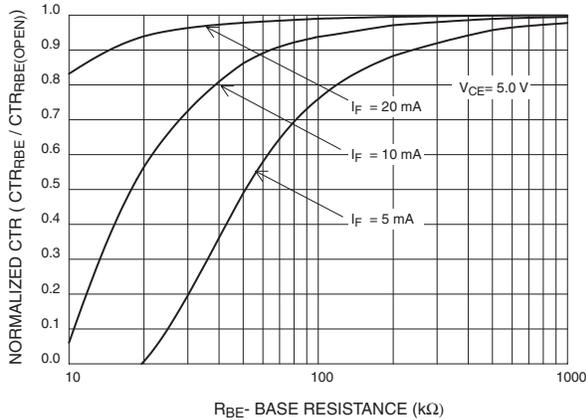
**Fig. 6 CTR vs. R<sub>BE</sub> (Unsaturated) (White Package)**
