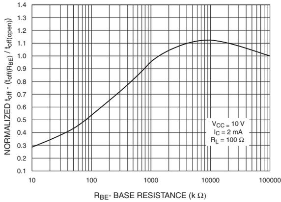
**Fig. 14 Normalized  $t_{off}$  vs.  $R_{BE}$  (White Package)**
