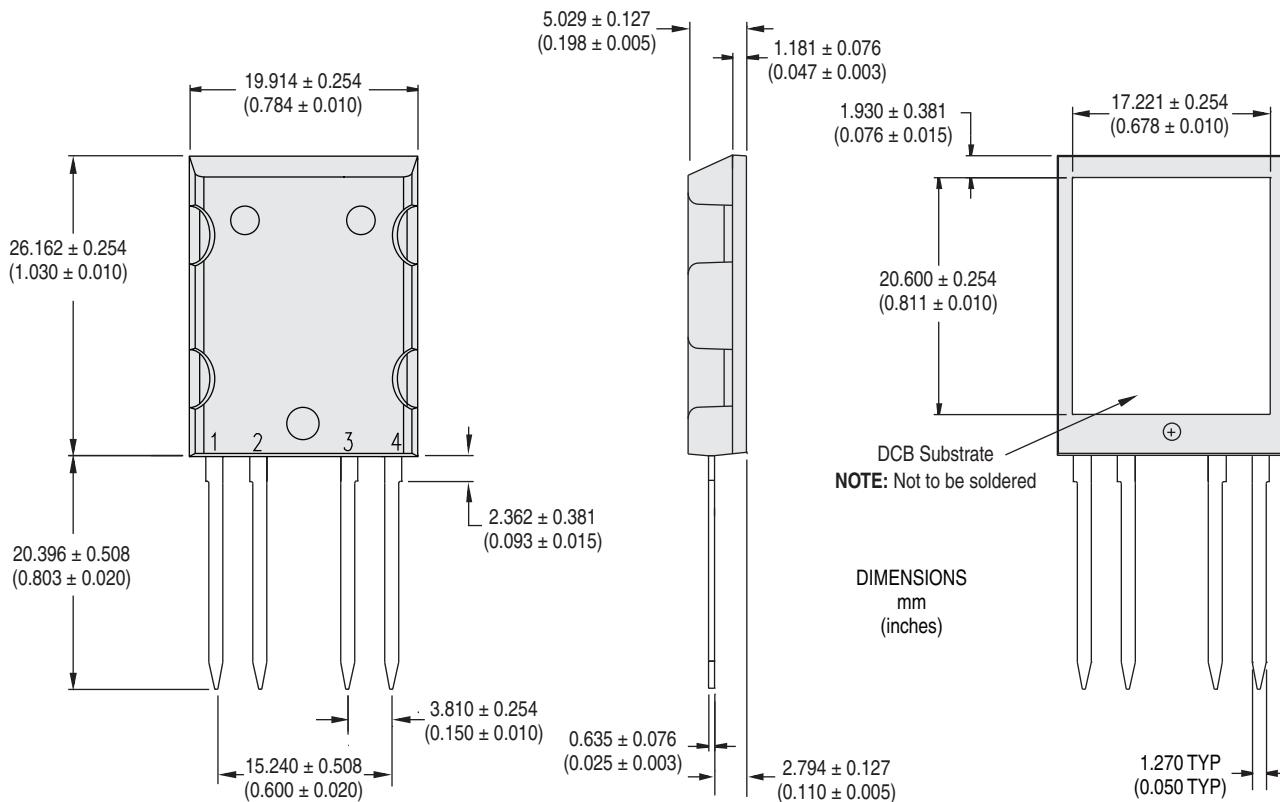
**NOTE:** Metallized external surface of DCB substrate maintains  $2500\text{V}_{\text{rms}}$  isolation to device internal structure and all external pins.
