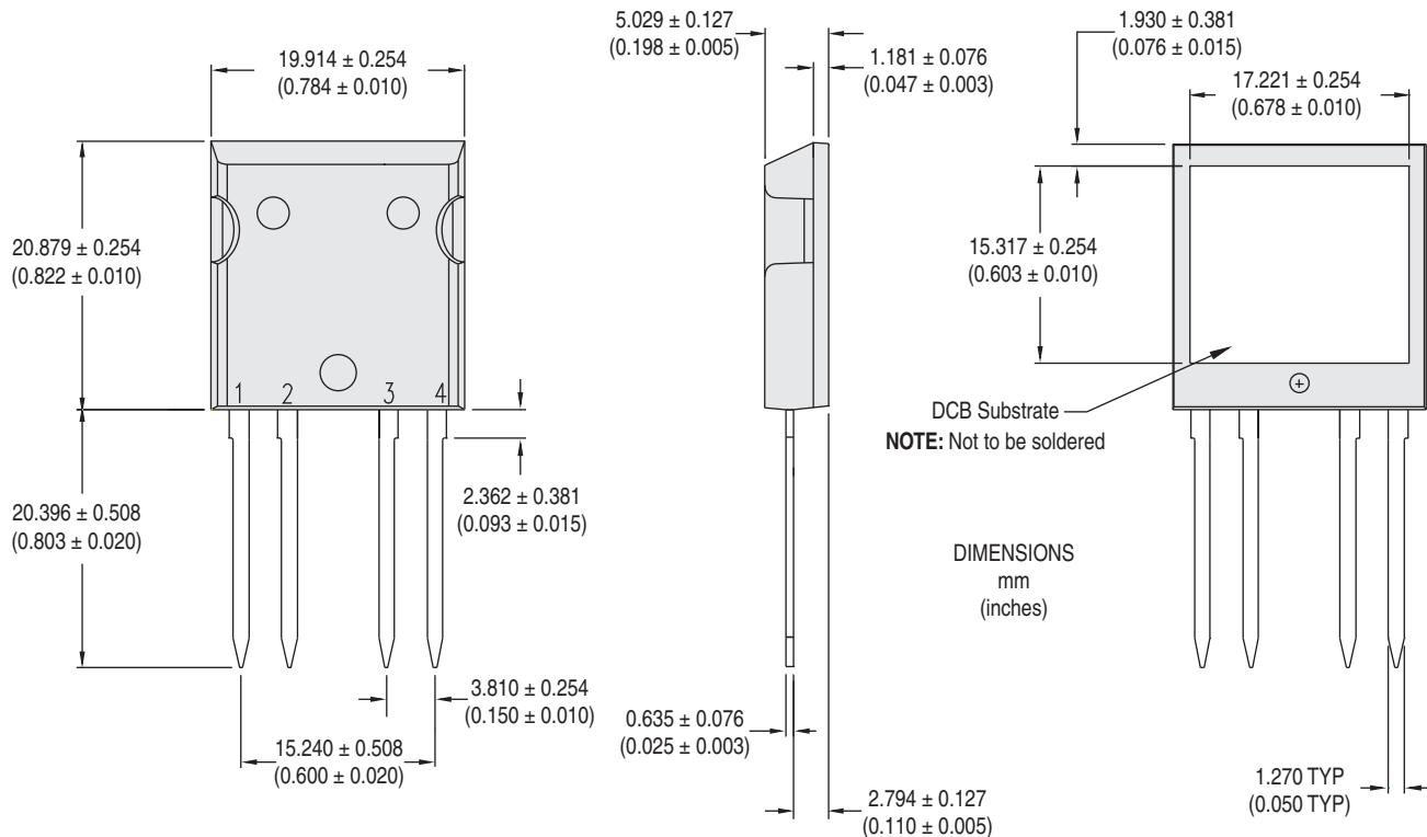
**NOTE:** Metallized external surface of DCB substrate maintains  $2500V_{rms}$  isolation to device internal structure and all external pins.
