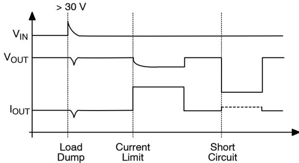
Figure 3. Typical Circuit Waveforms for Output Stage Protection
