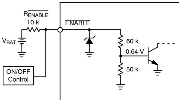
Figure 7. Using the  $\overline{\text{ENABLE}}$  pin with  $V_{\text{BAT}}$
