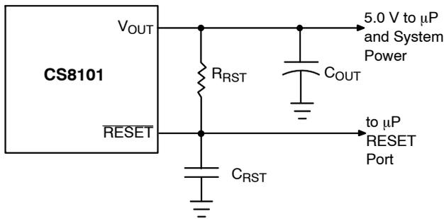
**Figure 5. RC Network for  $\overline{\text{RESET}}$  Delay**
