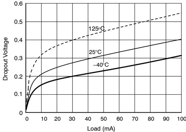
Figure 2. CS8101 Dropout Voltage vs. Load Over Temperature
