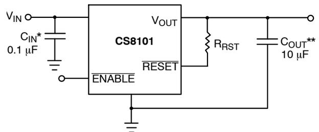
\* $C_{\text{IN}}$  required if regulator is located far from the power supply filter.
