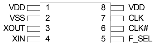
Figure 1. Pin Diagram - 8 Pin TSSOP
