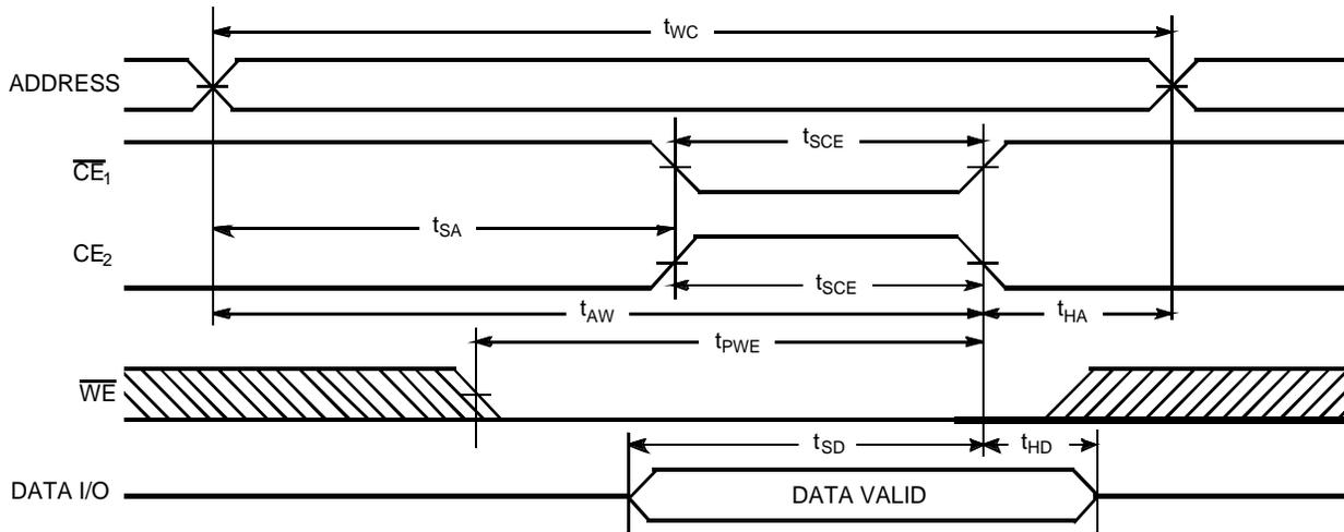
Write Cycle No. 3 ( $\overline{WE}$  Controlled,  $\overline{OE}$  LOW)<sup>[10, 16, 17]</sup>
