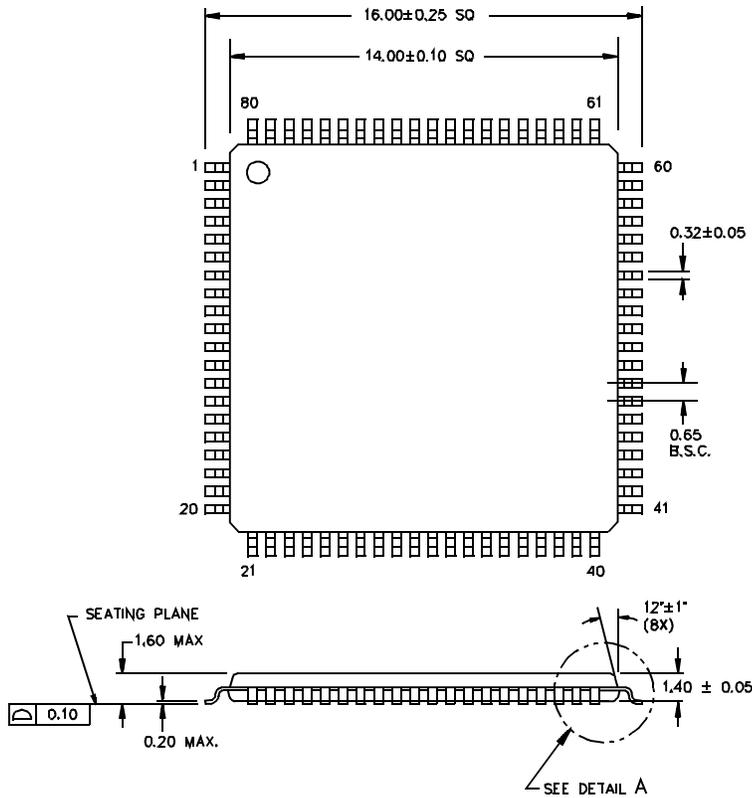
DIMENSIONS ARE IN MILLIMETERS
