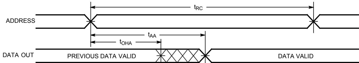
**Read Cycle No. 2 ( $\overline{OE}$  Controlled)<sup>[13, 14]</sup>**
