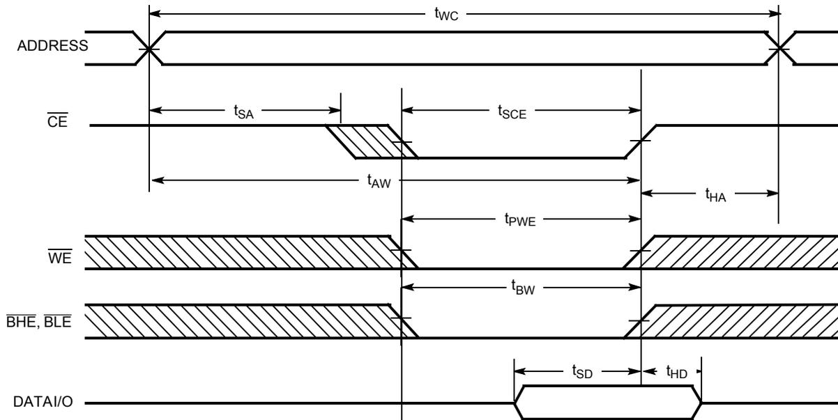
**Write Cycle No. 2 ( $\overline{\text{BLE}}$  or  $\overline{\text{BHE}}$  Controlled)**
