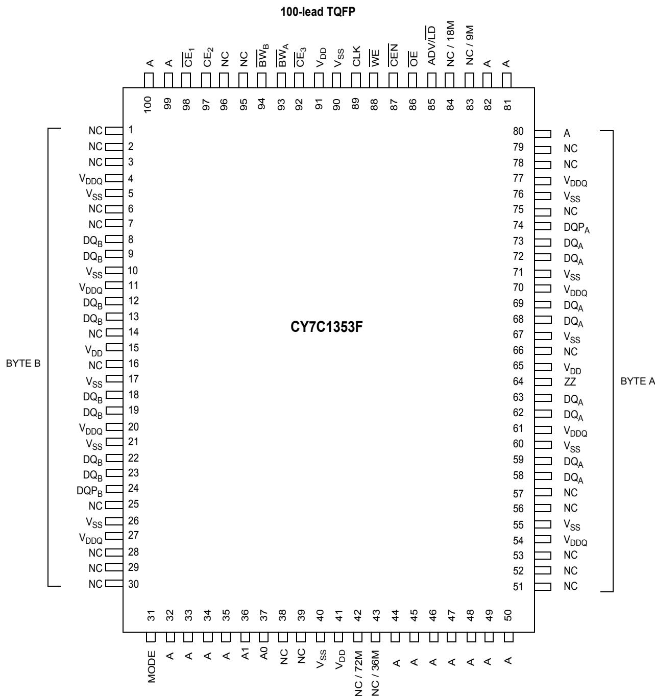
**Pin Definitions** (100-pin TQFP Package)
