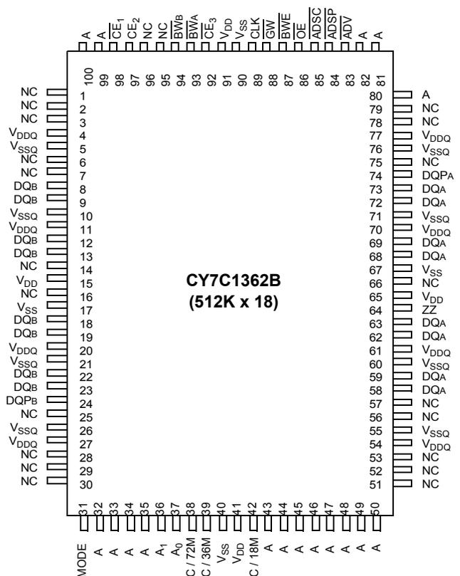
**100-pin TQFP (2 Chip Enables) (AJ Version)**
