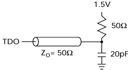
**2.5V TAP AC Output Load Equivalent**
