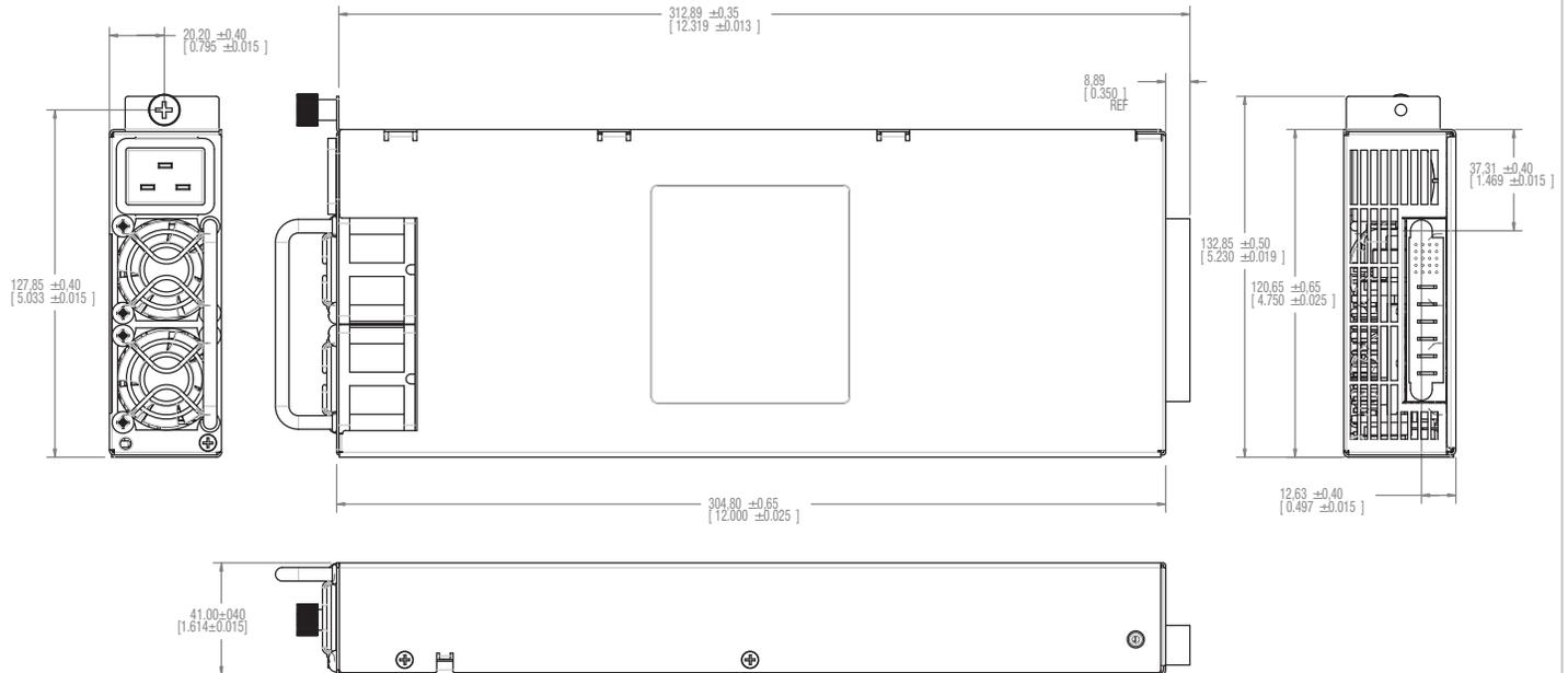
AC Input Connector: The AC input connector is standard IEC320 C20 (20A)
