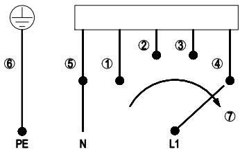
When changing speeds, switch must break the circuit
