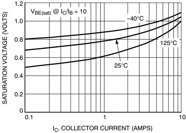
Figure 7. D44H11 ON-Voltage
