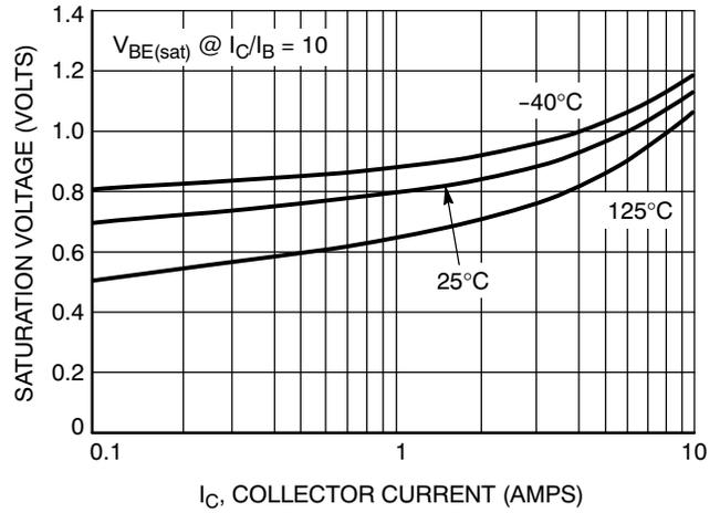
Figure 8. D45H11 ON-Voltage
