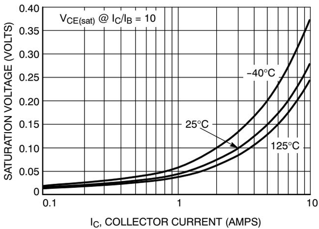
Figure 5. D44H11 ON-Voltage
