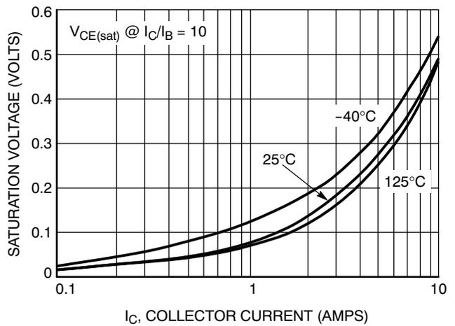
Figure 6. D45H11 ON-Voltage
