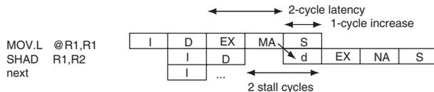
Due to the flow dependency between the load and the SHAD/SHLD shift amount, the latency of the load is increased to 3 cycles.
