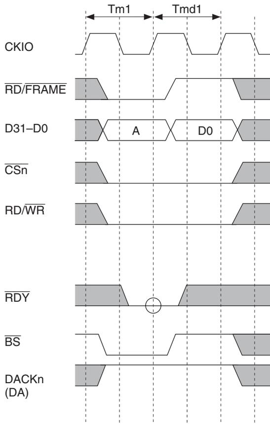
Note: For DACKn, an example is shown where CHCRn.AL (access level) = 0 for the DMAC.
