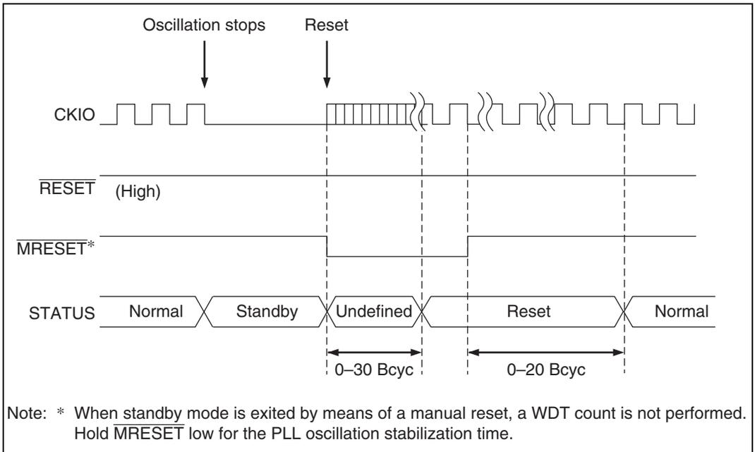
Figure 9.5 STATUS Output in Standby → Manual Reset Sequence
