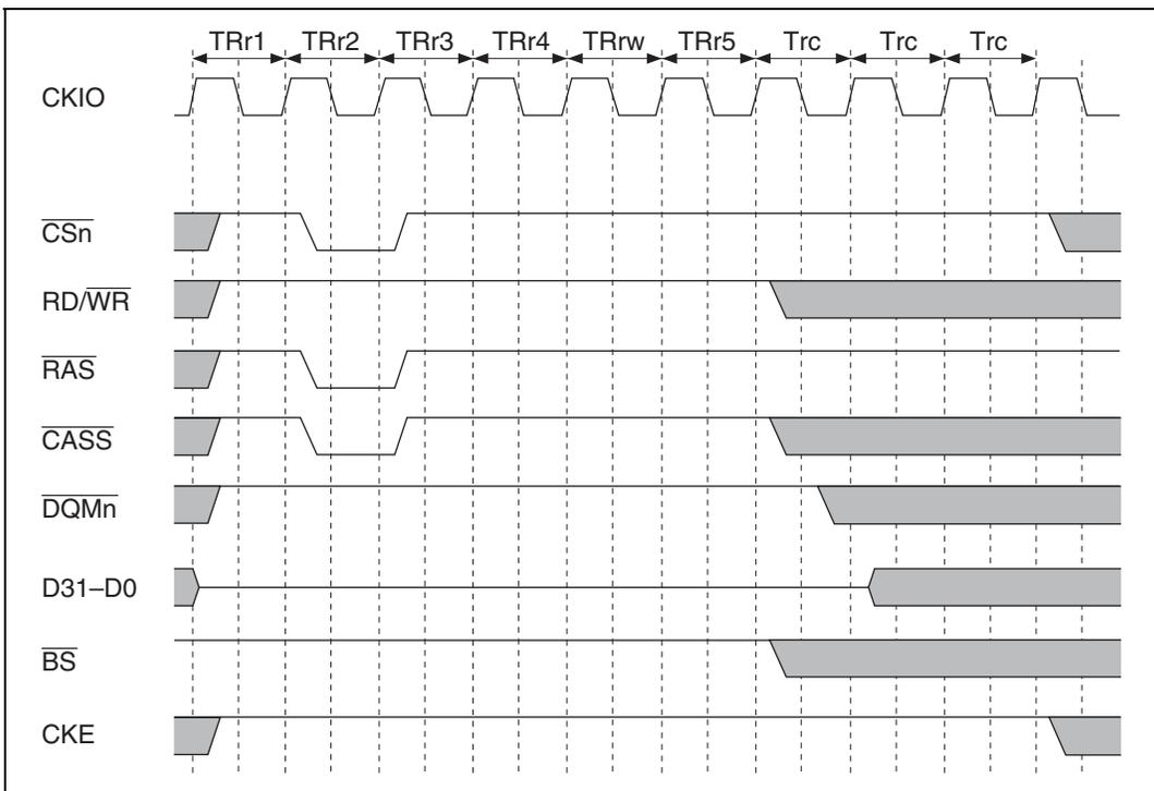
Figure 13.36 Synchronous DRAM Auto-Refresh Timing
