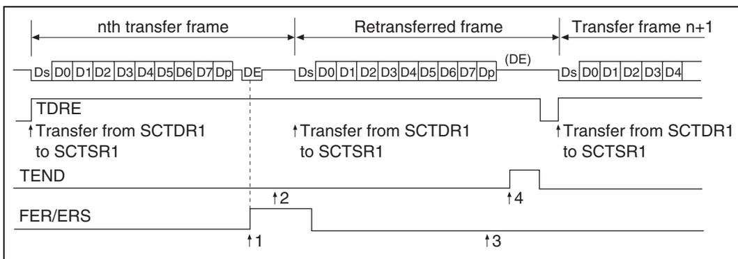
**Figure 17.12 Retransfer Operation in SCI Transmit Mode**
