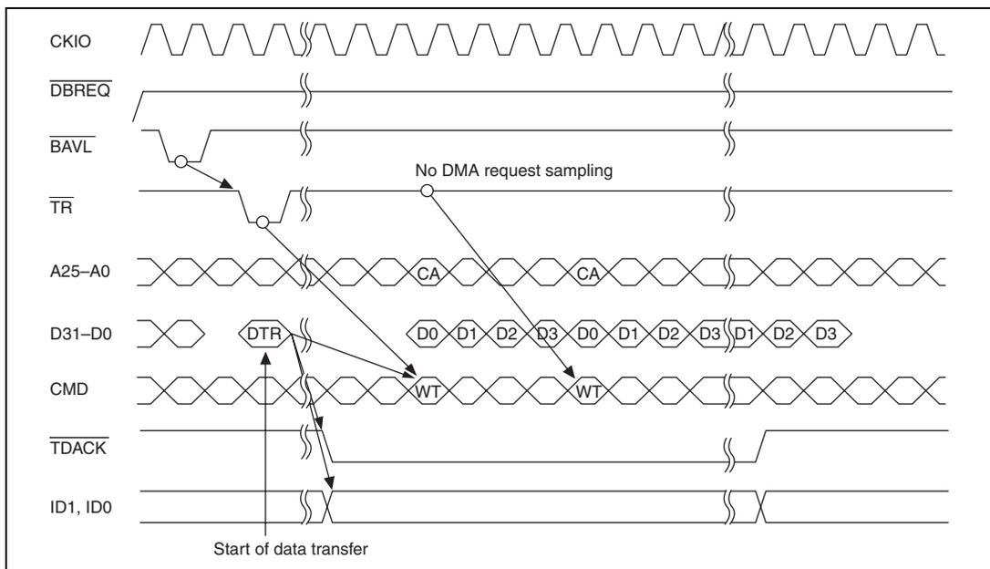
Figure 14.43 Single Address Mode/Burst Mode/Edge Detection/
