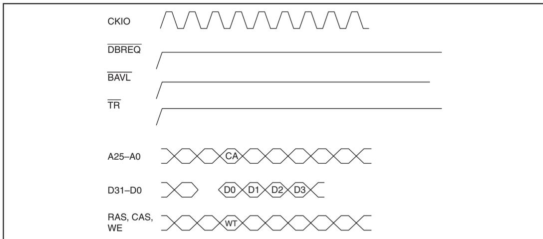
**Figure 14.40 Write to Synchronous DRAM (Row Hit)**
