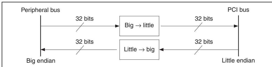
**Figure 22.17 Endian Conversion Modes for Peripheral Bus**
