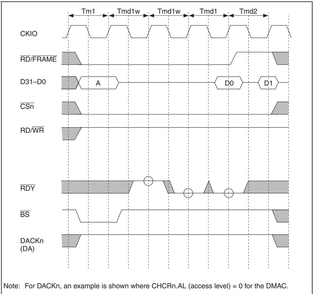
**Figure 13.61 MPX Interface Timing 10**
