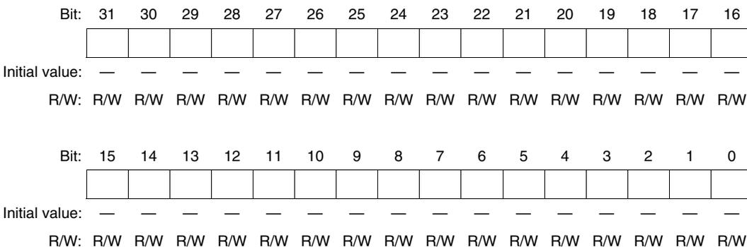
DMA destination address registers 0–7 (DAR0–DAR7) are 32-bit readable/writable registers that specify the destination address for a DMA transfer. The functions of these registers are the same as on the SH7751. For more information, see section 14.2.2, DMA Destination Address Registers 0–3 (DAR0–DAR3).
