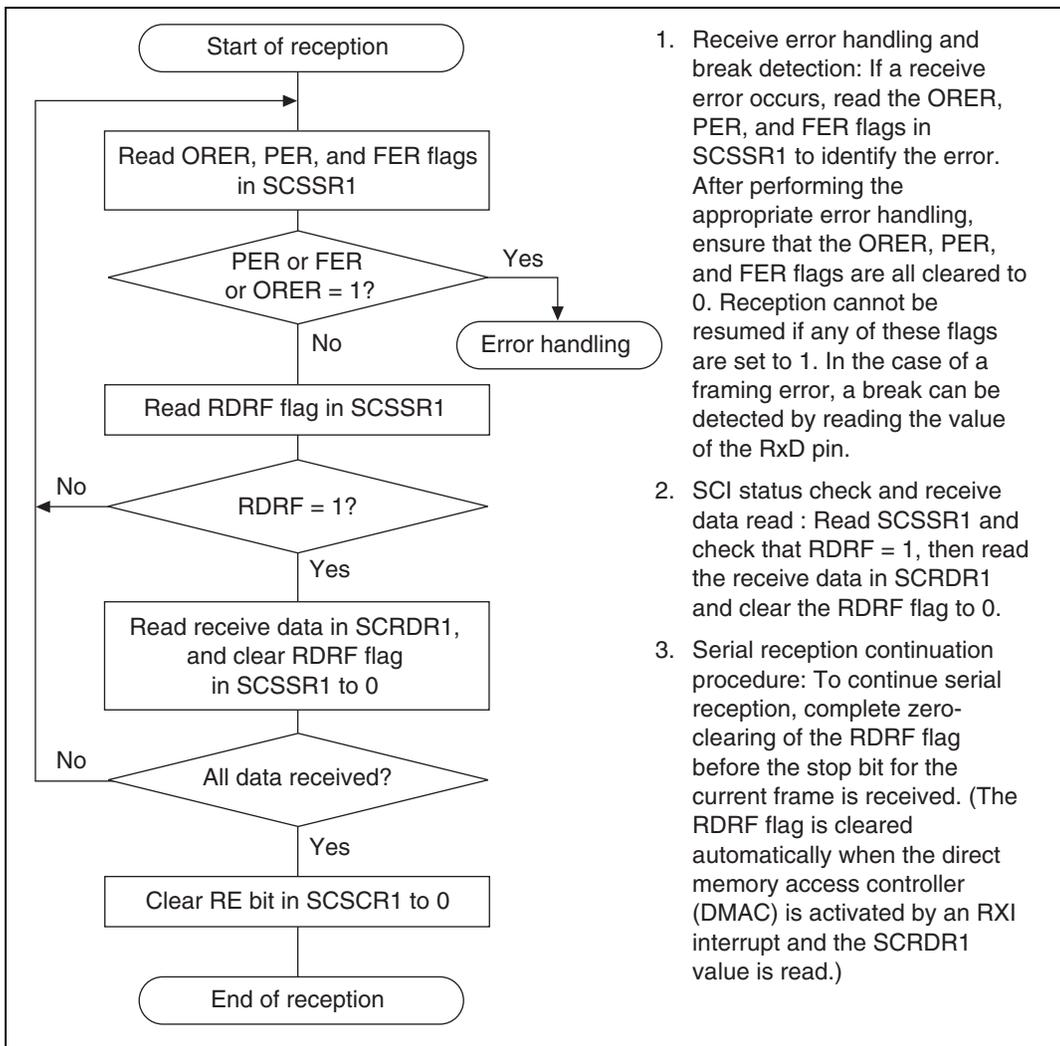
1. Receive error handling and break detection: If a receive error occurs, read the ORER, PER, and FER flags in SCSSR1 to identify the error. After performing the appropriate error handling, ensure that the ORER, PER, and FER flags are all cleared to 0. Reception cannot be resumed if any of these flags are set to 1. In the case of a framing error, a break can be detected by reading the value of the RxD pin.
