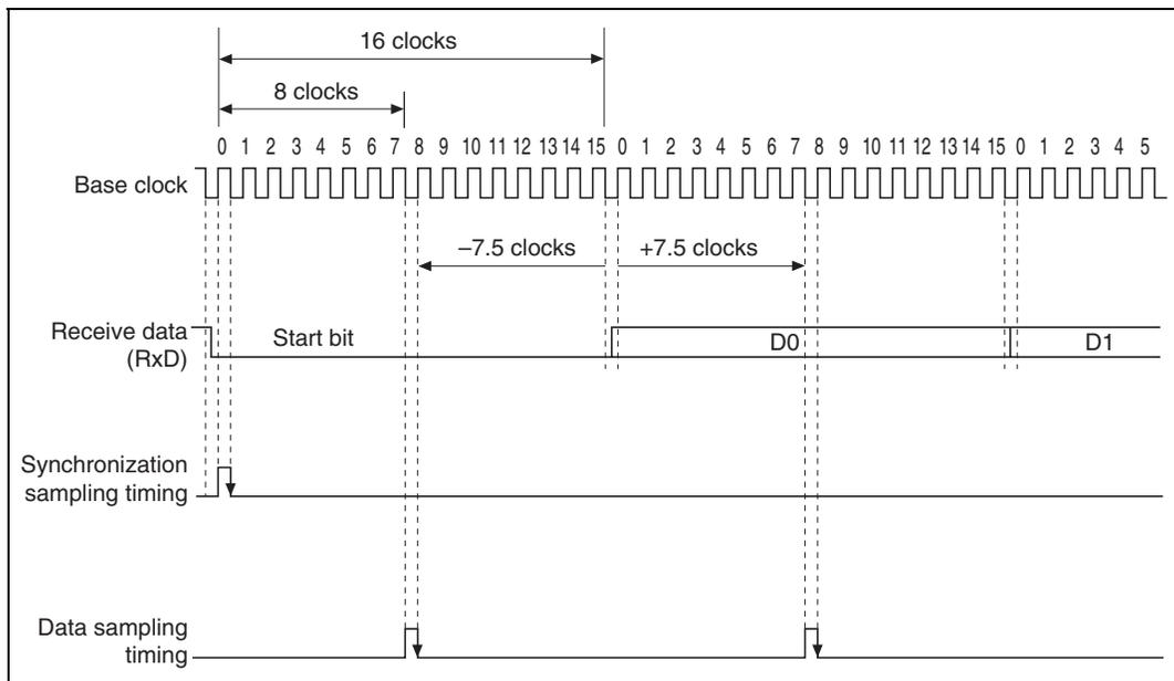
**Figure 15.25 Receive Data Sampling Timing in Asynchronous Mode**
