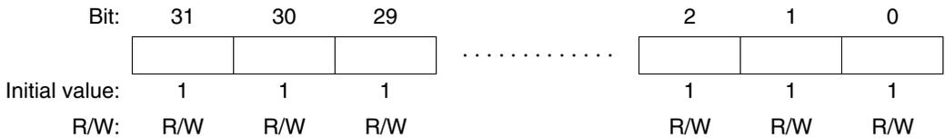
In channels 0 to 2, when the input clock is the on-chip RTC output clock (RTCCLK), TCNT counts even in module standby mode (that is, when the clock for the TMU is stopped). When the input clock is the external clock (TCLK) or internal clock (Pck), TCNT contents are retained in standby mode.
