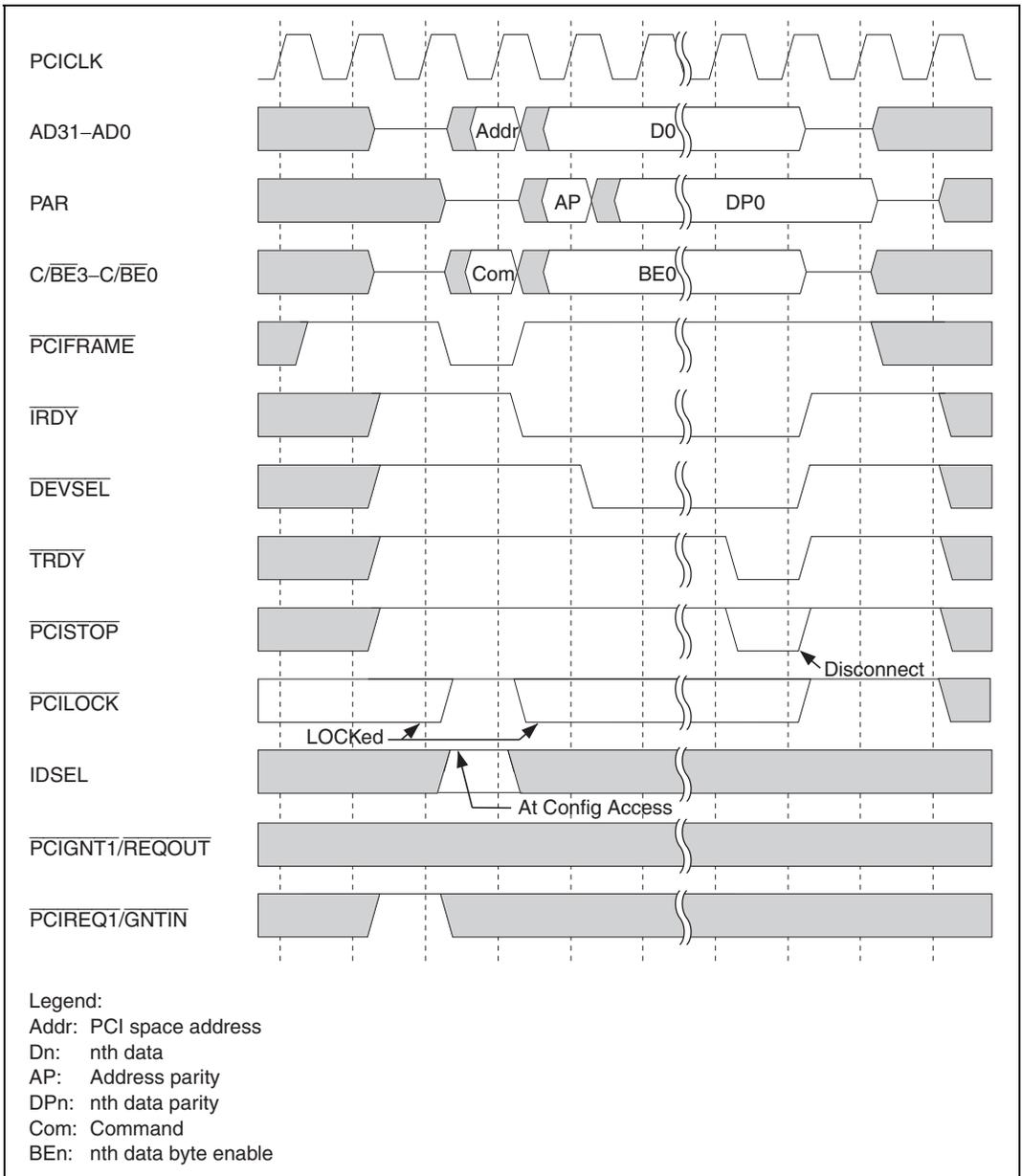
Figure 22.12 Target Write Cycle in Non-Host Mode (Single)
