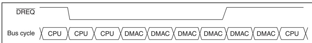
**Figure 14.10 Example of DMA Transfer in Burst Mode**
