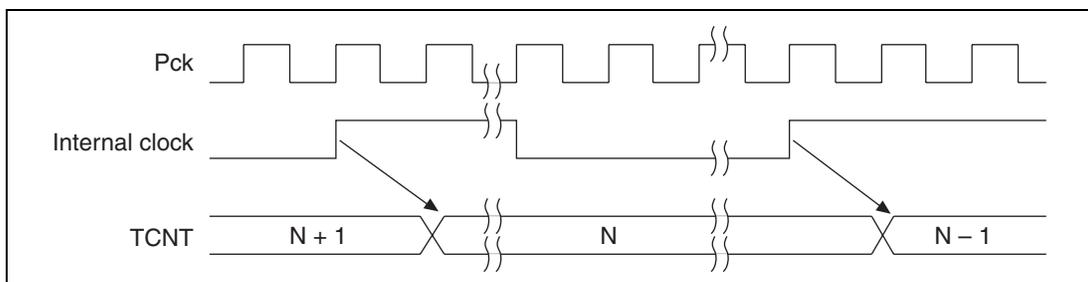
**Figure 12.4 Count Timing when Operating on Internal Clock**
