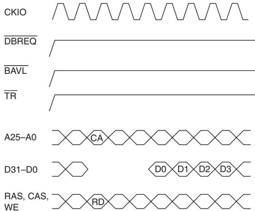
**Figure 14.37 Read from Synchronous DRAM (Row Hit)**
