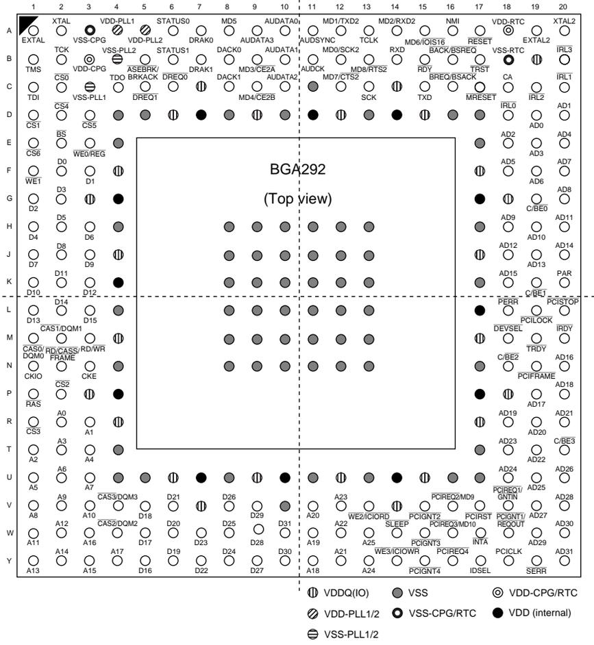
Note: Power must be supplied to the on-chip PLL power supply pins (VDD-PLL1, VDD-PLL2, VSS-PLL1, VSS-PLL2, VDD-CPG, VSS-CPG, VDD-RTC, and VSS-RTC) regardless of whether or not the PLL circuits, crystal oscillation circuit, and RTC are used.
