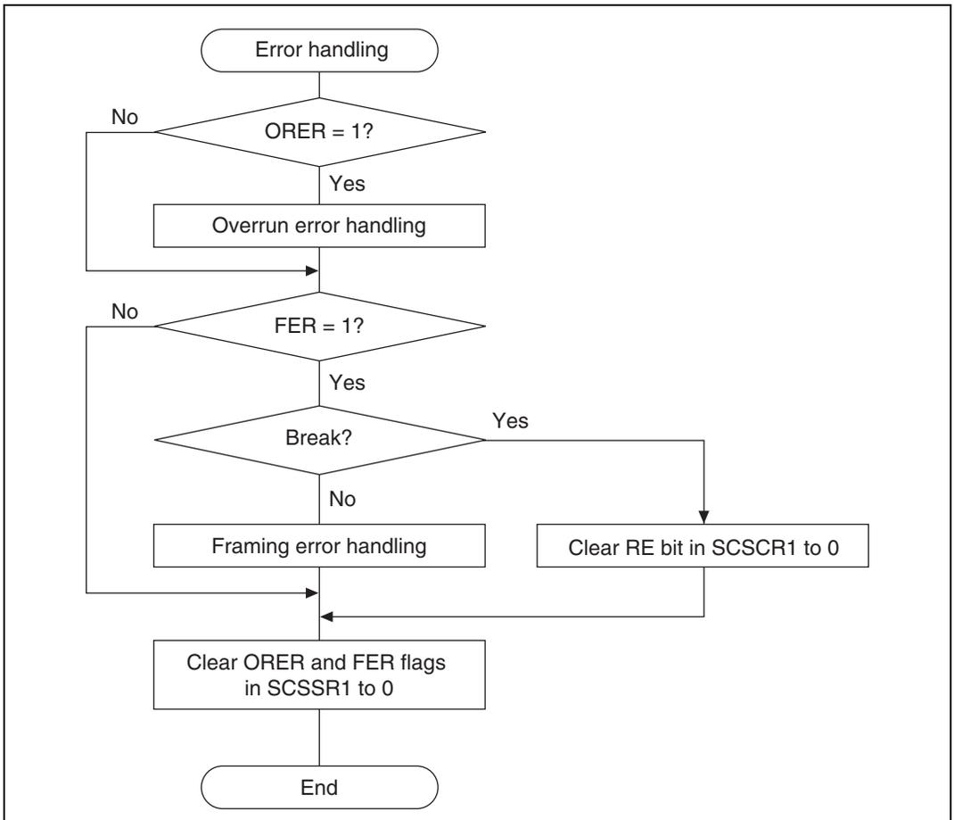
**Figure 15.16 Sample Multiprocessor Serial Reception Flowchart (2)**
