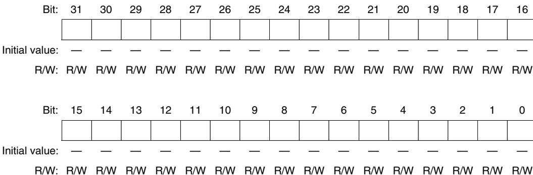
DMA source address registers 0–7 (SAR0–SAR7) are 32-bit readable/writable registers that specify the source address for a DMA transfer. The functions of these registers are the same as on the SH7751. For more information, see section 14.2.1, DMA Source Address Registers 0–3 (SAR0–SAR3).
