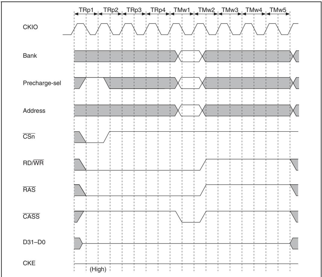
Figure 13.38 (1) Synchronous DRAM Mode Write Timing (PALL)
