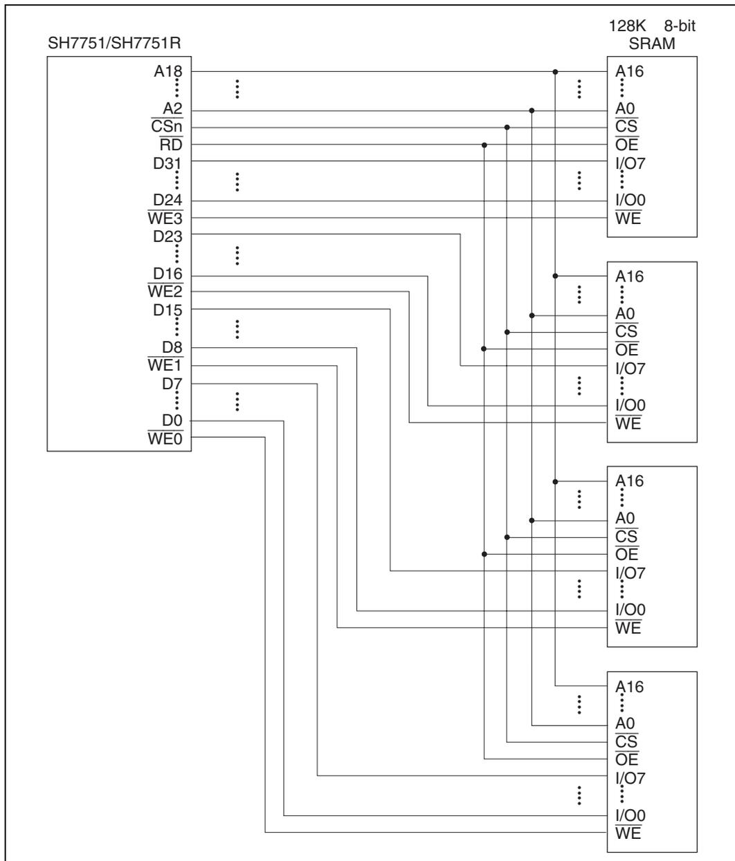
**Figure 13.7 Example of 32-Bit Data Width SRAM Connection**
