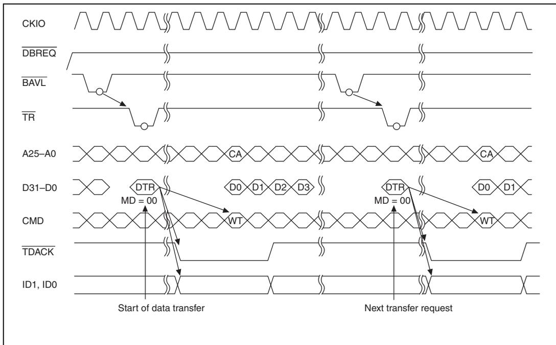
**Figure 14.33 Handshake Protocol Using Data Bus
