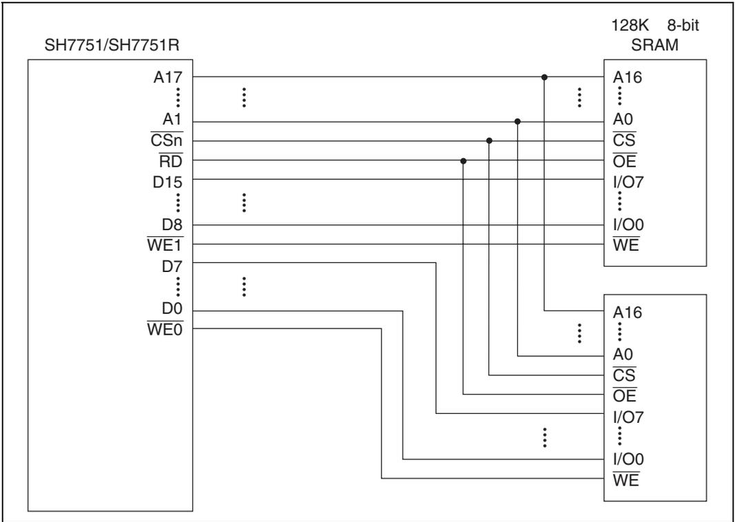
Figure 13.8 Example of 16-Bit Data Width SRAM Connection
