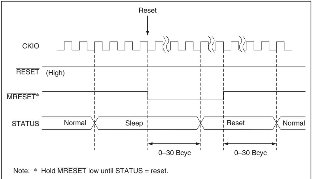
**Figure 9.8 STATUS Output in Sleep → Manual Reset Sequence**
