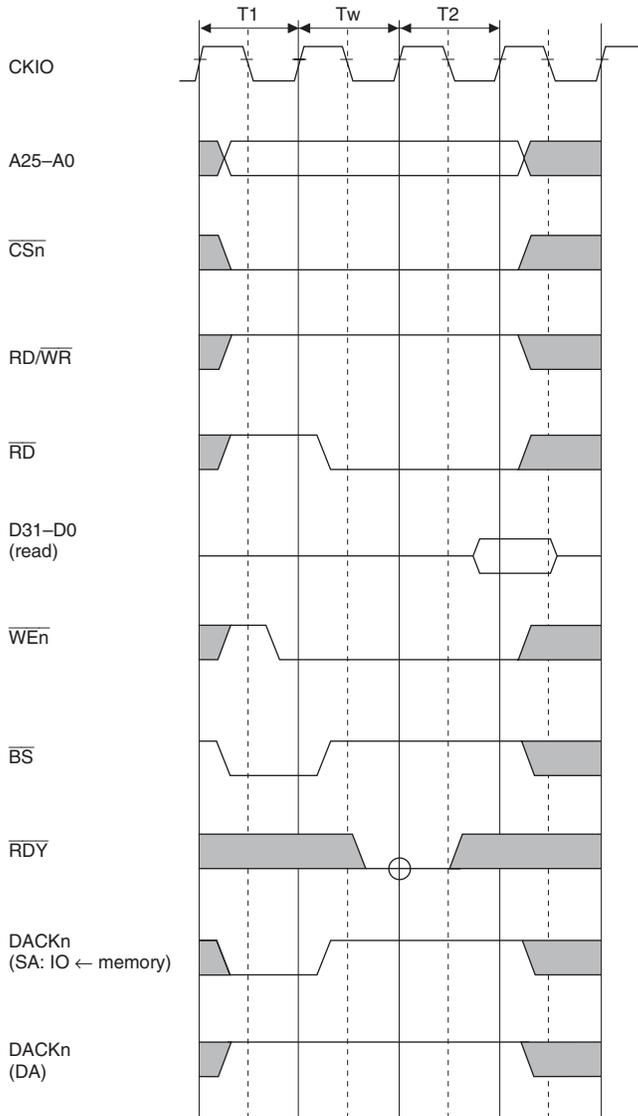
Note: For DACK<sub>n</sub>, an example is shown where CHCR<sub>n</sub>.AL (access level) = 0 for the DMAC.
