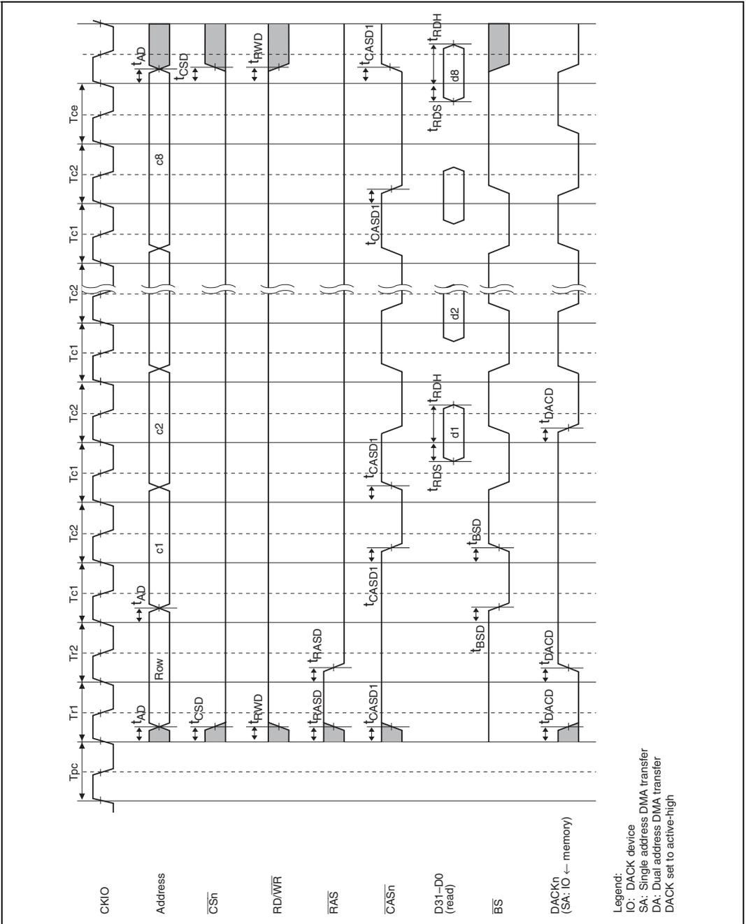
**Figure 23.40 DRAM Burst Bus Cycle: RAS Down Mode State
