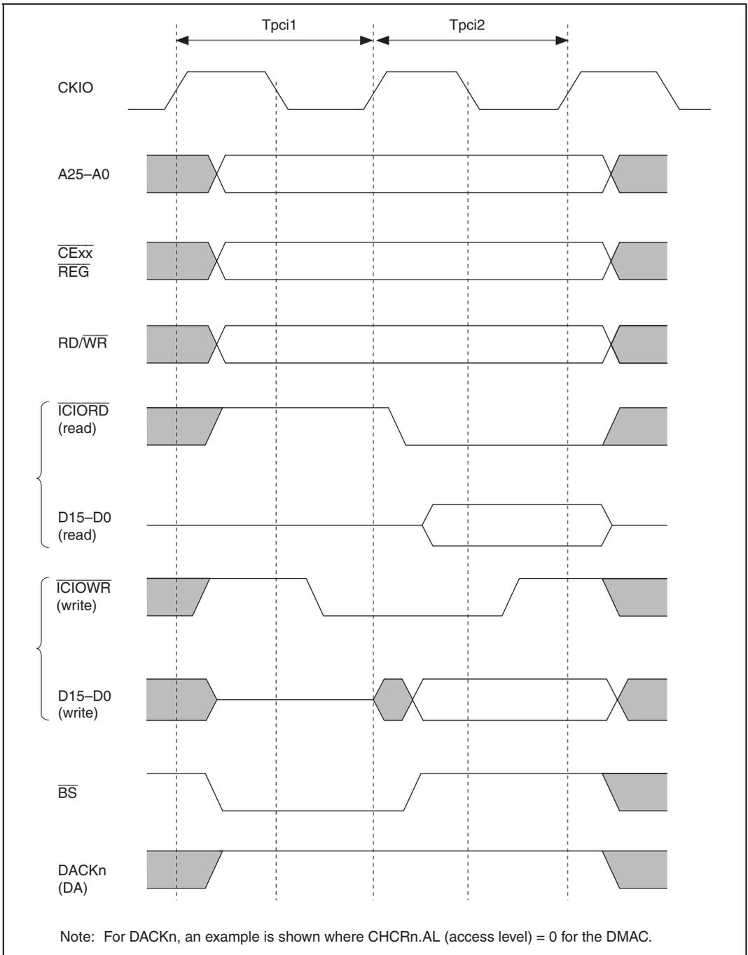
**Figure 13.48 Basic Timing for PCMCIA I/O Card Interface**
