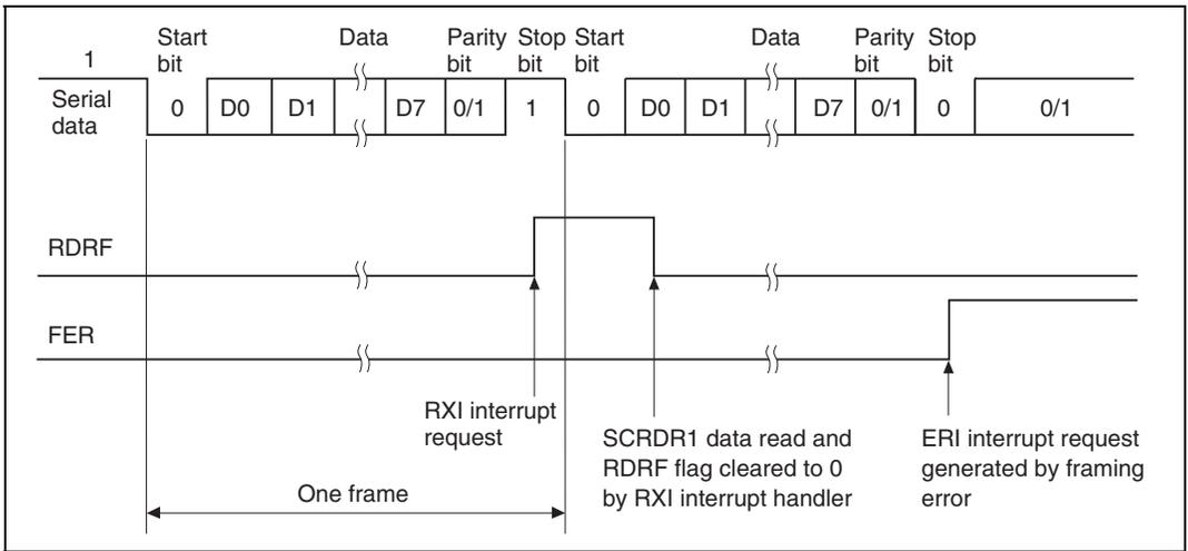
**Figure 15.11 Example of SCI Receive Operation
