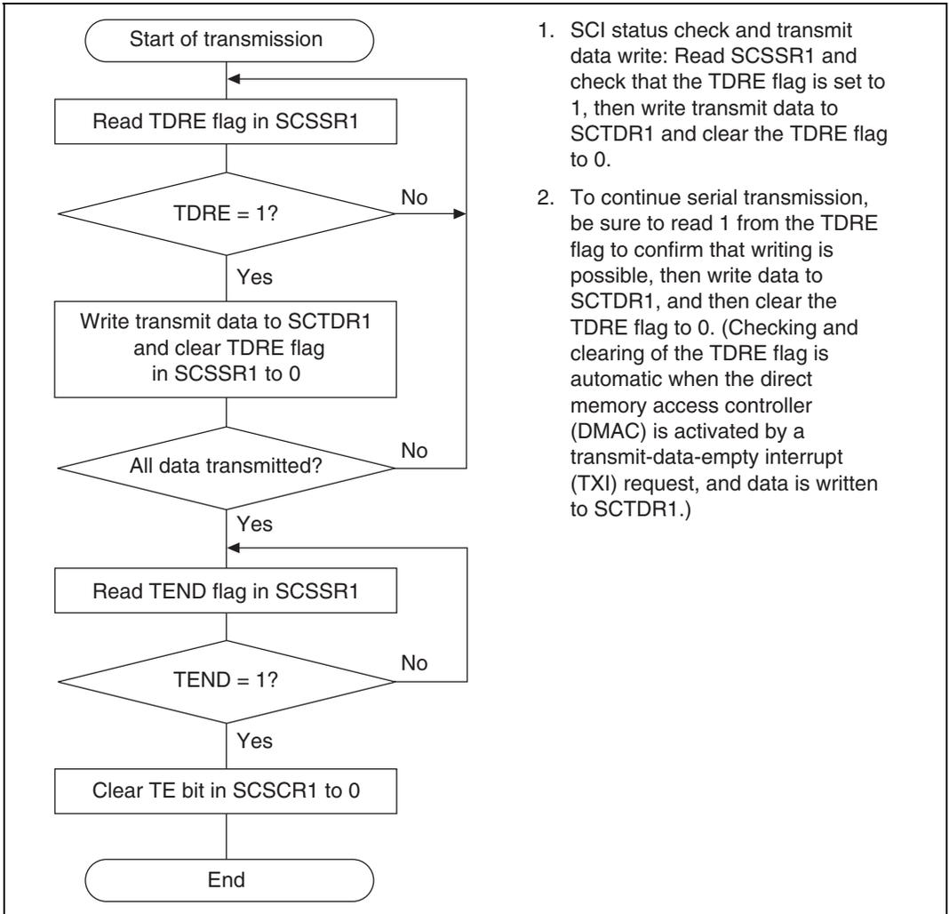
1. SCI status check and transmit data write: Read SCSSR1 and check that the TDRE flag is set to 1, then write transmit data to SCTDR1 and clear the TDRE flag to 0.
