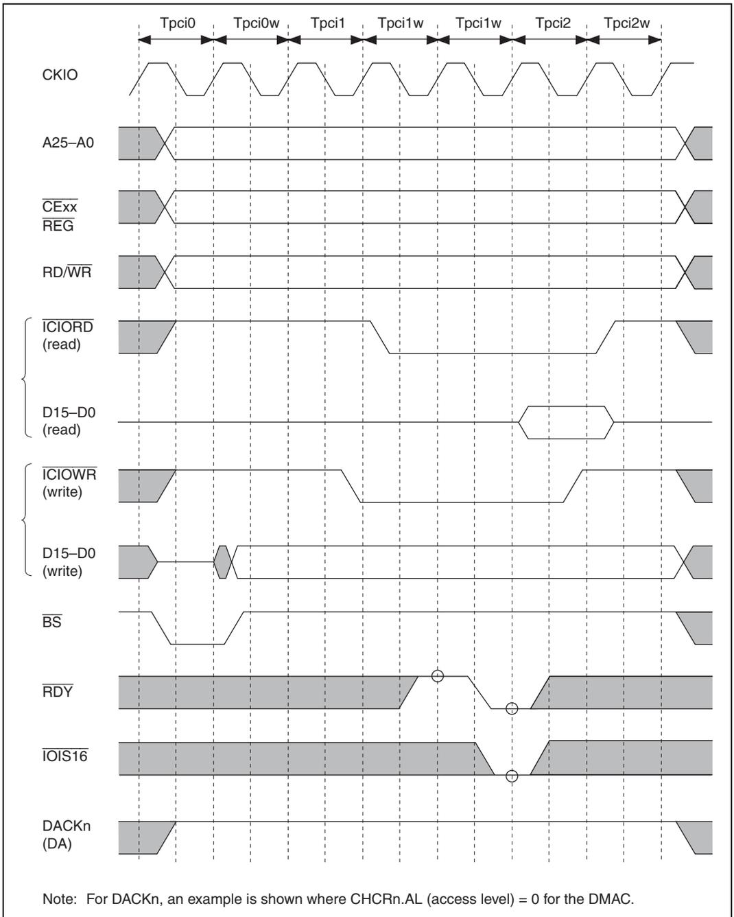
**Figure 13.49 Wait Timing for PCMCIA I/O Card Interface**
