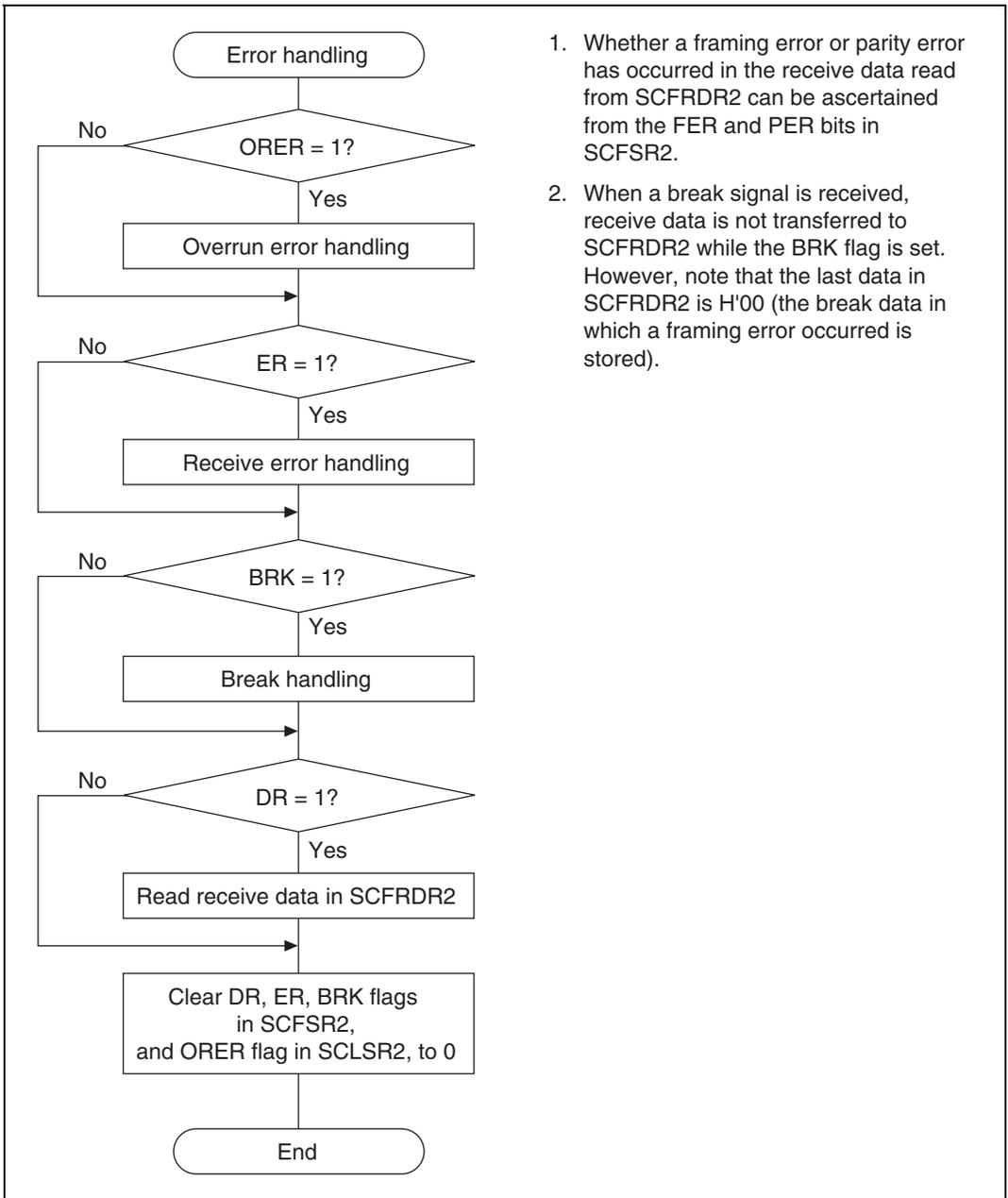
1. Whether a framing error or parity error has occurred in the receive data read from SCFRDR2 can be ascertained from the FER and PER bits in SCFSR2.
