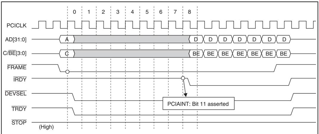
**Figure 22.26 Master Bus Timeout Interrupt Generation Example 1**
