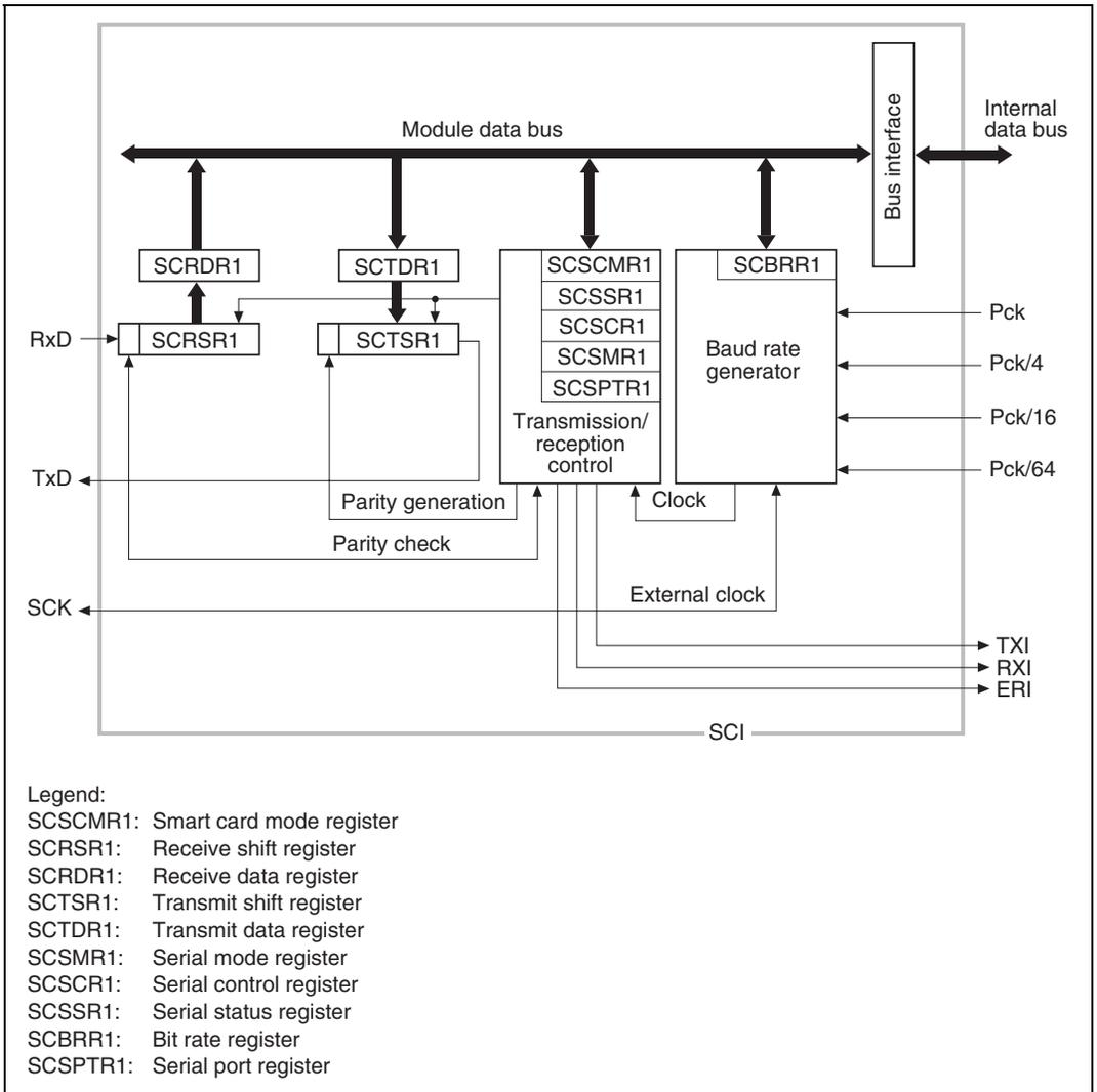
**Figure 17.1 Block Diagram of Smart Card Interface**
