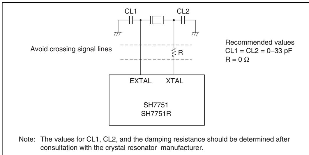
**Figure 10.4 Points for Attention when Using Crystal Resonator**
