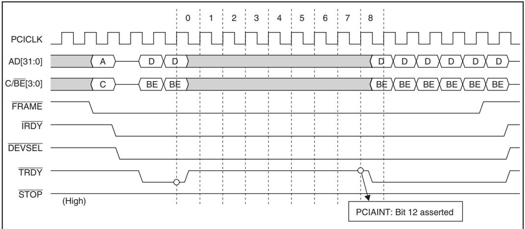
**Figure 22.25 Target Bus Timeout Interrupt Generation Example 2**
