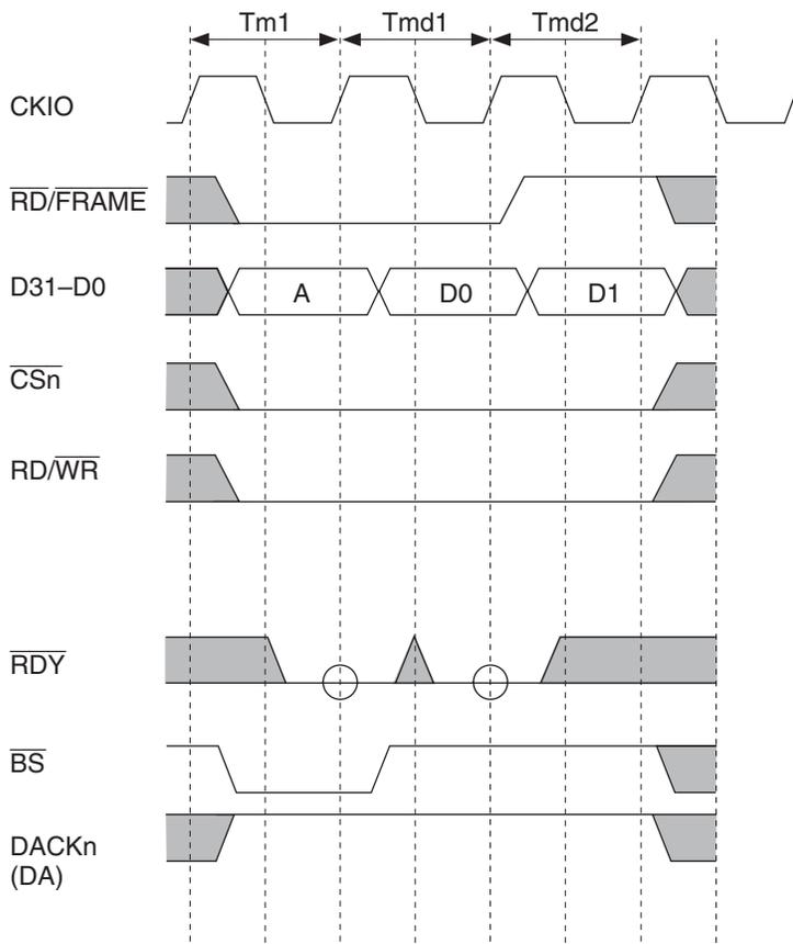
Note: For DACKn, an example is shown where CHCRn.AL (access level) = 0 for the DMAC.
