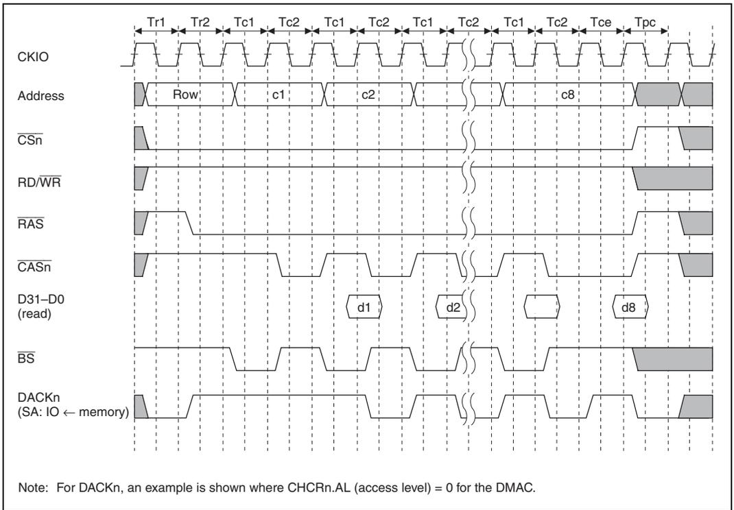
**Figure 13.18 Burst Access Timing in DRAM EDO Mode**
