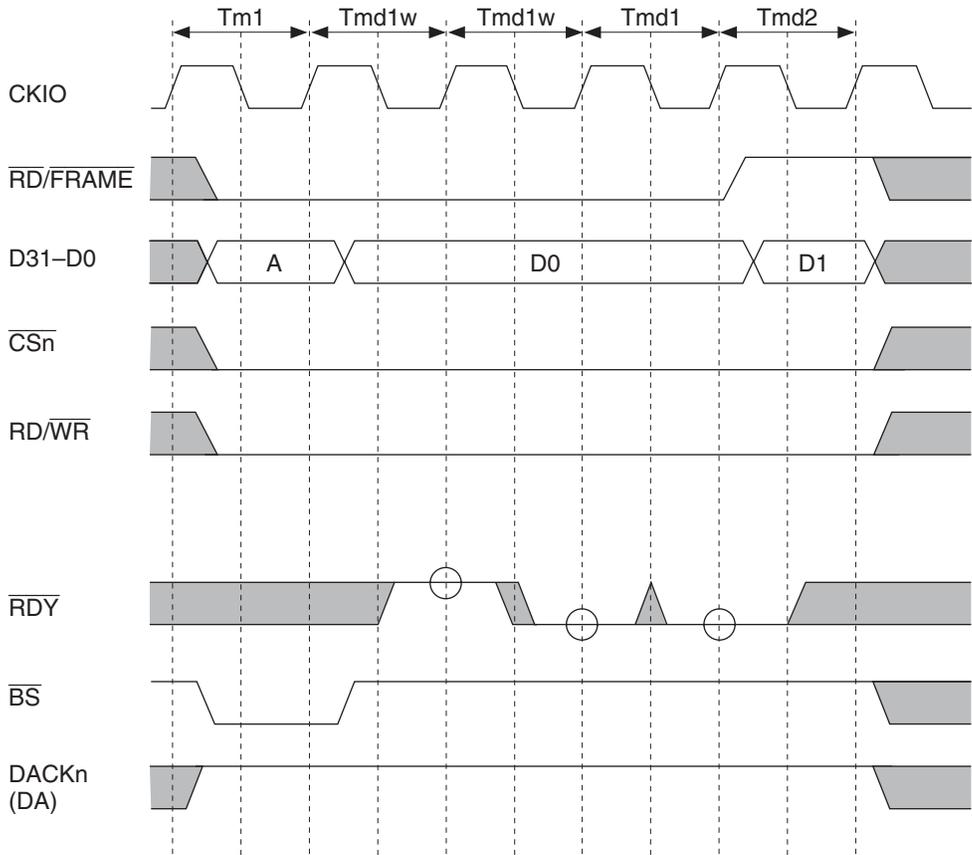
Note: For DACKn, an example is shown where CHCRn.AL (access level) = 0 for the DMAC.
