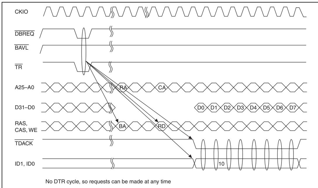
**Figure 14.48 Single Address Mode/Burst Mode/32-Byte Block Transfer/
