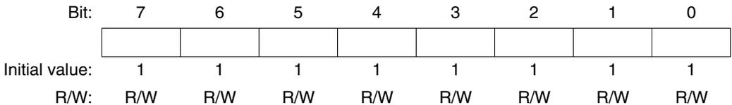
SCTDR1 is an 8-bit register that stores data for serial transmission.
