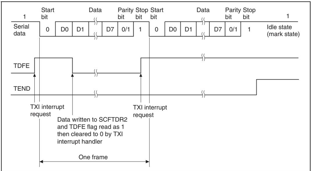
**Figure 16.9 Example of Transmit Operation
