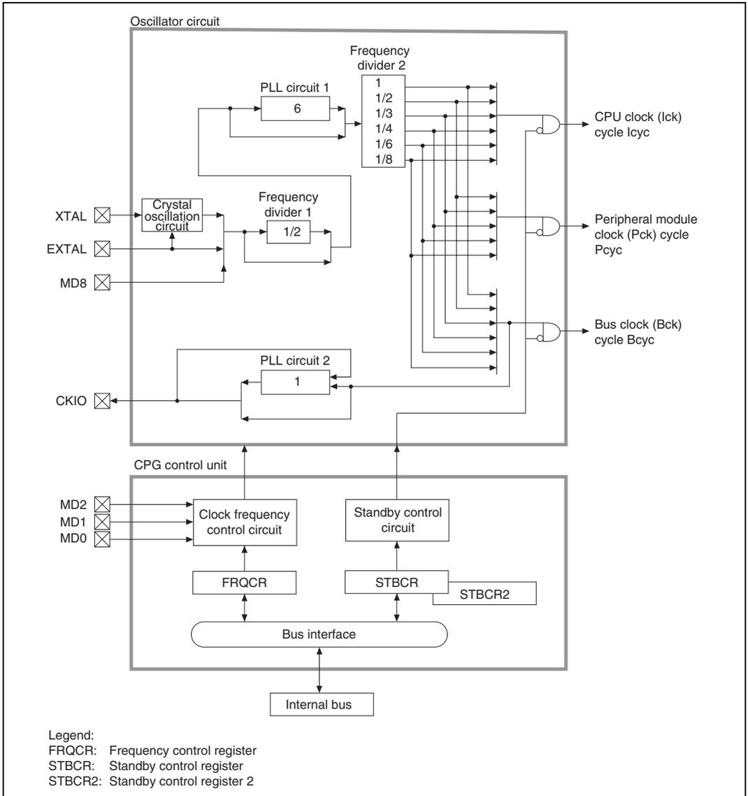
**Figure 10.1 (1) Block Diagram of CPG (SH7751)**
