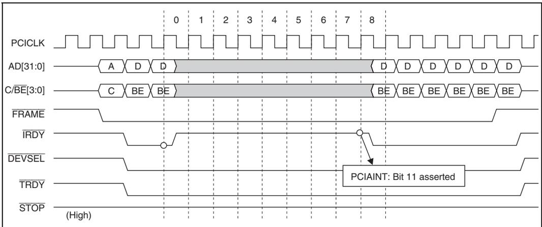
**Figure 22.27 Master Bus Timeout Interrupt Generation Example 2**
