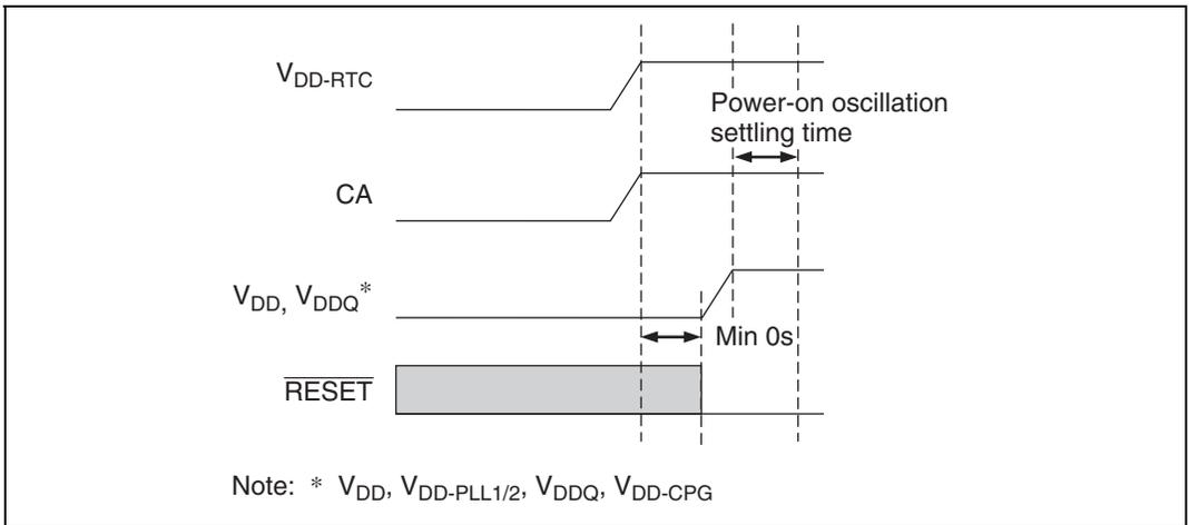
**Figure 9.15 Timing When VDD-RTC Power Is Off → On**
