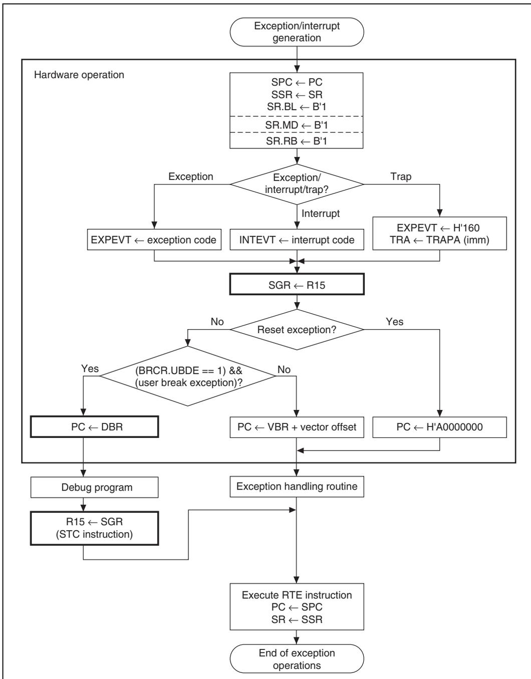
**Figure 20.2 User Break Debug Support Function Flowchart**
