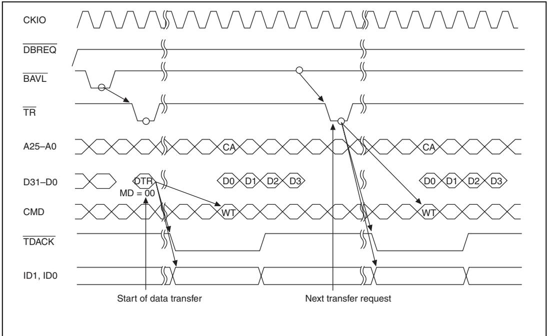
**Figure 14.34 Handshake Protocol without Use of Data Bus
