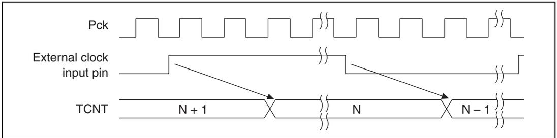
**Figure 12.5 Count Timing when Operating on External Clock**
