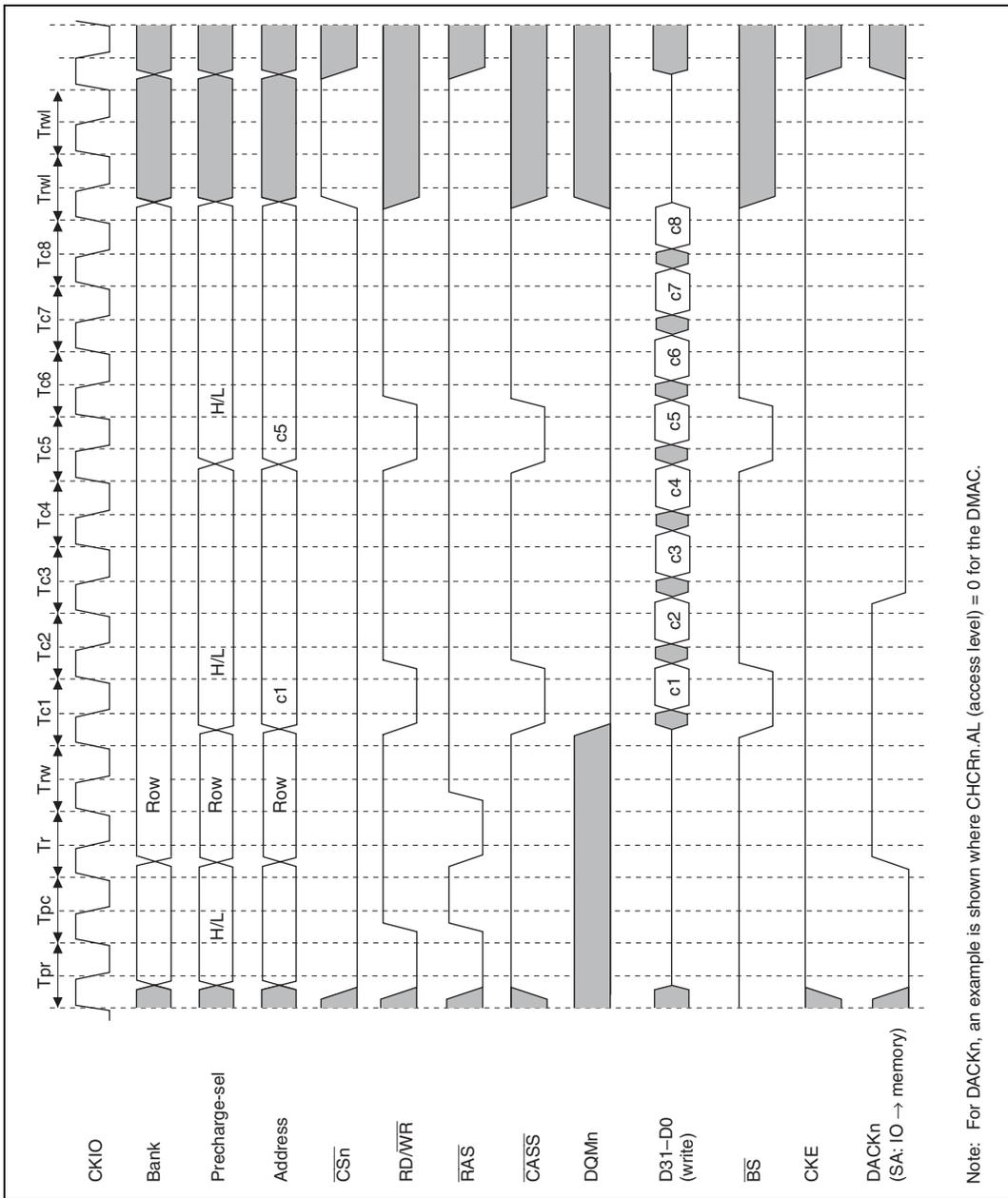
Figure 13.33 Burst Write Timing (Different Row Addresses)
