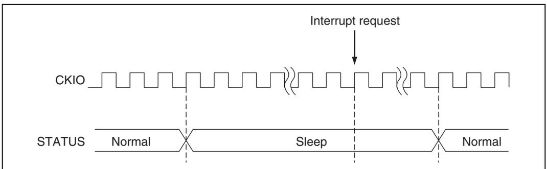
Figure 9.6 STATUS Output in Sleep → Interrupt Sequence
