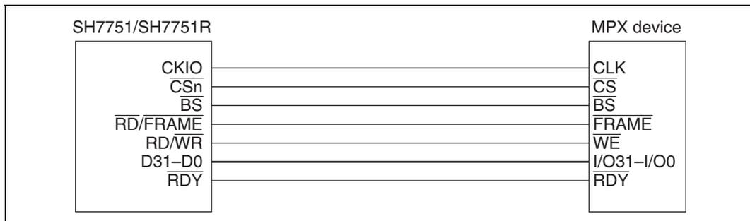
**Figure 13.51 Example of 32-Bit Data Width MPX Connection**
