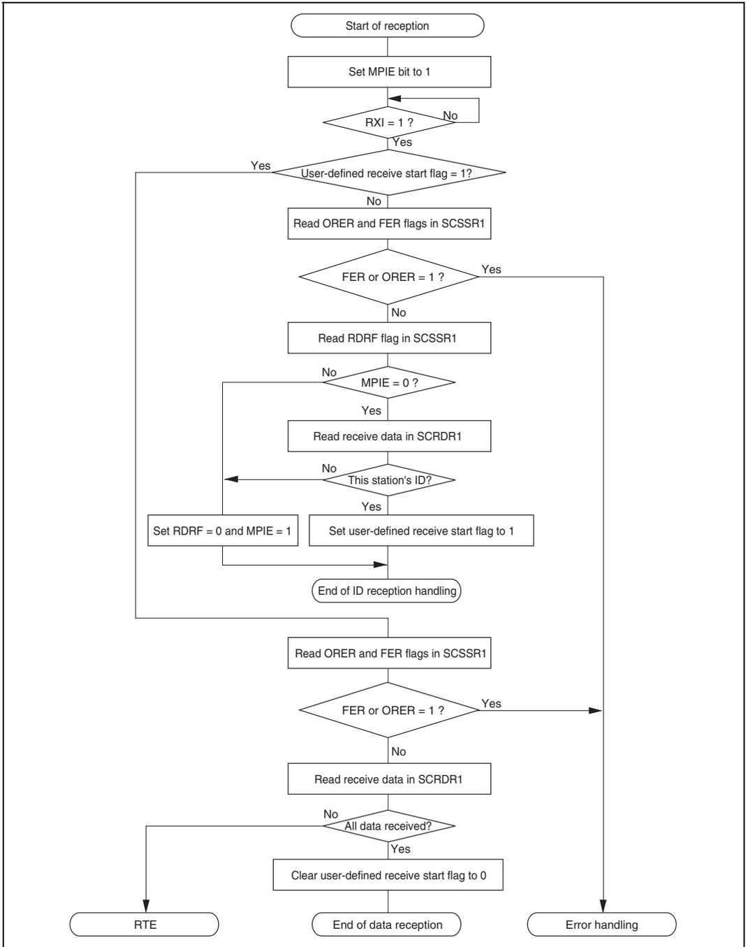
Figure 15.16 Sample Multiprocessor Serial Reception Flowchart (1)
