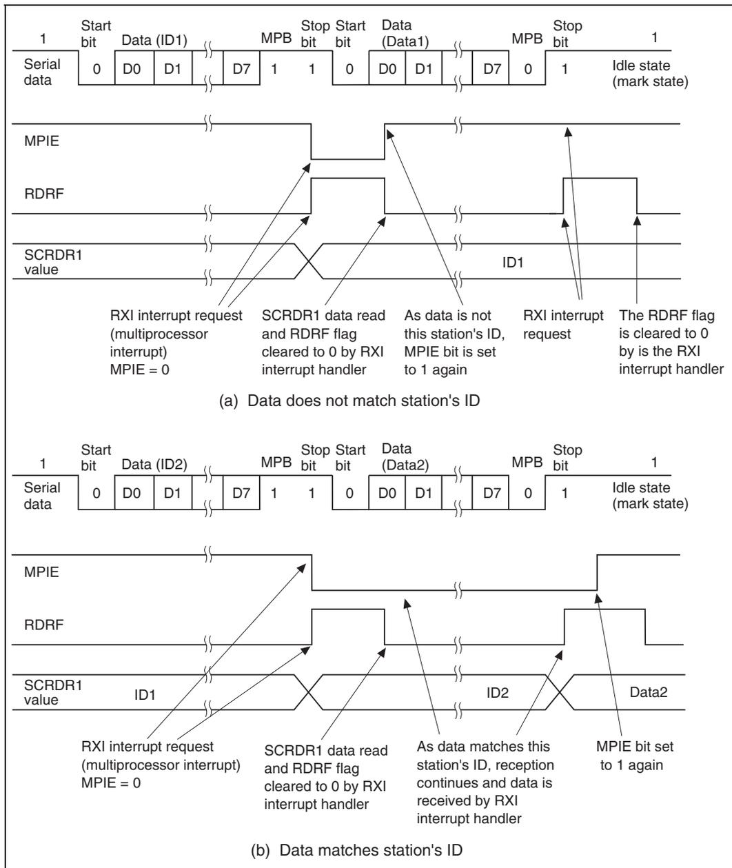
**Figure 15.17 Example of SCI Receive Operation
