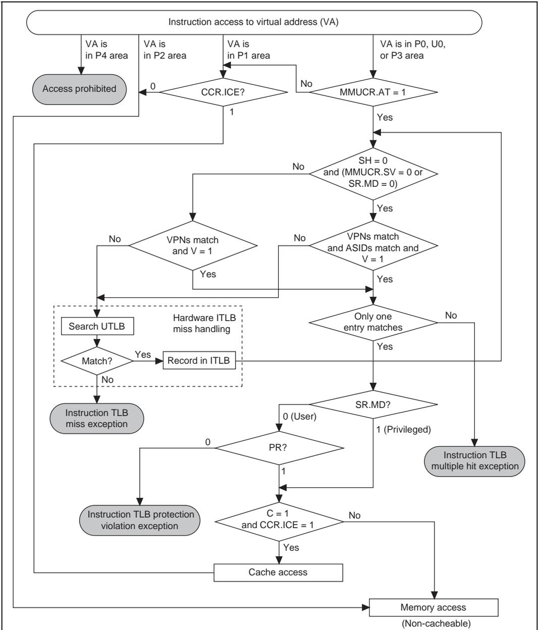
Figure 3.11 Flowchart of Memory Access Using ITLB
