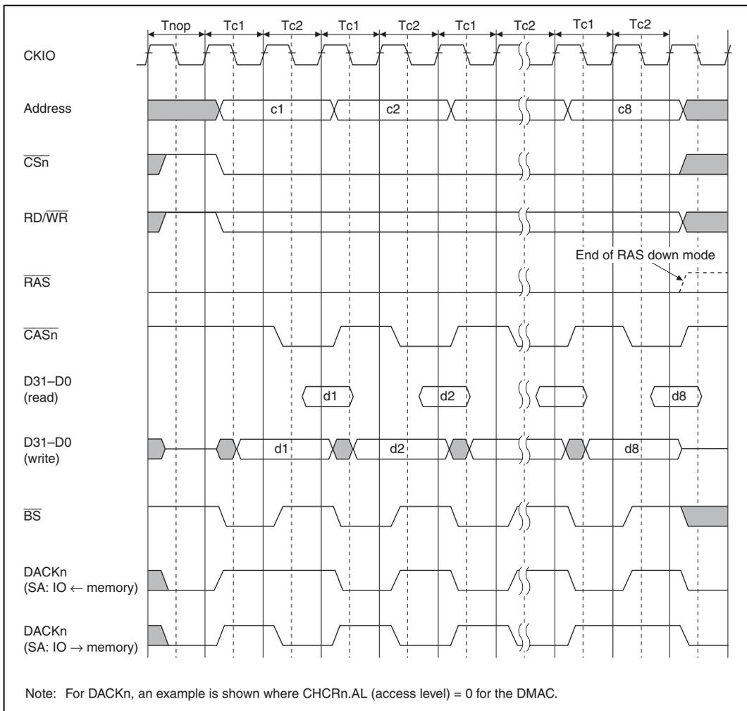
**Figure 13.19 (2) DRAM Burst Bus Cycle, RAS Down Mode Continuation
