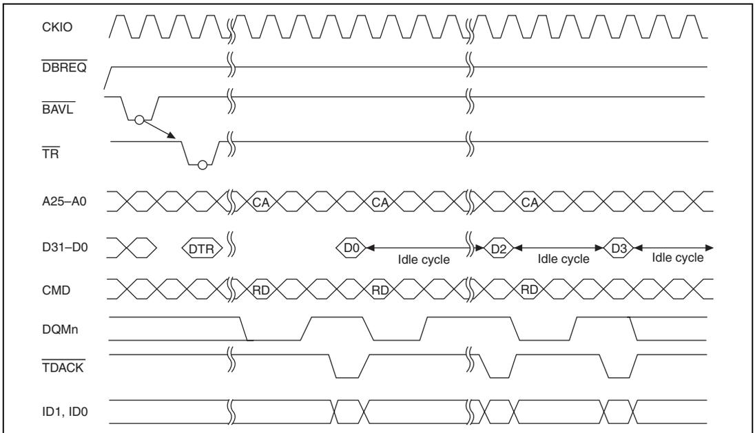
**Figure 14.45 Single Address Mode/Burst Mode/Edge Detection/Byte, Word, Longword,
