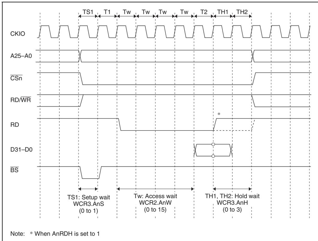
**Figure 13.12 SRAM Interface Read Strobe Negate Timing**
