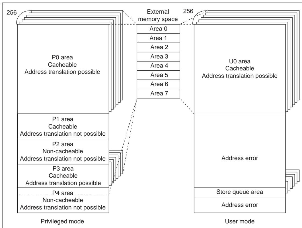
**Figure 3.6 Virtual Address Space (MMUCR.AT = 1)**
