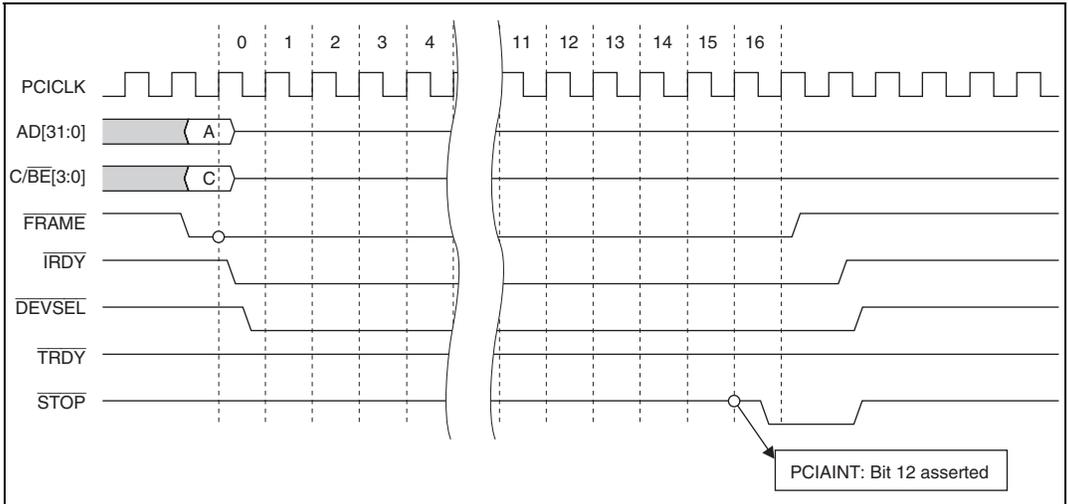
**Figure 22.24 Target Bus Timeout Interrupt Generation Example 1**
