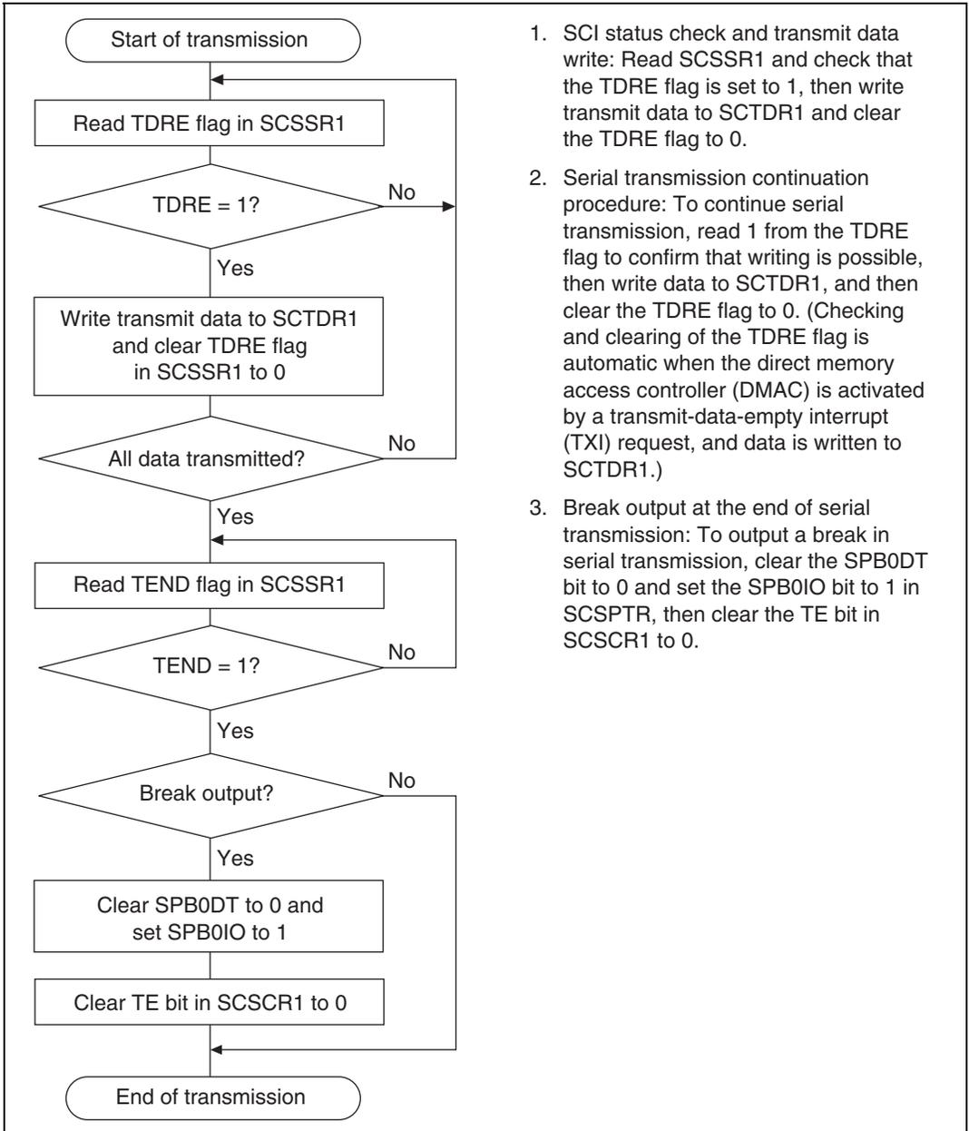
1. SCI status check and transmit data write: Read SCSSR1 and check that the TDRE flag is set to 1, then write transmit data to SCTDR1 and clear the TDRE flag to 0.
