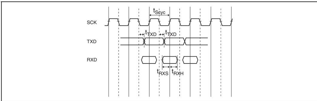
**Figure 23.62 SCI I/O Synchronous Mode Clock Timing**
