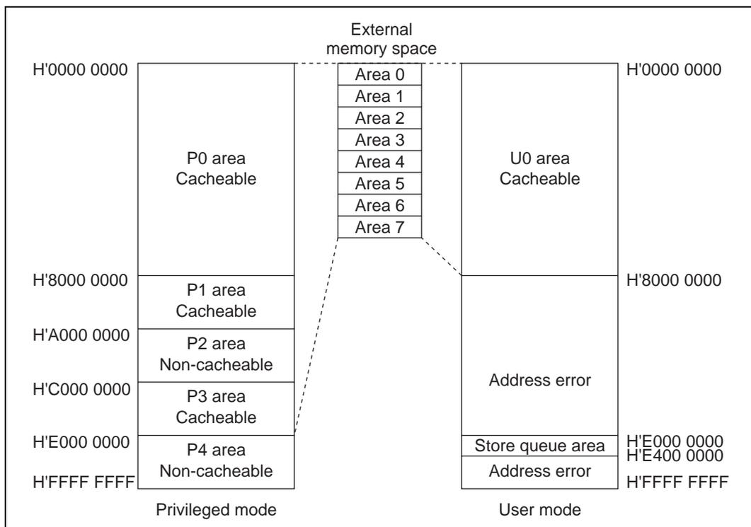
**Figure 3.3 Physical Address Space (MMUCR.AT = 0)**
