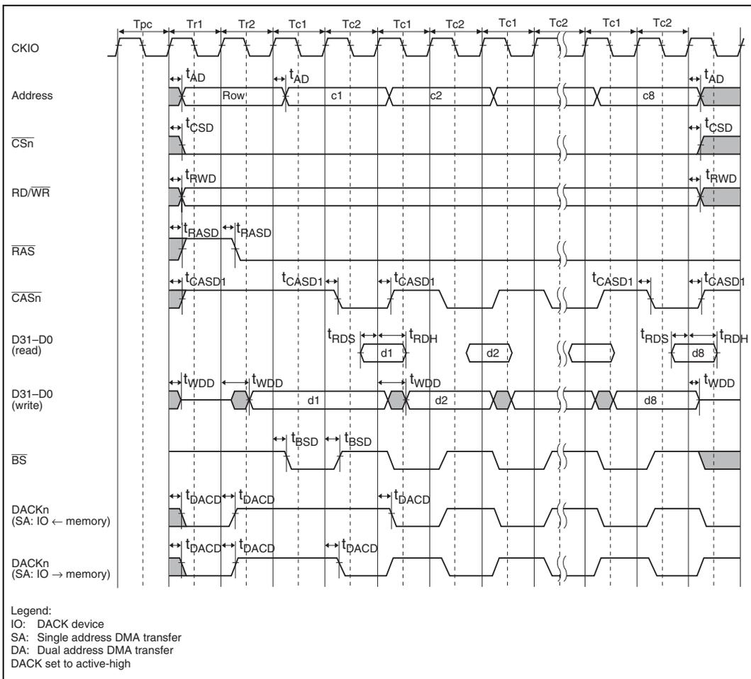
**Figure 23.45 DRAM Burst Bus Cycle: RAS Down Mode State
