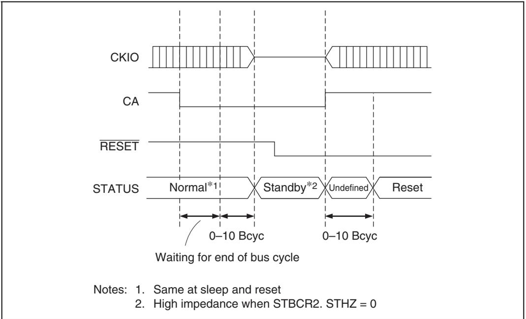
**Figure 9.12 Hardware Standby Mode Timing
