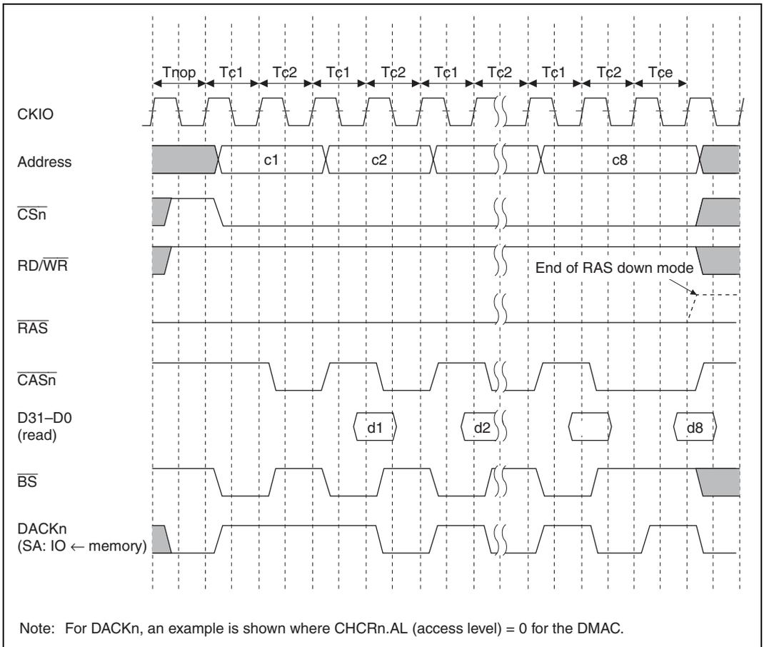
**Figure 13.19 (4) DRAM Burst Bus Cycle, RAS Down Mode Continuation
