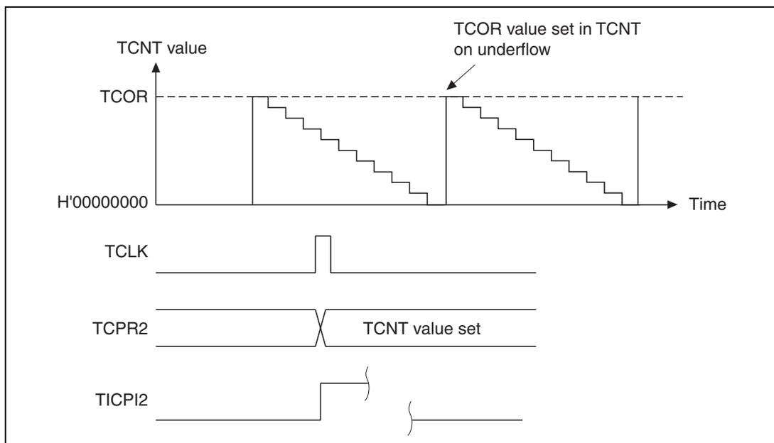
**Figure 12.7 Operation Timing when Using Input Capture Function**
