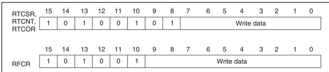
**Figure 13.5 Writing to RTCSR, RTCNT, RTCOR, and RFCR**
