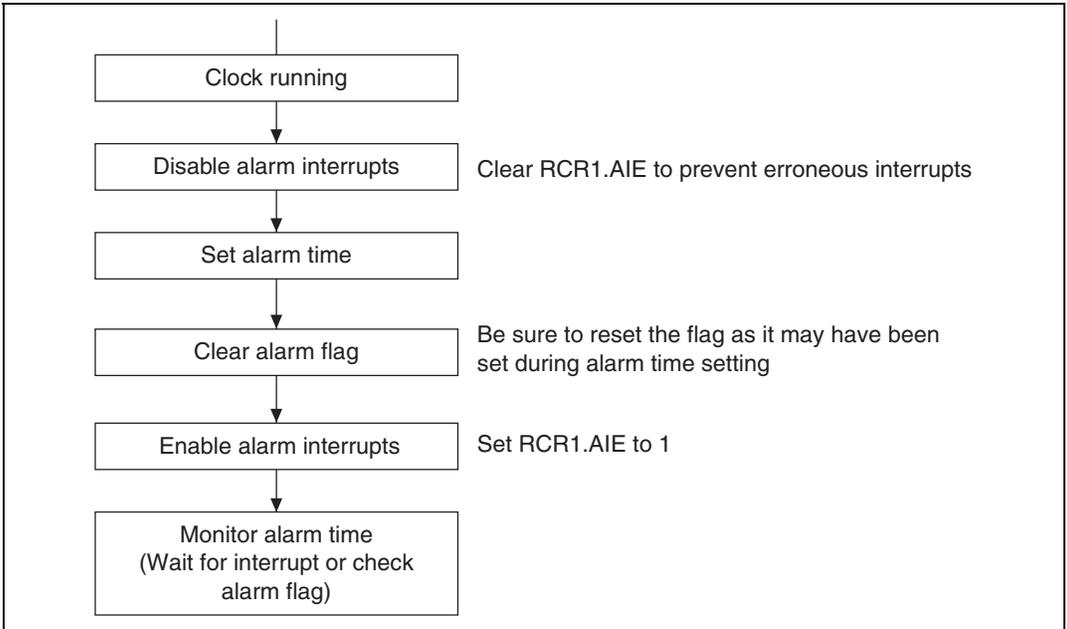
**Figure 11.4 Example of Use of Alarm Function**
