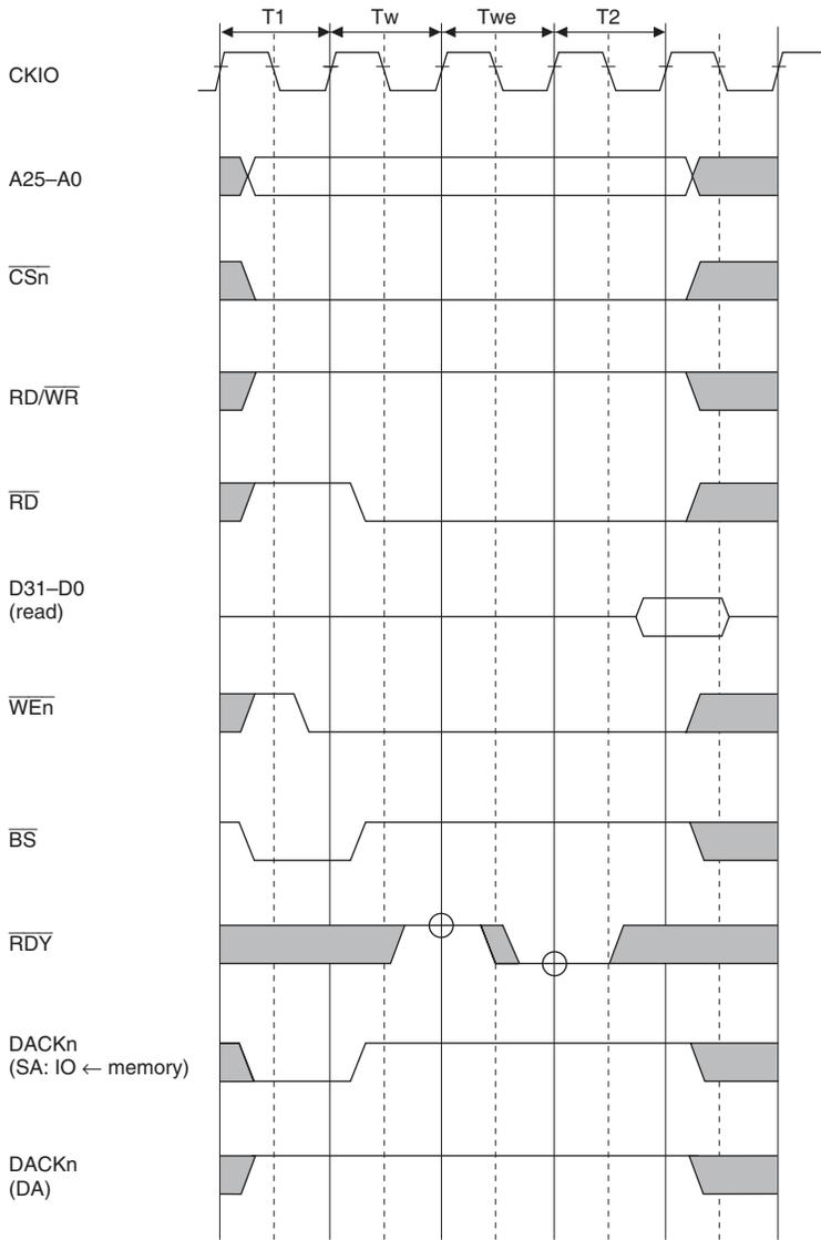
Note: For DACKn, an example is shown where CHCRn.AL (access level) = 0 for the DMAC.
