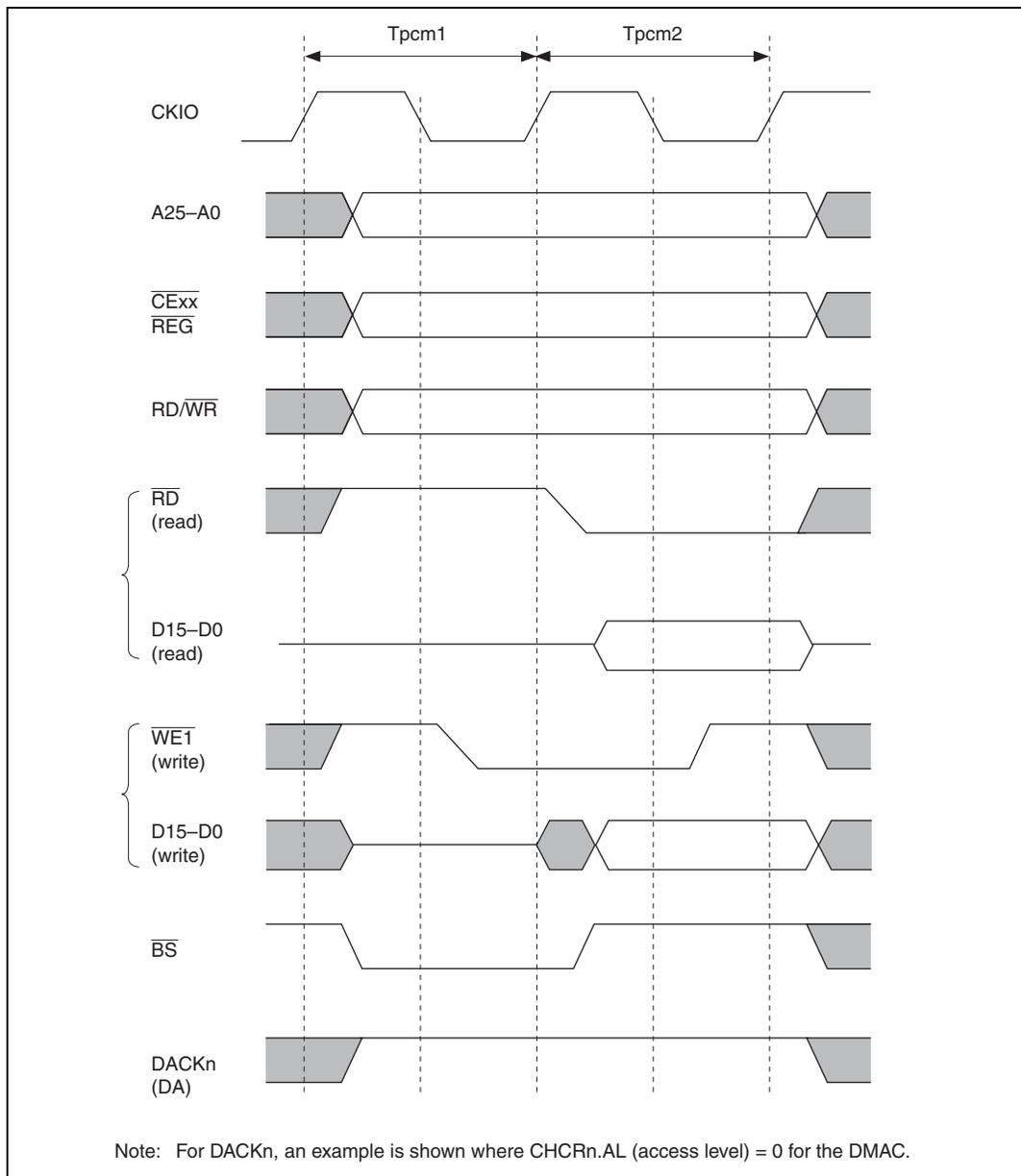
**Figure 13.45 Basic Timing for PCMCIA Memory Card Interface**
