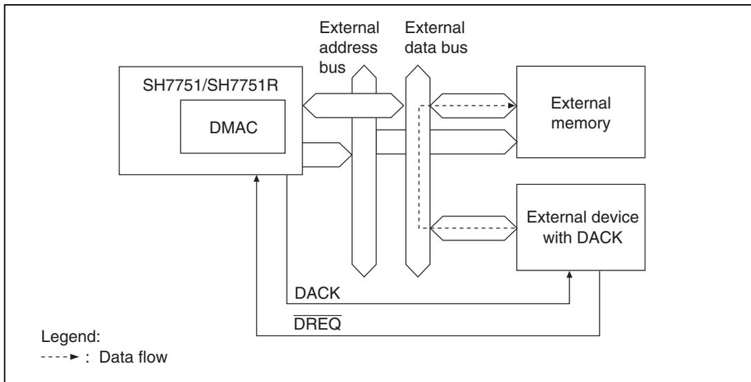
**Figure 14.5 Data Flow in Single Address Mode**
