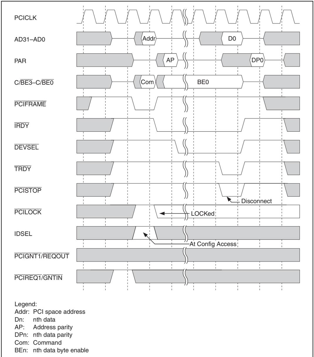
**Figure 22.11 Target Read Cycle in Non-Host Mode (Single)**
