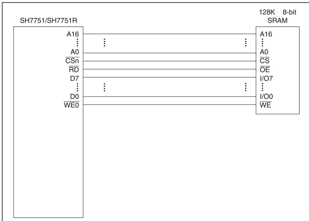
**Figure 13.9 Example of 8-Bit Data Width SRAM Connection**
