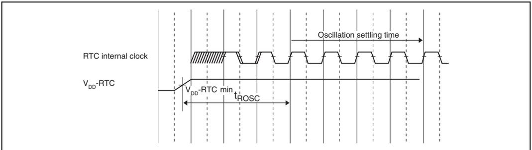
Figure 23.60 RTC Oscillation Settling Time at Power-On
