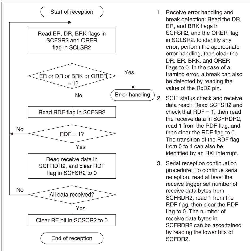
1. Receive error handling and break detection: Read the DR, ER, and BRK flags in SCFSR2, and the ORER flag in SCLSR2, to identify any error, perform the appropriate error handling, then clear the DR, ER, BRK, and ORER flags to 0. In the case of a framing error, a break can also be detected by reading the value of the RxD2 pin.
