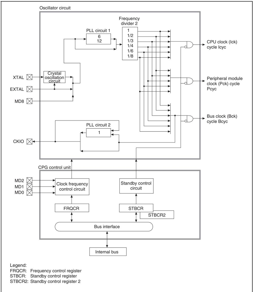
Figure 10.1 (2) Block Diagram of CPG (SH7751R)
