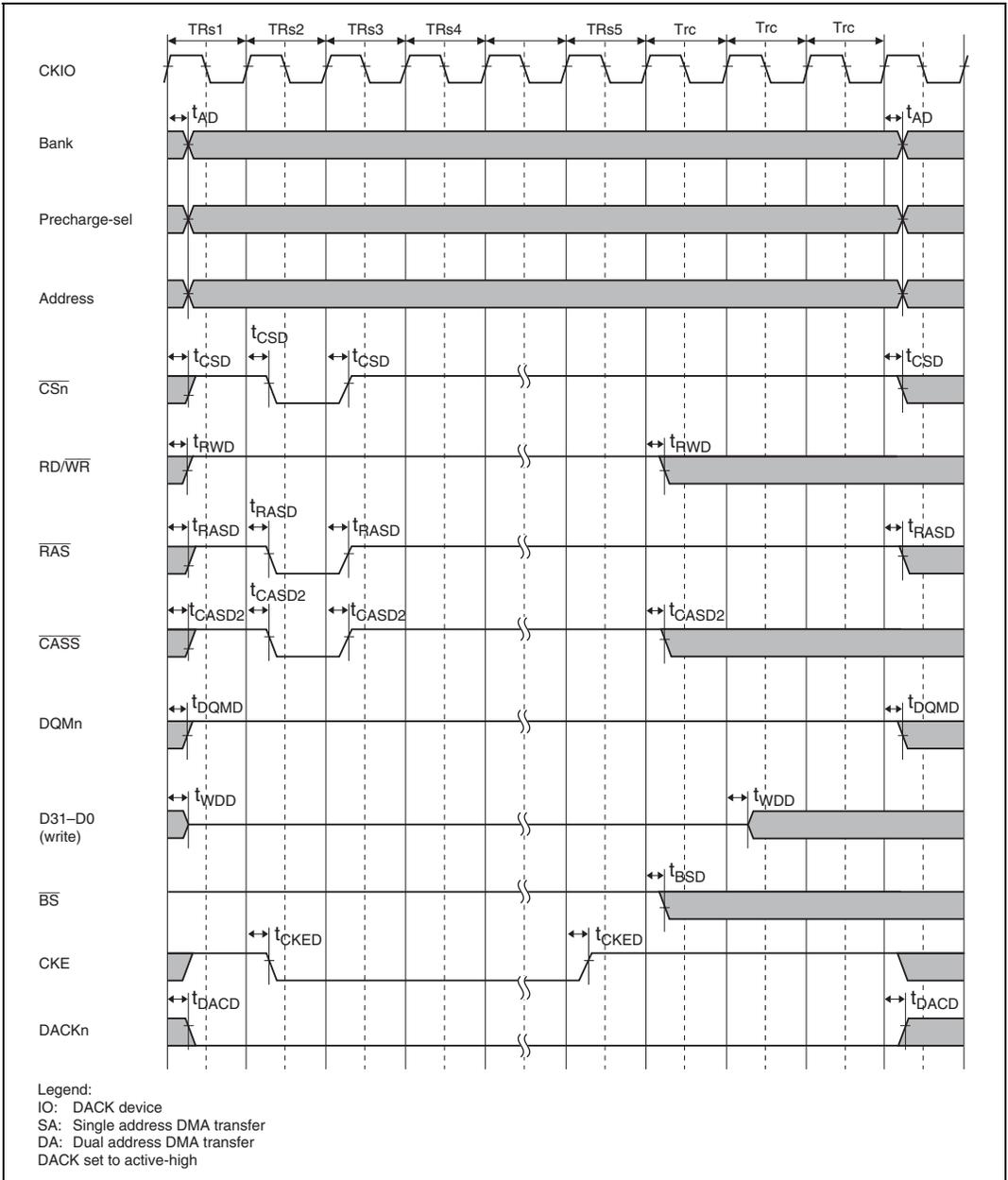
Figure 23.33 Synchronous DRAM Bus Cycle: Self-Refresh (TRC [2:0] = 001)
