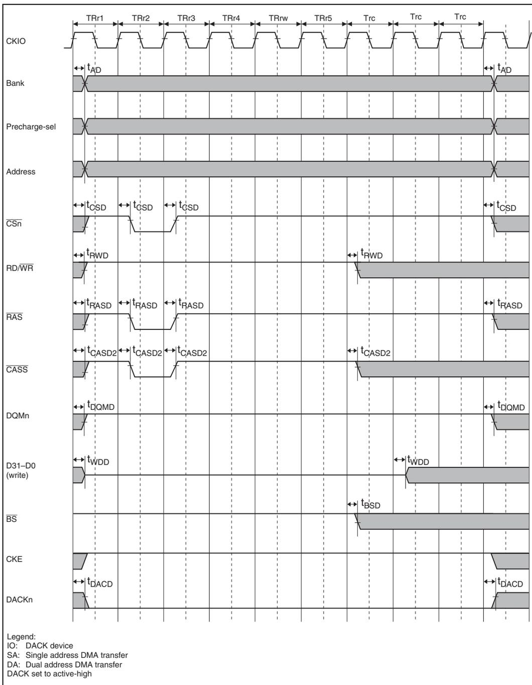
**Figure 23.32 Synchronous DRAM Bus Cycle: Auto-Refresh (TRAS = 1, TRC [2:0] = 001)**
