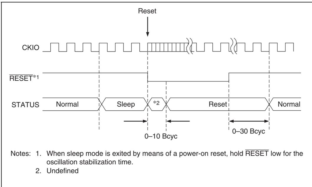
**Figure 9.7 STATUS Output in Sleep → Power-On Reset Sequence**
