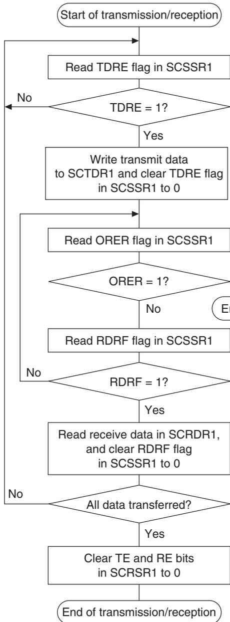
1. SCI status check and transmit data write:
