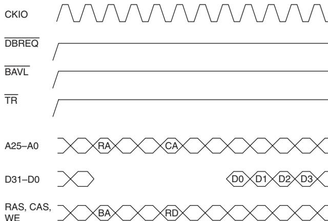
**Figure 14.35 Read from Synchronous DRAM Precharge Bank**
