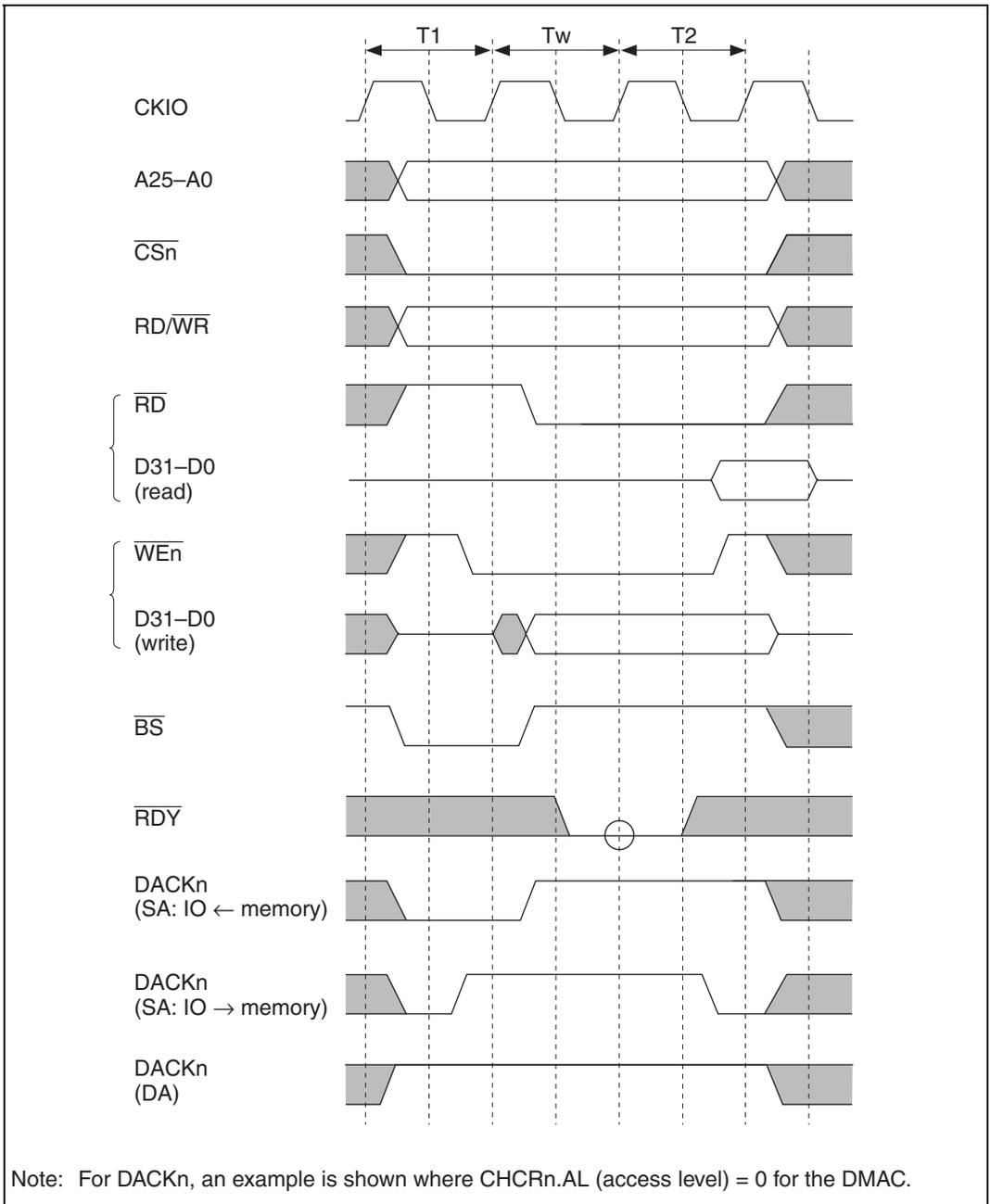
**Figure 13.10 SRAM Interface Wait Timing (Software Wait Only)**
