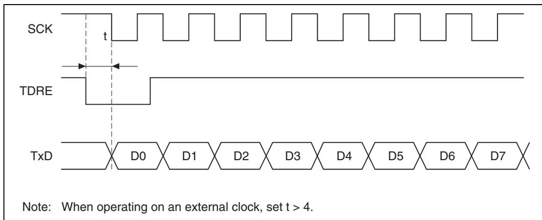
**Figure 15.26 Example of Synchronous Transmission by DMAC**
