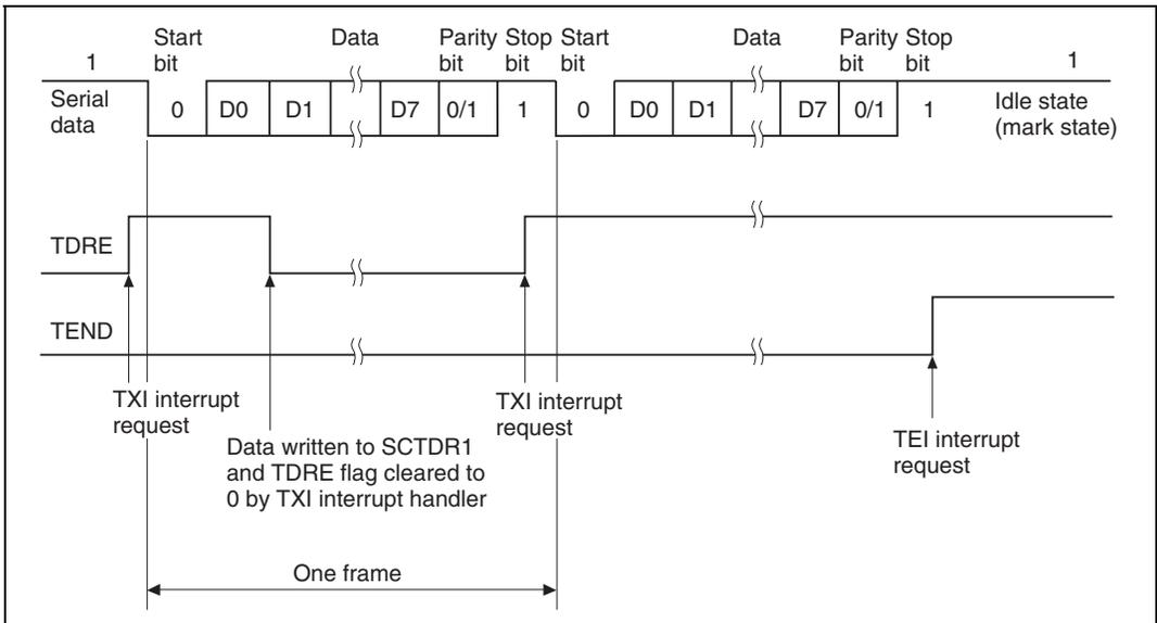
**Figure 15.9 Example of Transmit Operation in Asynchronous Mode
