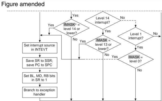
Note: \* IMASK: Interrupt mask bits in status register (SR)
