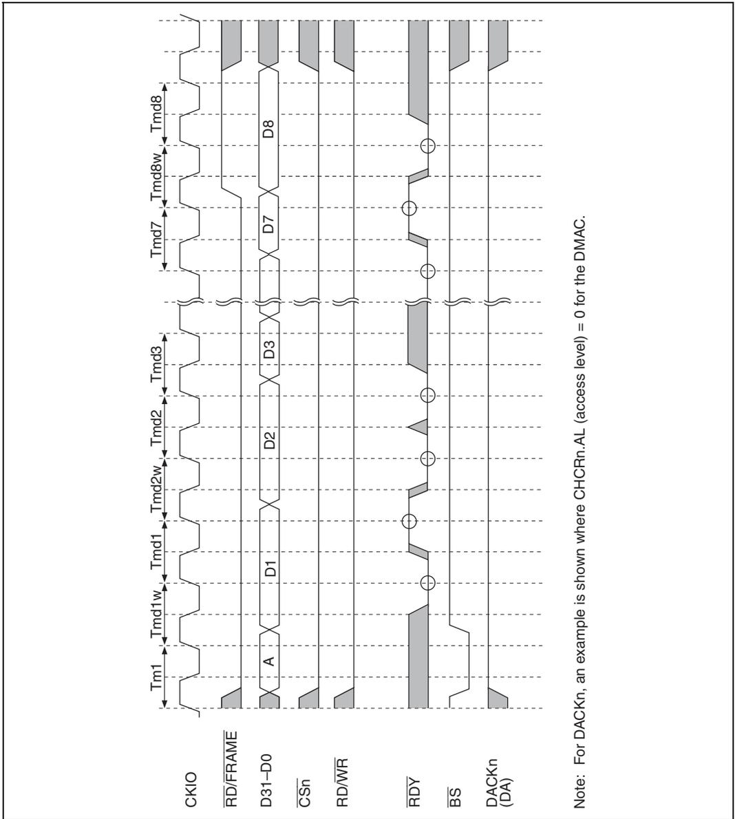
**Figure 13.59 MPX Interface Timing 8**
