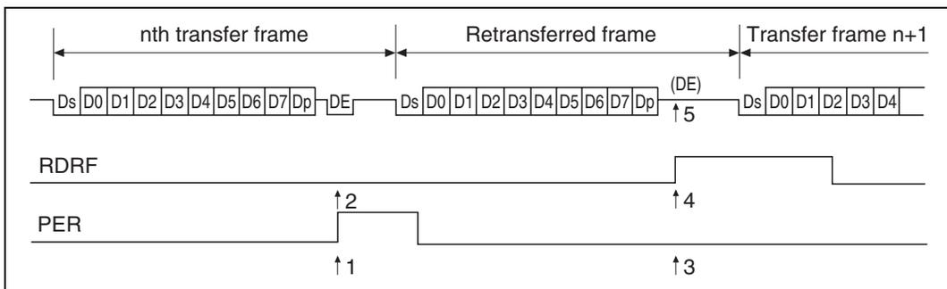
**Figure 17.11 Retransfer Operation in SCI Receive Mode**
