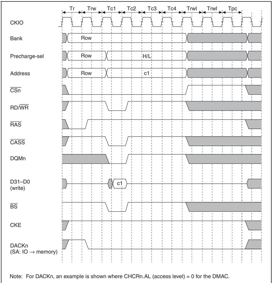
**Figure 13.27 Basic Timing for Synchronous DRAM Single Write**
