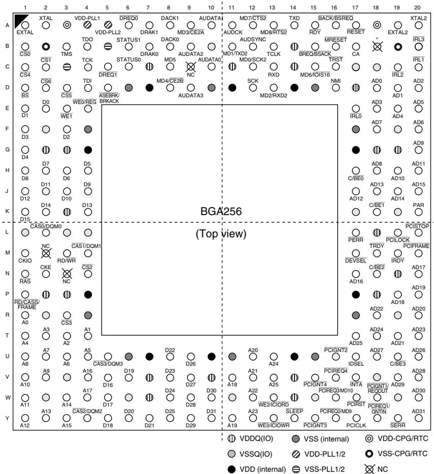
**Notes:** Power must be supplied to the on-chip PLL power supply pins (VDD-PLL1, VDD-PLL2, VSS-PLL1, VSS-PLL2, VDD-CPG, VSS-CPG, VDD-RTC, and VSS-RTC) regardless of whether or not the PLL circuits, crystal oscillation circuit, and RTC are used.
