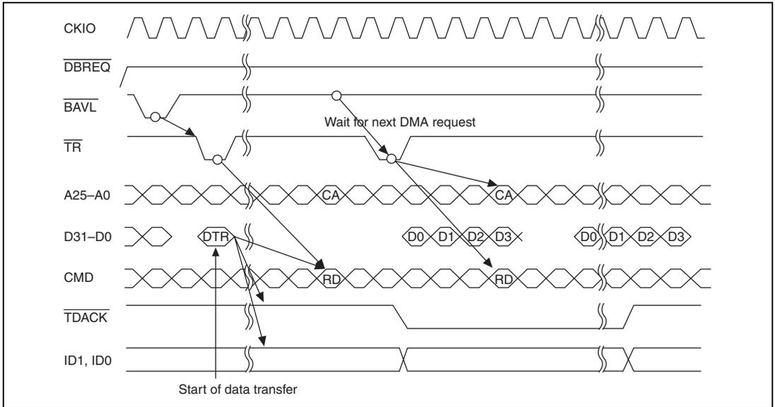
**Figure 14.44 Single Address Mode/Burst Mode/Level Detection/
