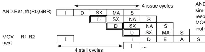
AND.B and MOV are fetched simultaneously, but MOV is stalled due to resource locking. After the lock is released, MOV is refetched together with the next instruction.
