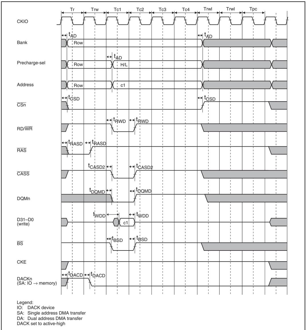
**Figure 23.26 Synchronous DRAM Auto-Precharge Write Bus Cycle: Single**
