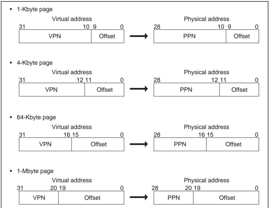
**Figure 3.8 Relationship between Page Size and Address Format**
