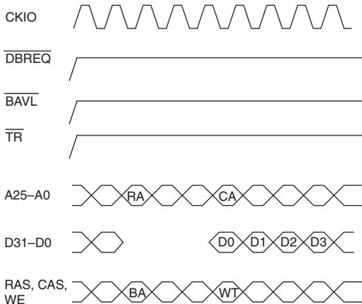
**Figure 14.38 Write to Synchronous DRAM Precharge Bank**
