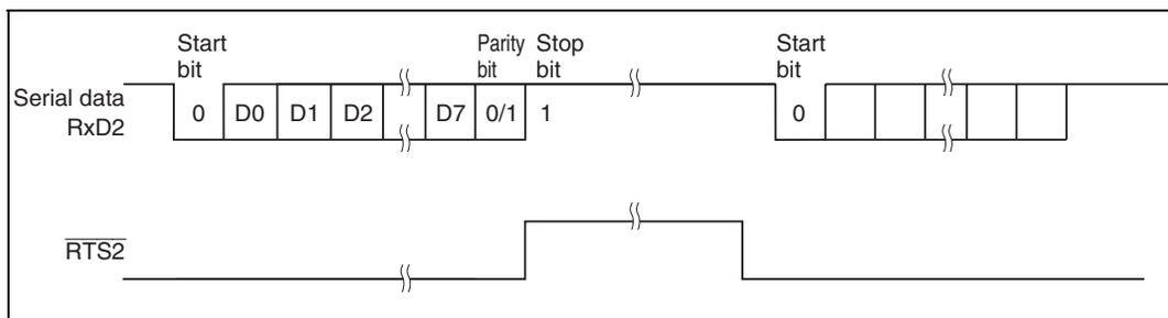
**Figure 16.13 Example of Operation Using Modem Control ( $\overline{\text{RTS2}}$ )**
