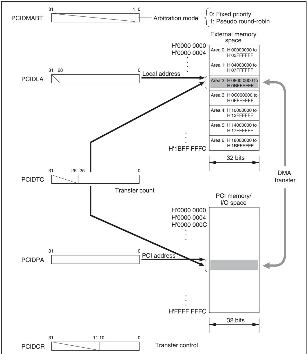
Figure 22.5 Example of DMA Transfer Control Register Settings
