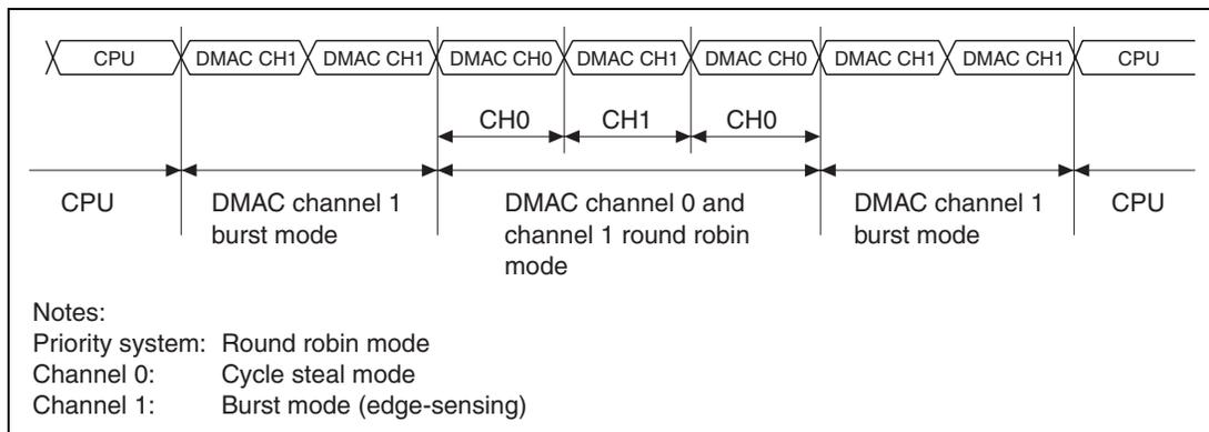
**Figure 14.11 Bus Handling with Two DMAC Channels Operating**
