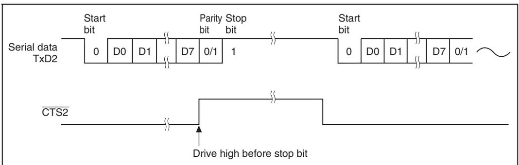
**Figure 16.10 Example of Operation Using Modem Control ( $\overline{\text{CTS2}}$ )**
