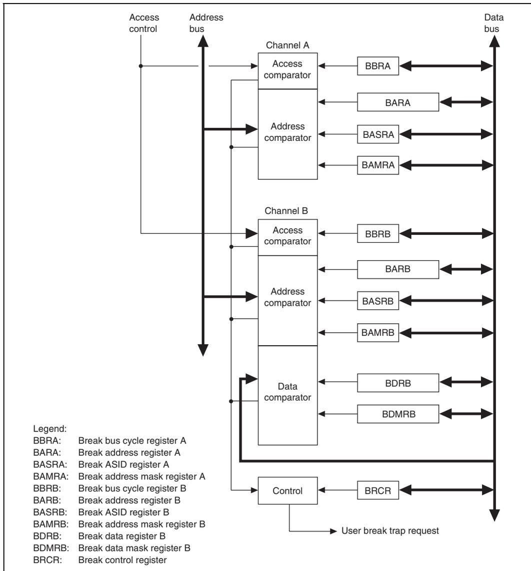
**Figure 20.1 Block Diagram of User Break Controller**
