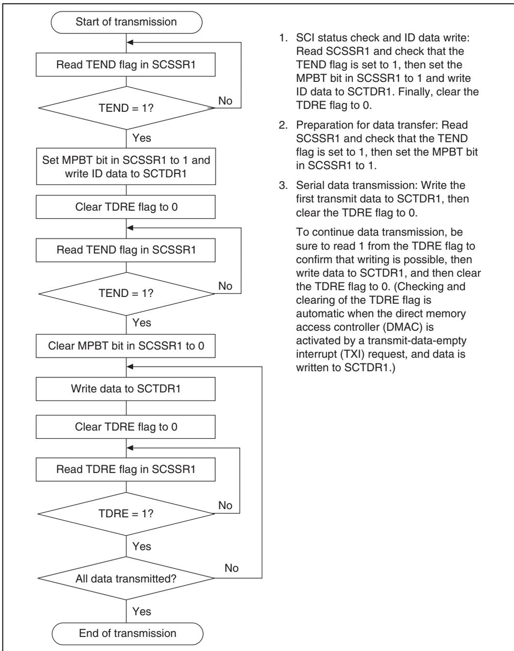
1. SCI status check and ID data write: Read SCSSR1 and check that the TEND flag is set to 1, then set the MPBT bit in SCSSR1 to 1 and write ID data to SCTDR1. Finally, clear the TDRE flag to 0.
