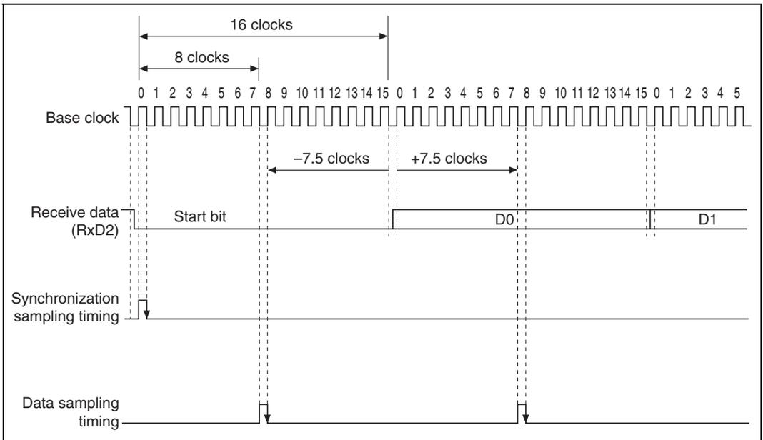
**Figure 16.14 Receive Data Sampling Timing in Asynchronous Mode**
