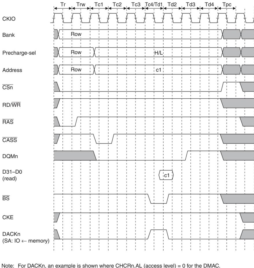
**Figure 13.25 Basic Timing for Synchronous DRAM Single Read**
