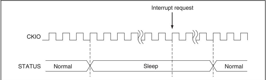
Figure 9.9 STATUS Output in Deep Sleep → Interrupt Sequence
