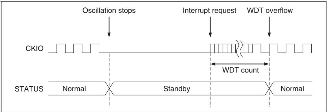
Figure 9.3 STATUS Output in Standby → Interrupt Sequence
