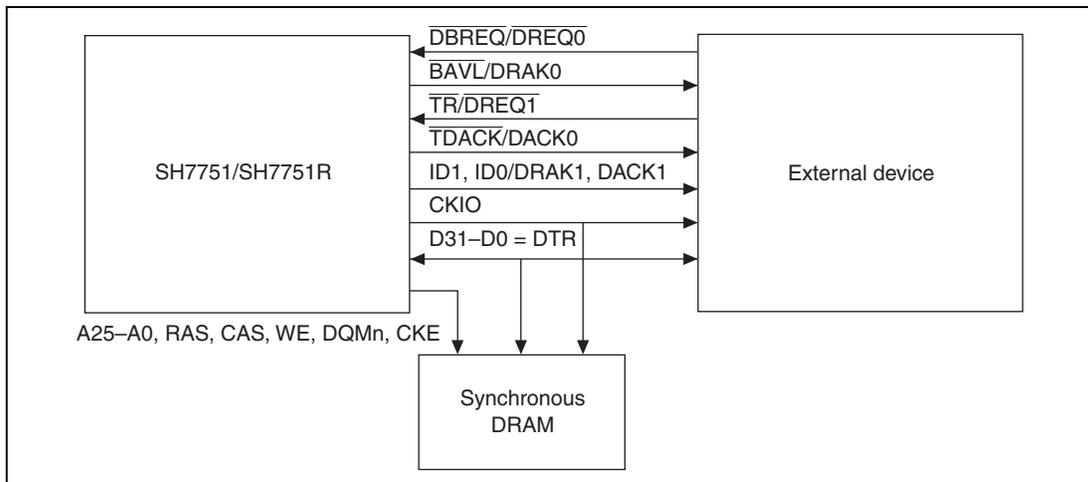
**Figure 14.24 System Configuration in On-Demand Data Transfer Mode**
