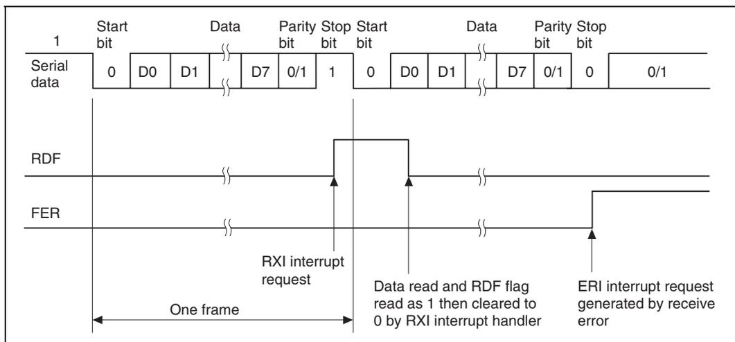
**Figure 16.12 Example of SCIF Receive Operation
