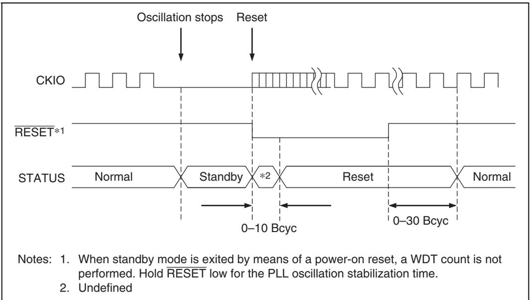
Notes: 1. When standby mode is exited by means of a power-on reset, a WDT count is not performed. Hold RESET low for the PLL oscillation stabilization time.
