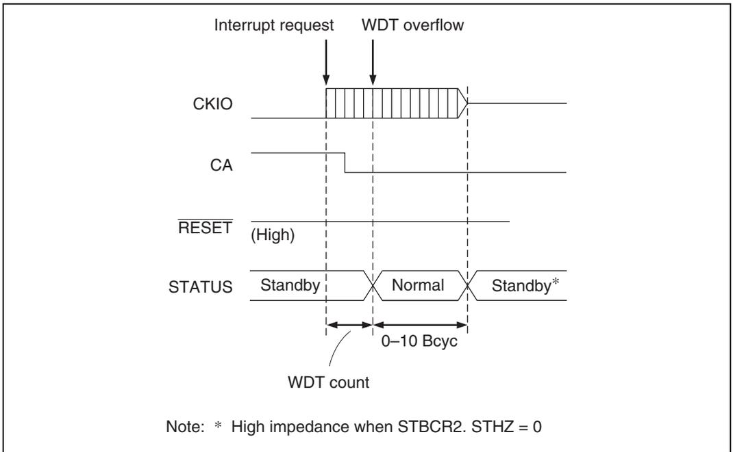
**Figure 9.13 Hardware Standby Mode Timing
