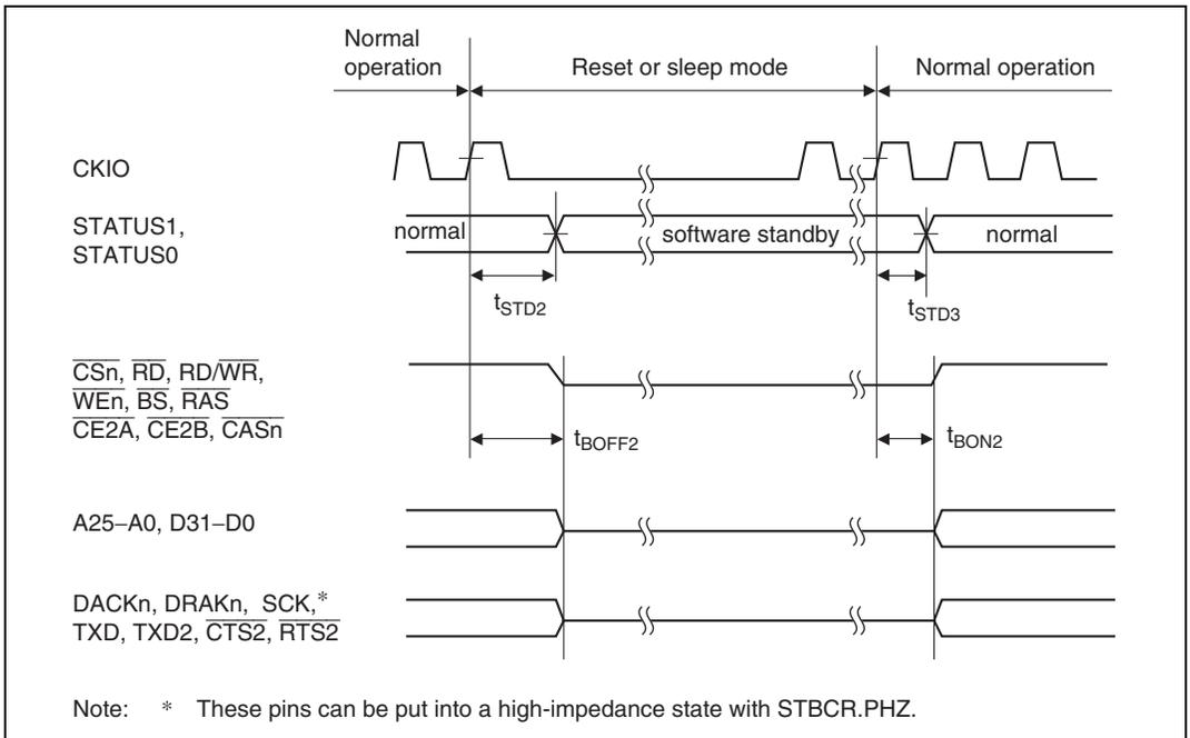
**Figure 23.12 (2) Pin Drive Timing for Software Standby Mode**
