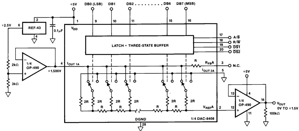
Figure 8. Unipolar Supply, Voltage Output DAC Operation
