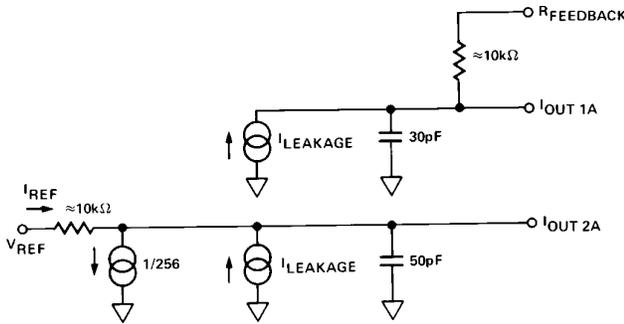
Figure 4. Equivalent DAC Circuit (All Digital Inputs LOW)
