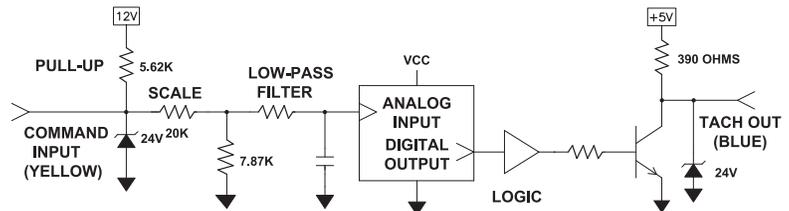
DC Impellers can be speed controlled via the yellow input lead in either of two ways:
