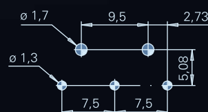
Drilling pattern for PCB terminal 0,6x0,5 mm lateral with location pins
