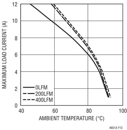
Figure 13. 12V<sub>IN</sub>, 3.3V<sub>OUT</sub>, No Heat Sink
