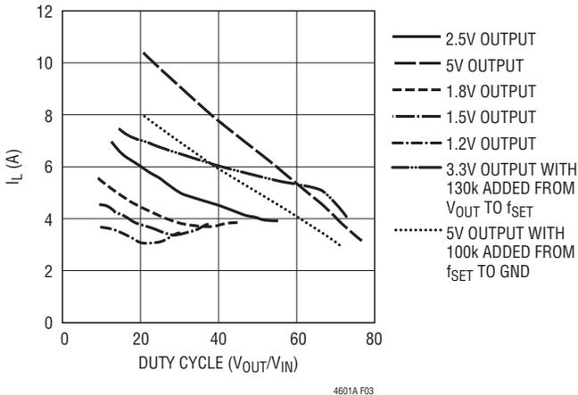
Figure 3. Inductor Ripple Current vs Duty Cycle
