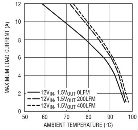
Figure 12. BGA Heat Sink 12V<sub>IN</sub>
