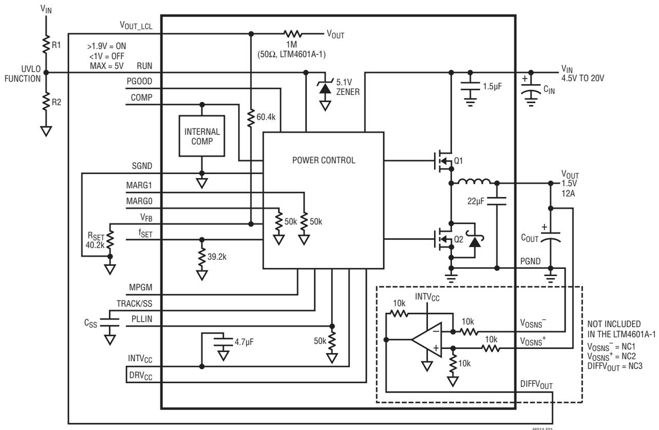
Figure 1. Simplified LTM4601A/LTM4601A-1 Block Diagram
