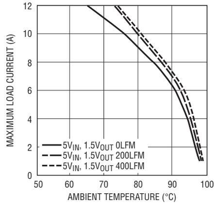
Figure 10. BGA Heat Sink 5V<sub>IN</sub>
