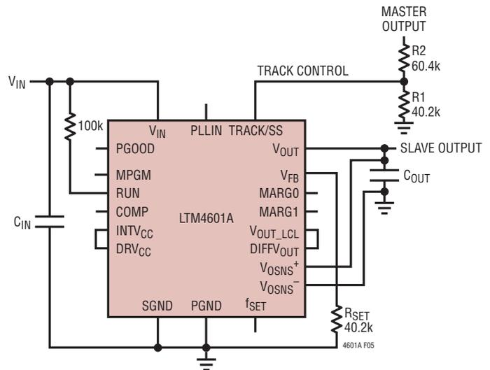
Figure 5. Coincident Tracking
