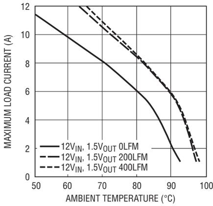
Figure 11. No Heat Sink 12V<sub>IN</sub>
