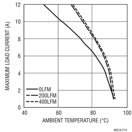
Figure 14. 12V<sub>IN</sub>, 3.3V<sub>OUT</sub>, BGA Heat Sink
