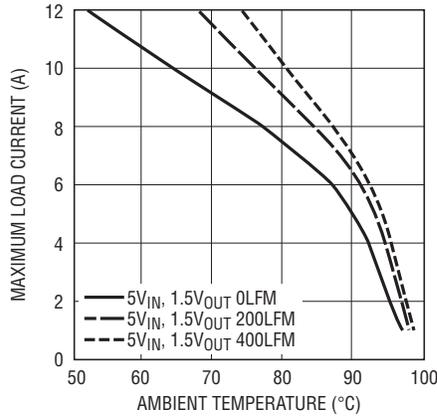
Figure 9. No Heat Sink 5V<sub>IN</sub>
