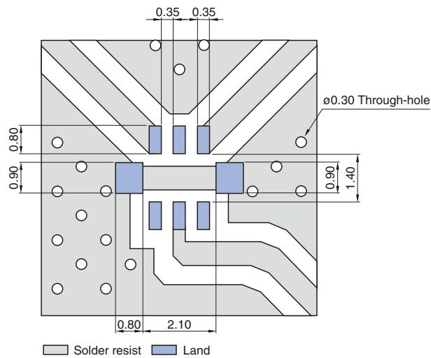
Line width be designed to match 50Ω characteristic impedance
