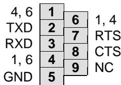
Female DB9 connector that interfaces to the MCU internal SCI0 serial port via the RS232 transceiver. Flow control is provided at test points on the board.
