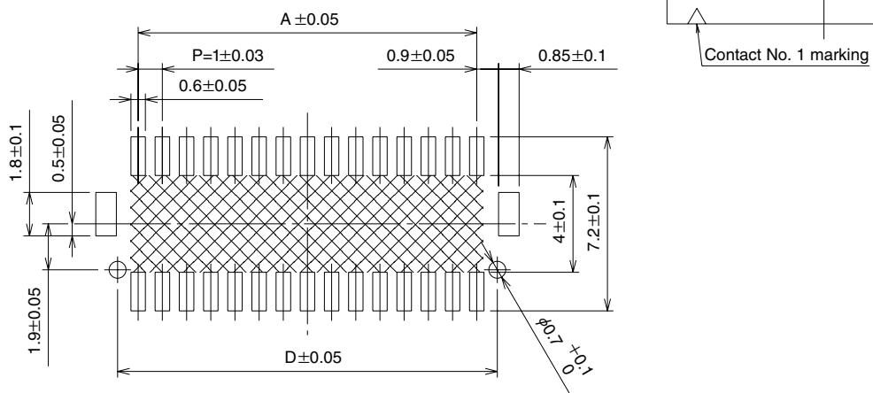
Note 1: Shaded area must be free of any electrically conductive traces to avoid contact with soldered pin header terminations.
