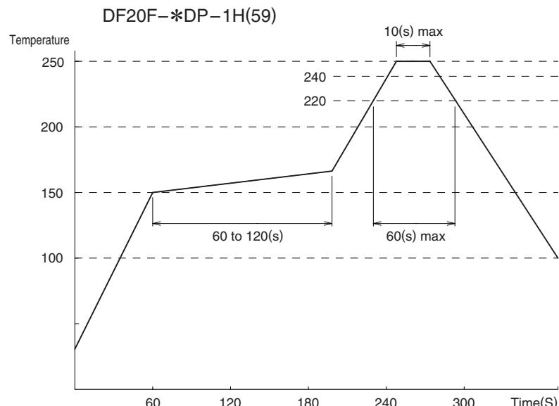
Note 1: Up to 2 cycles of reflow soldering are possible under the same conditions, provided that there is a return to normal temperature between the first and second cycle.
