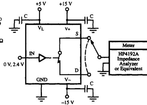
**Figure 7.** Source/Drain Capacitances
