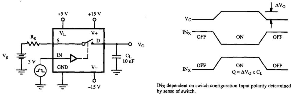
$IN_x$  dependent on switch configuration Input polarity determined by sense of switch.
