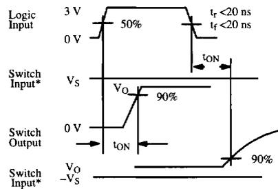
\* $V_S = 10V$  for  $t_{ON}$ ,  $V_S = -10V$  for  $t_{OFF}$
