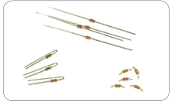
A range of NTC chip thermistors in DO-35 style glass package (diode outline) with axial solder-coated copper-clad steel wires.
