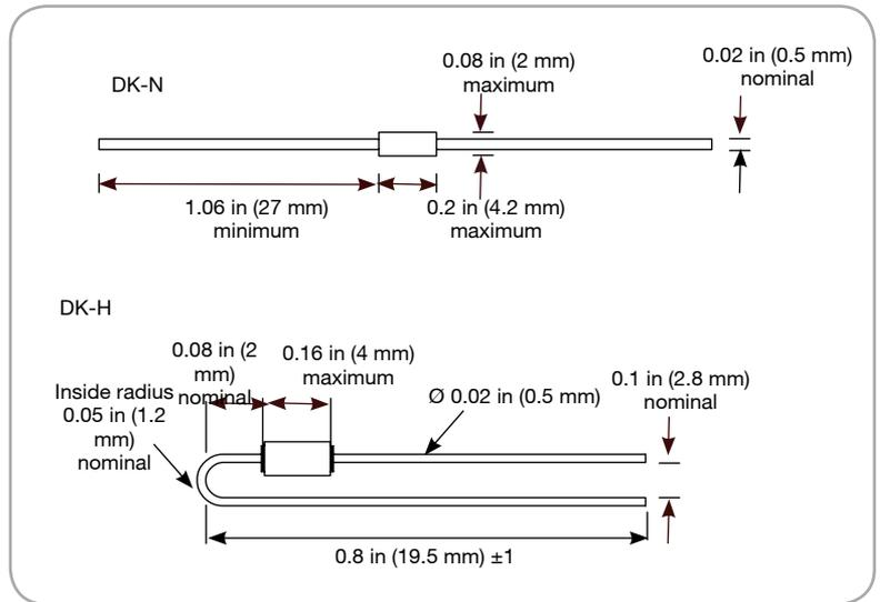
*NTC Type DK wires should not be bent within 0.08 in (2 mm) of glass body*
