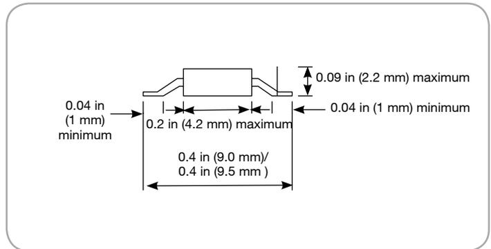
*NTC Type DKM wires should not be bent within 0.08 in (2 mm) of glass body*
