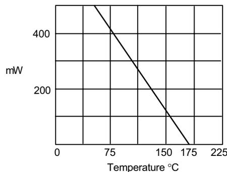
Power Dissipation (mW) - Versus - Ambient Temperature °C
