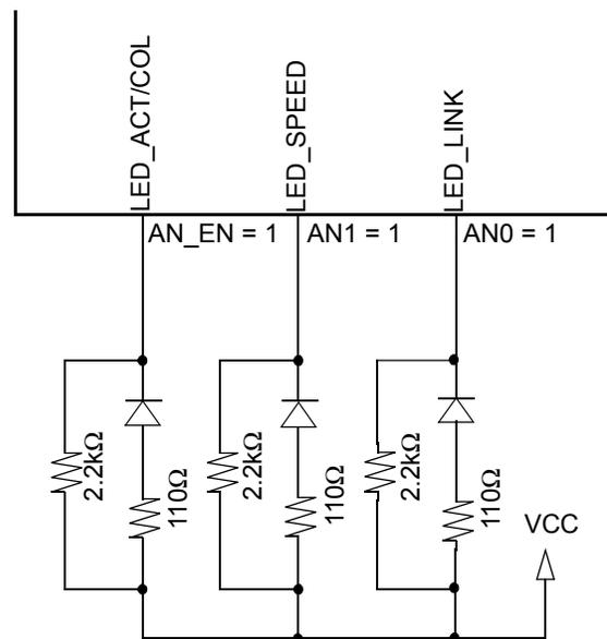
**Figure 3. AN Strapping and LED Loading Example**
