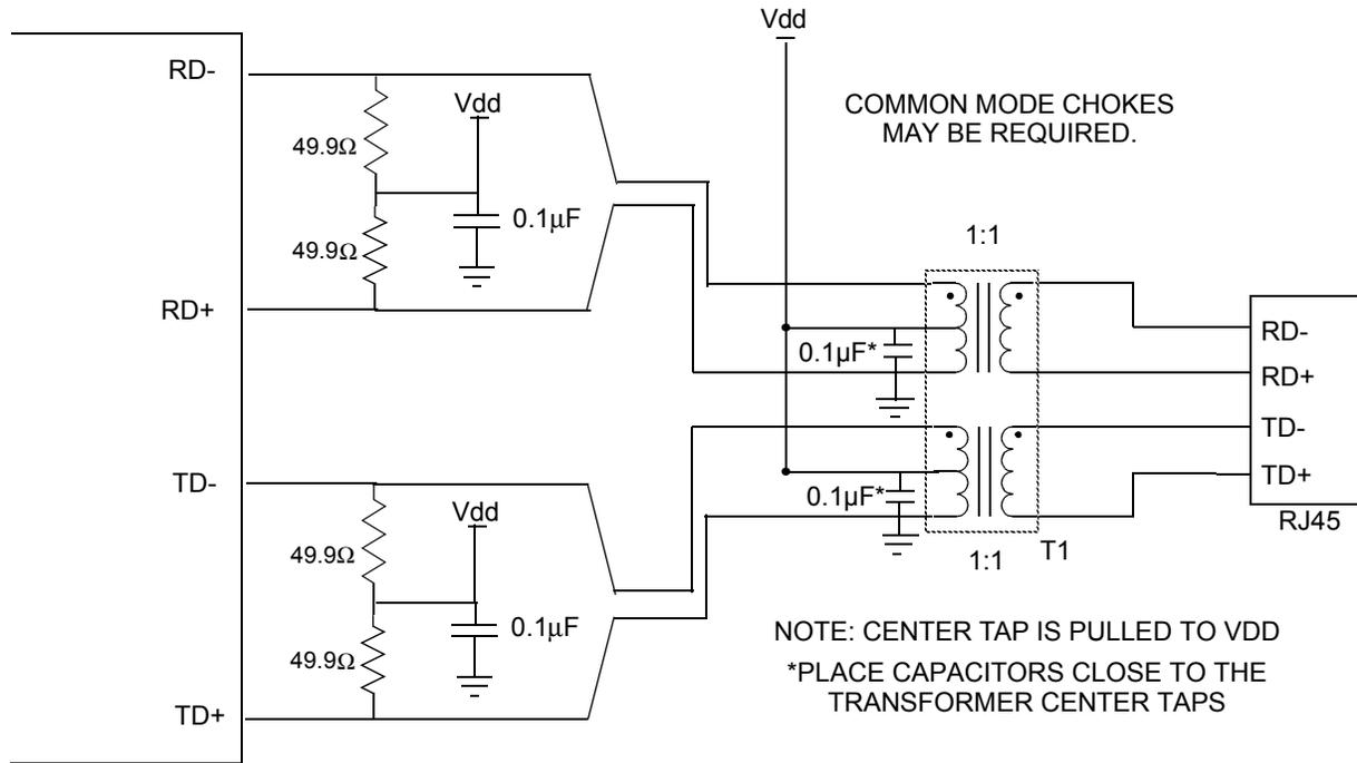
PLACE RESISTORS AND CAPACITORS CLOSE TO THE DEVICE.
