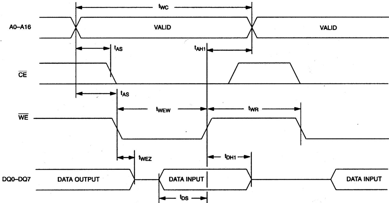
**WRITE CYCLE TIMING DIAGRAM, CHIP ENABLE CONTROLLED**
