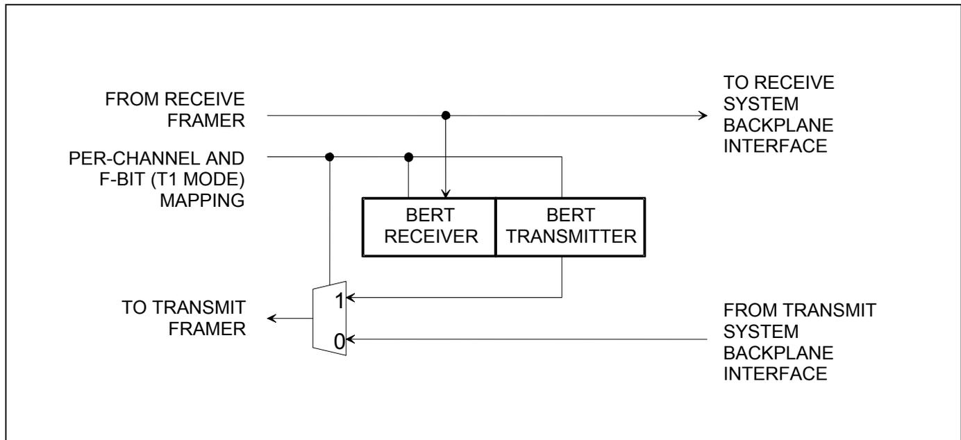
**Figure 26-2. Simplified Diagram of BERT in Backplane Direction**
