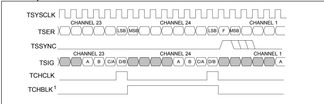
**Note 1:** TCHBLK is programmed to block channel 24 (if the TPCSI bit is set, then the signaling data at TSIG is ignored during channel 24).
