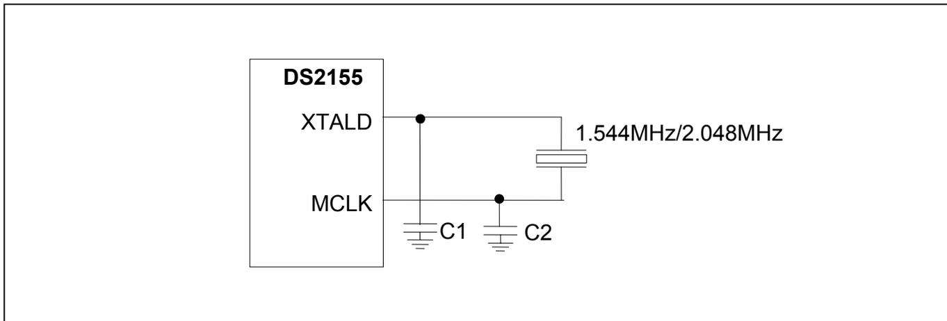
**Note 1:** C1 and C2 should be 5pF lower than two times the nominal loading capacitance of the crystal to adjust for the input capacitance of the DS2155.
