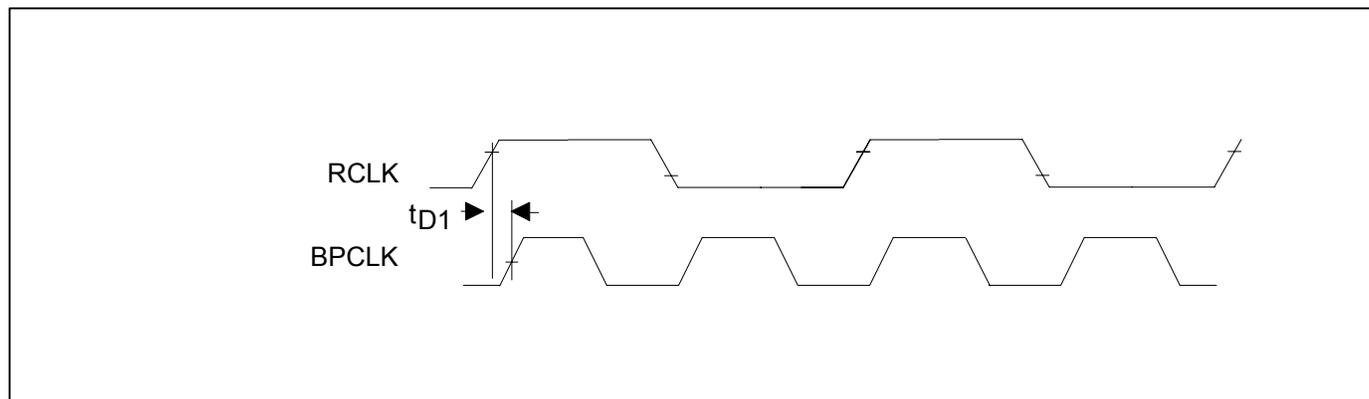
**Note 1:** If RCLK is 1.544 MHz, BPCLK will be asynchronous.
