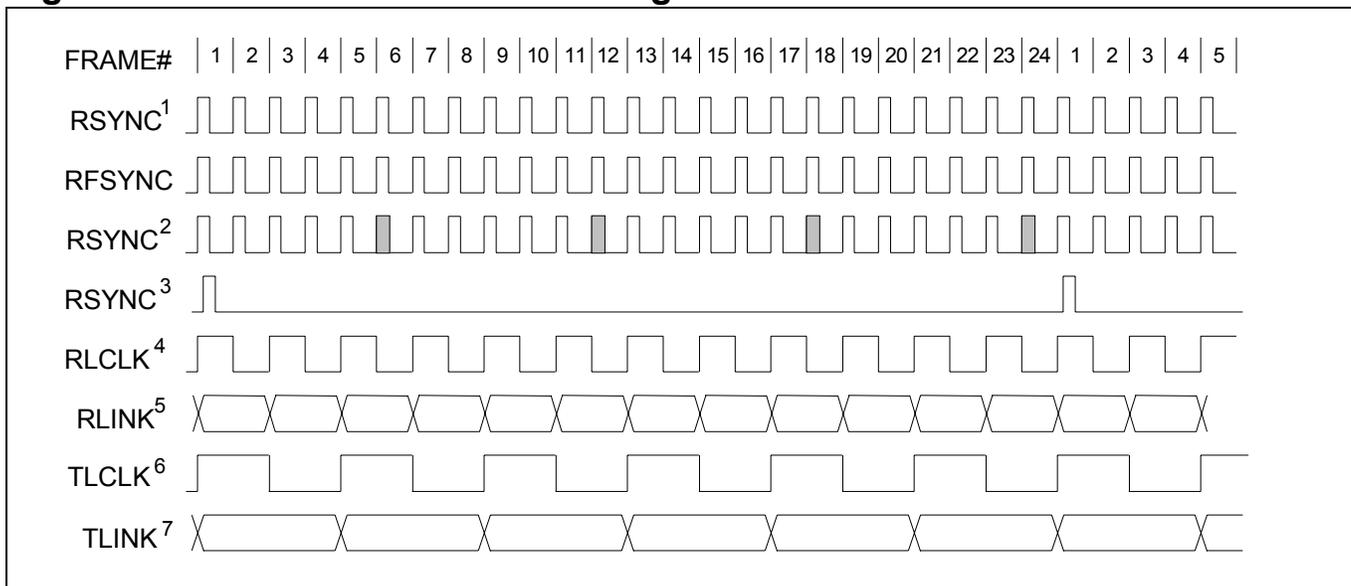
**Note 1:** RSYNC in frame mode (IOCR1.4 = 0) and double-wide frame sync is not enabled (IOCR1.6 = 0).
