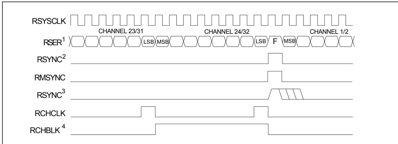
**Note 1:** Data from the E1 channels 1, 5, 9, 13, 17, 21, 25, and 29 is dropped (channel 2 from the E1 link is mapped to channel 1 of the T1 link, etc.) and the F-bit position is added (forced to on 1).
