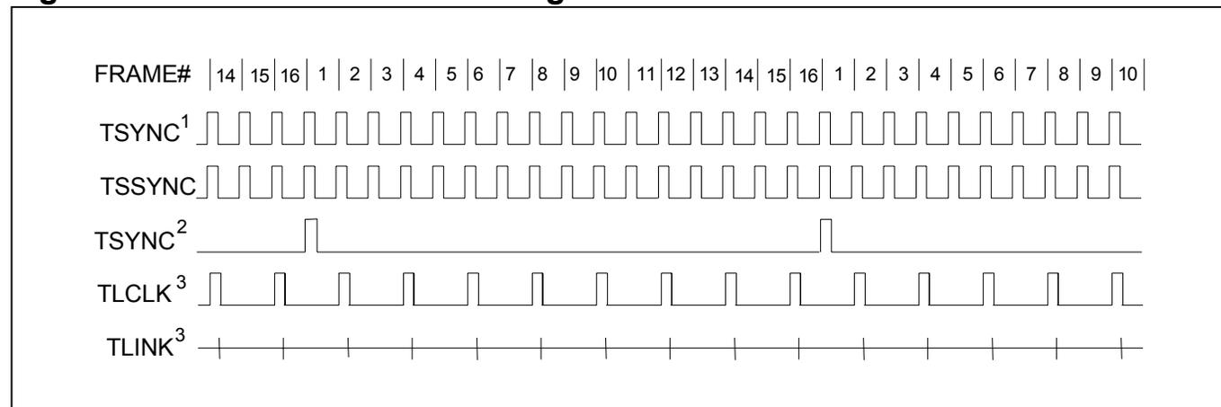
**Note 1:** TSYNC in frame mode (IOCR1.2 = 0).
