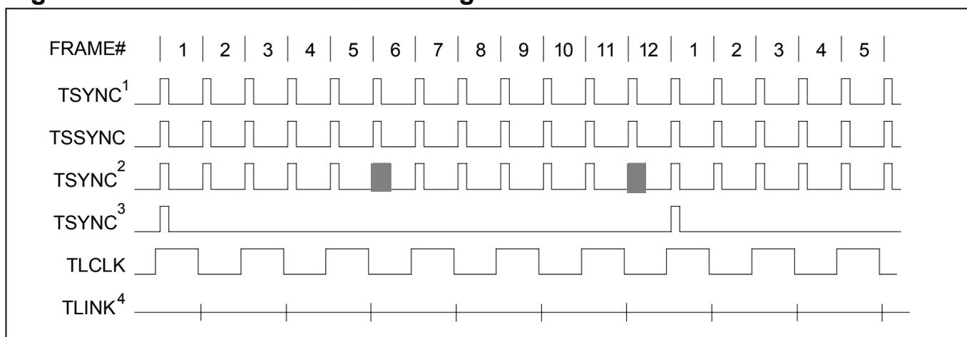
**Note 1:** TSYNC in the frame mode (IOCR1.2 = 0) and double-wide frame sync is not enabled (IOCR1.1 = 0).
