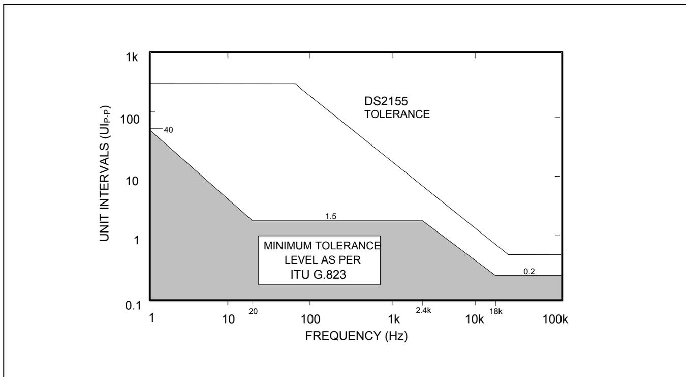
**Figure 24-9. Jitter Attenuation (T1 Mode)**
