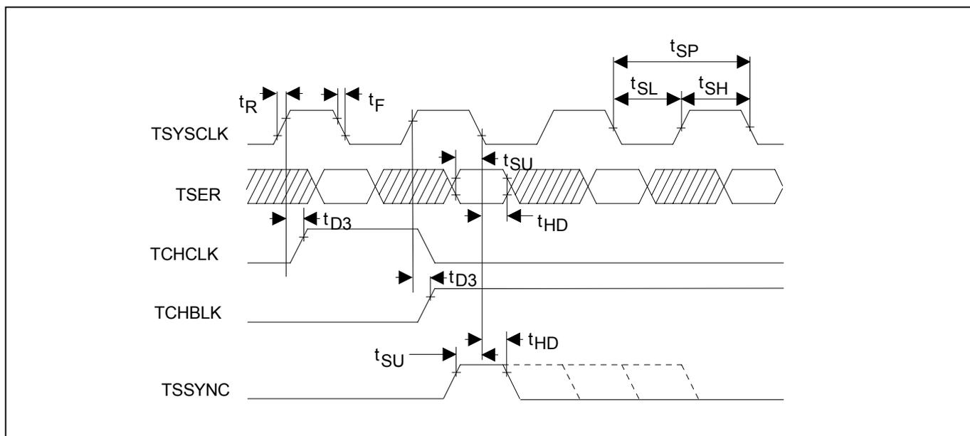
**Note 1:** TSER is only sampled on the falling edge of TSYCLK when the transmit-side elastic store is enabled.
