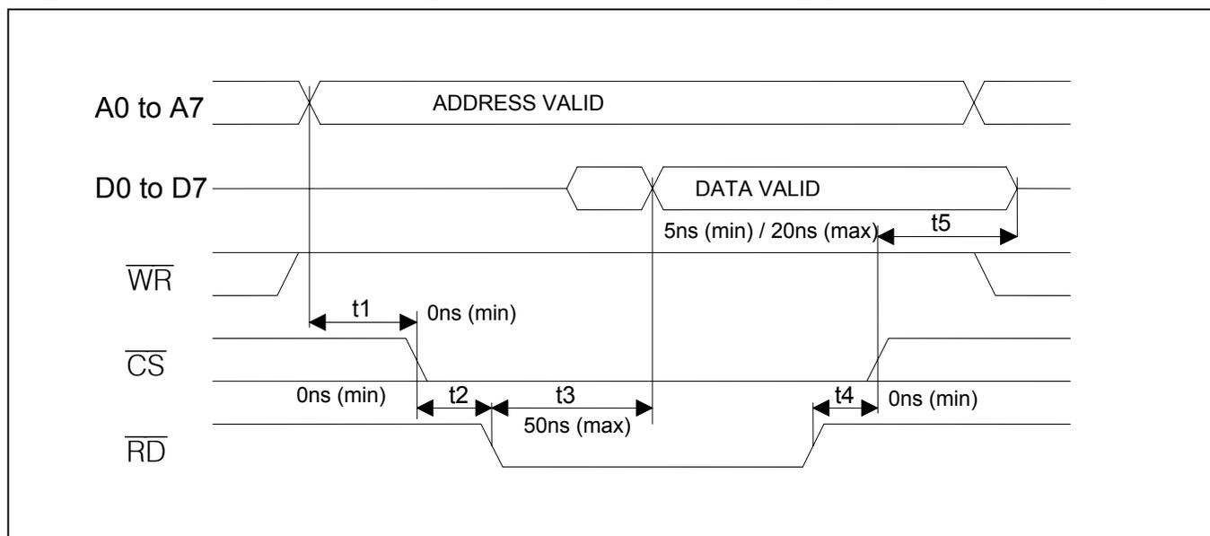
**Figure 37-5. Intel Nonmultiplexed Bus Write Timing (BTS = 0/MUX = 0)**
