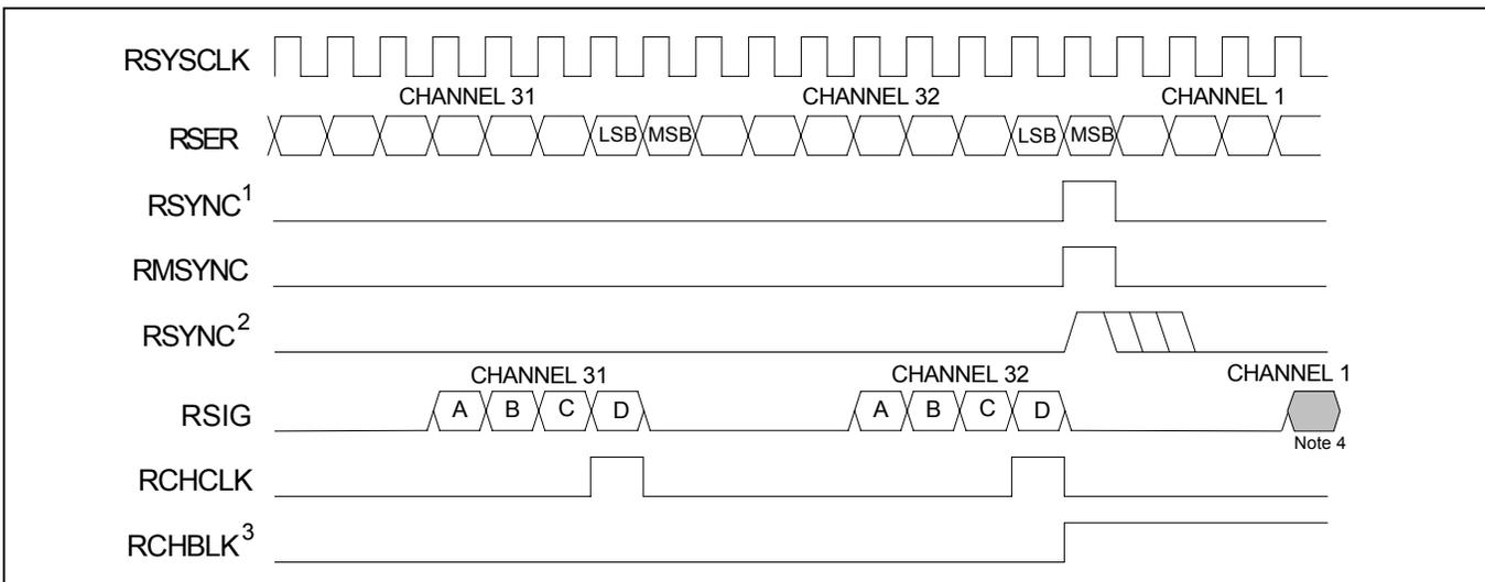
**Note 1:** RSYNC is in the output mode (IOCR1.4 = 0).
