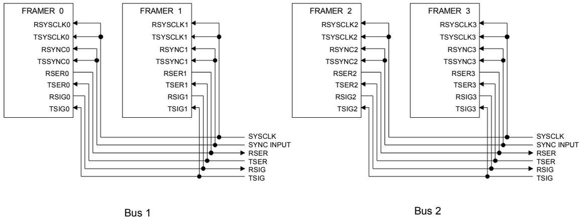
**Figure 18-2. 8.192MHz INTERLEAVED BUS EXTERNAL PIN CONNECTION EXAMPLE**
