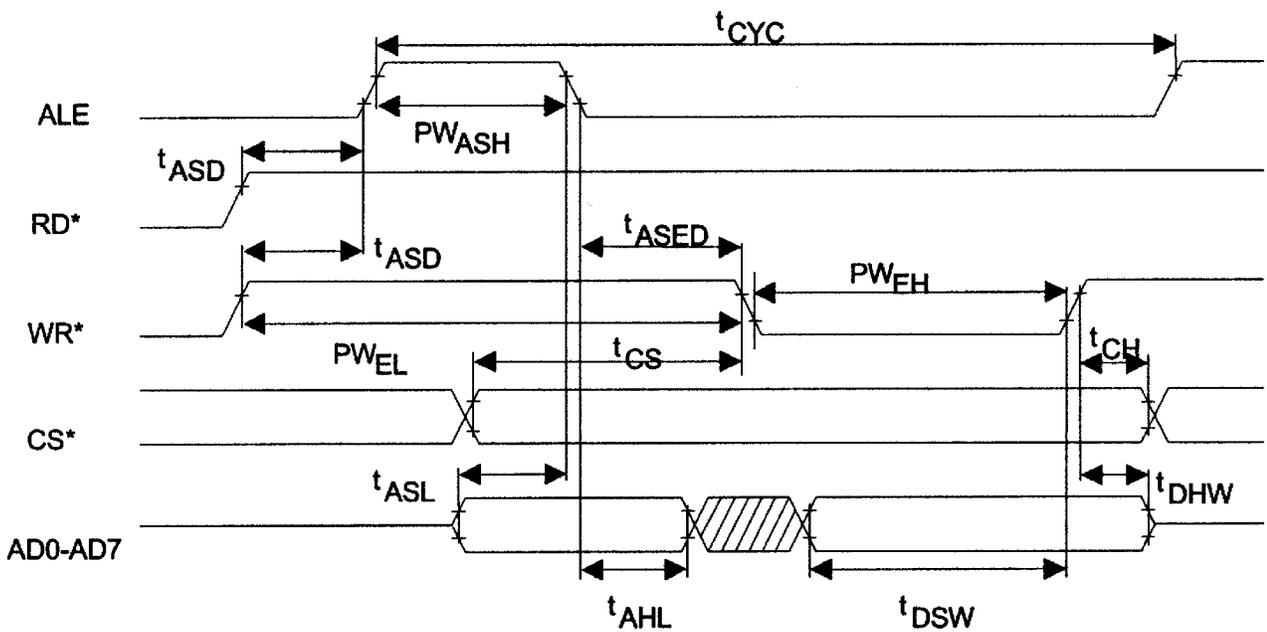
Figure 21-3. MOTOROLA BUS AC TIMING (BTS = 1 / MUX = 1)
