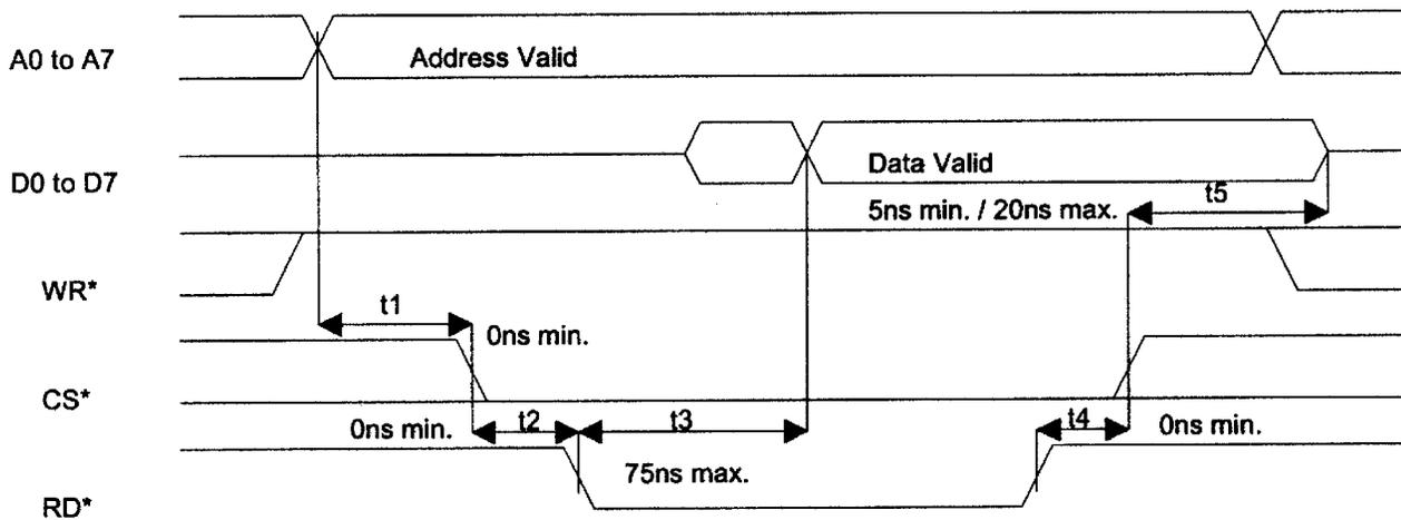
**Figure 21-5. INTEL BUS WRITE AC TIMING (BTS = 0 / MUX = 0)**
