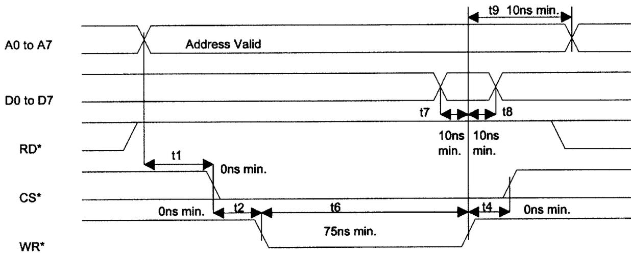
**Figure 21-6. MOTOROLA BUS READ AC TIMING (BTS = 1 / MUX = 0)**
