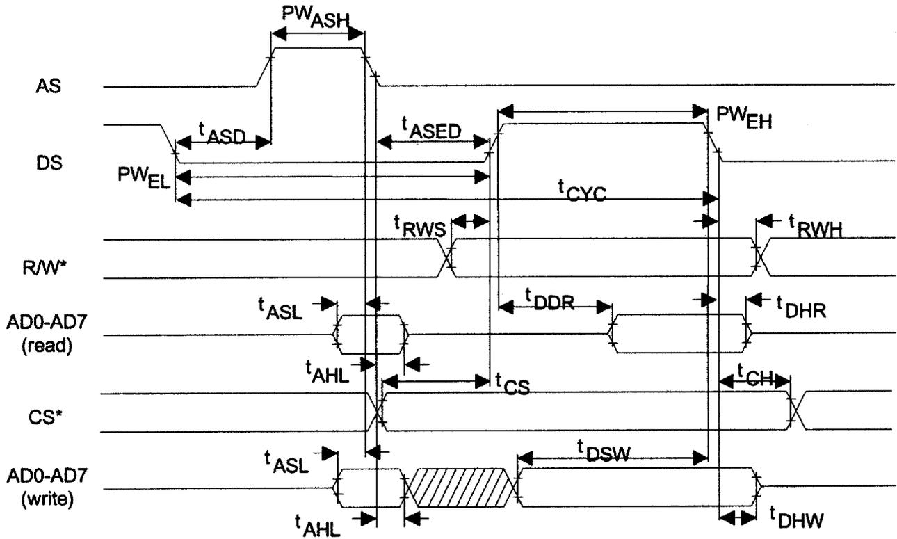
Figure 21-4. INTEL BUS READ AC TIMING (BTS = 0 / MUX = 0)
