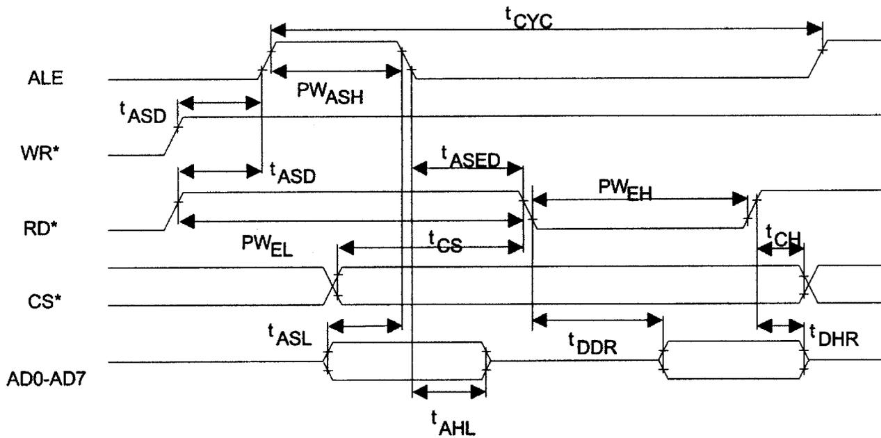
Figure 21-2. INTEL BUS WRITE TIMING (BTS = 0 / MUX = 1)
