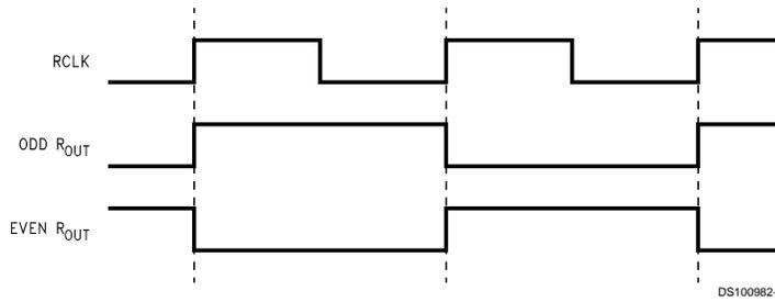
FIGURE 1. "Worst Case" Deserializer ICC Test Pattern
