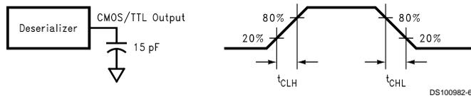
FIGURE 2. Deserializer CMOS/TTL Output Load and Transition Times
