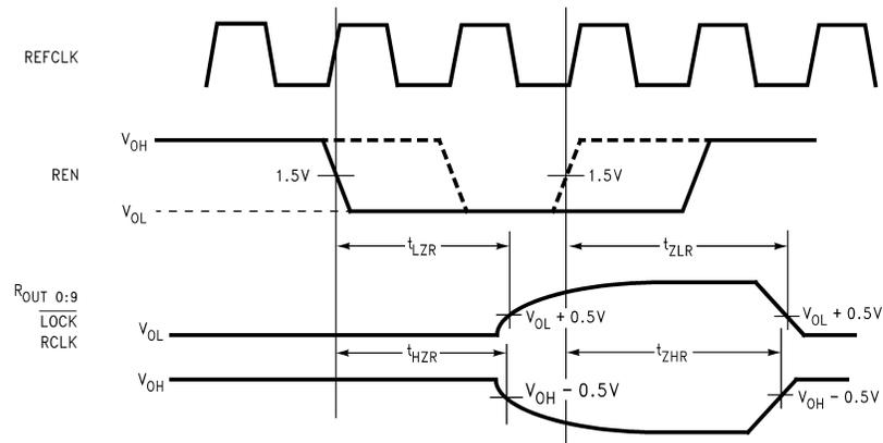
**FIGURE 6. Deserializer TRI-STATE Test Circuit and Timing**
