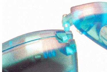
**\*Note:** The data contact faces down and away from the embossed 'i'. Once the iButton is inserted in the enclosure, snap the end cap over it. The end cap is removed by depressing the release tab with a paper clip, swinging it fully open, and sliding out the hinge.
