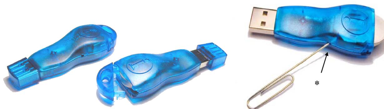
**\*Note:** To eject an *i*Button, insert a straightened paper clip into the side access hole of the DS9490B. Push the paper clip in the direction of the *i*Button. A different *i*Button can then be inserted. The data contact faces down and away from the embossed 'i'. Before inserting the paper clip disconnect the DS9490B from the USB bus.
