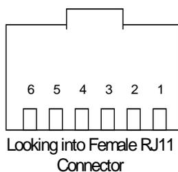
**Figure 5. iButton SOCKET FOR DS9490B**
