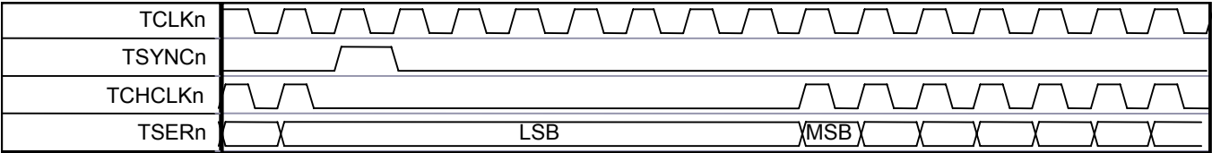
Figure 11-31. E1 Transmit-Side TCHCLKn Gapped Mode During Channel 1
