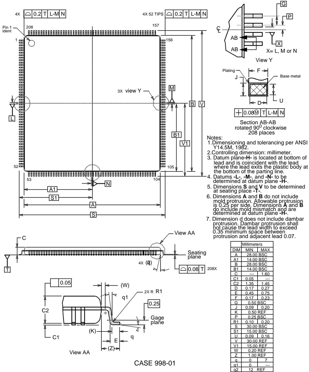
Figure 3-3. DSP56301 Mechanical Information, 208-pin TQFP Package
