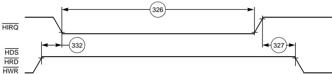
Figure 2-30.  $\overline{\text{HIRQ}}$  Pulse Width ( $\text{HIRH} = 0$ )
