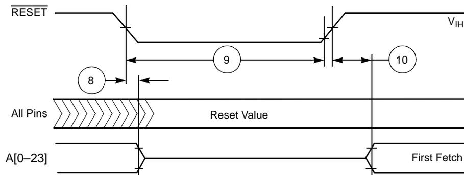
Figure 2-3. Reset Timing
