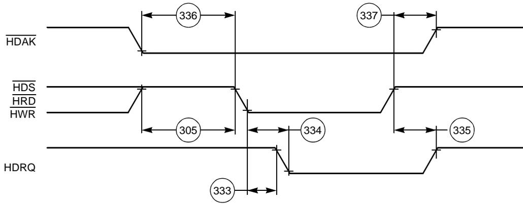
Figure 2-28. Universal Bus Mode DMA Access Timing
