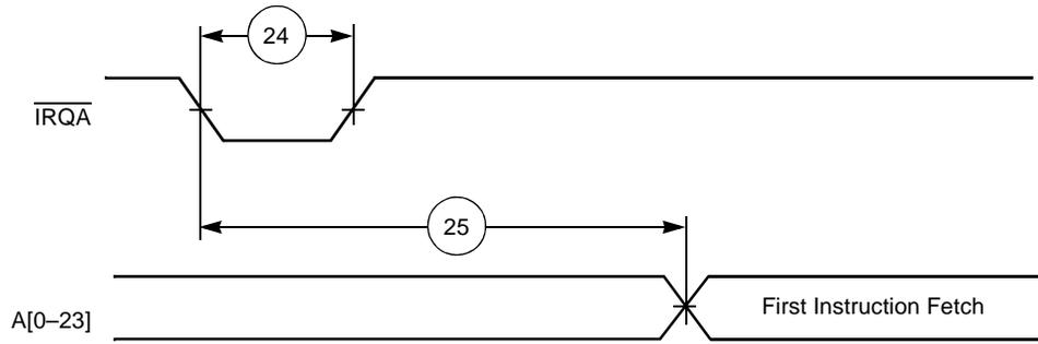
**Figure 2-9.** Recovery from Stop State Using  $\overline{\text{IRQA}}$
