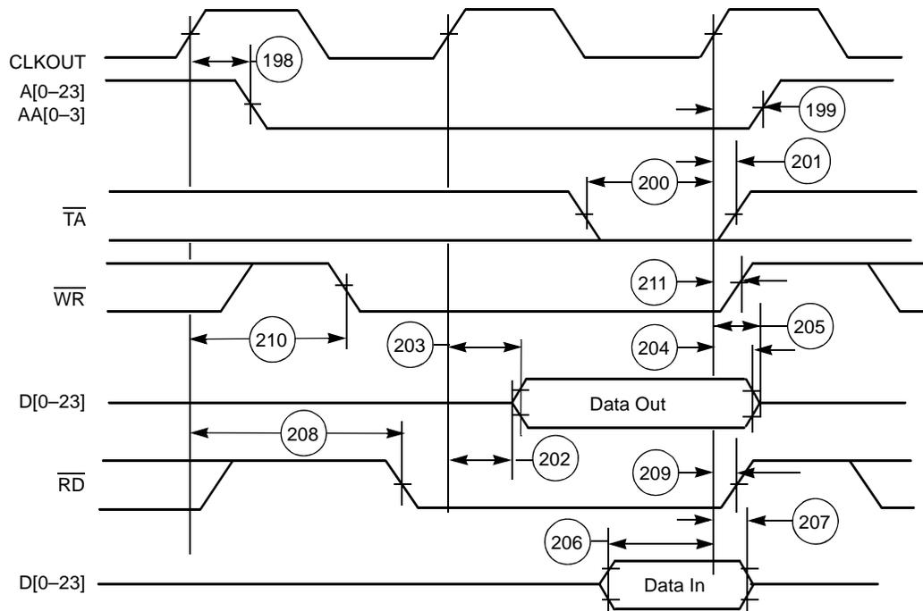
**Note:** Address lines A[0-23] hold their state after a read or write operation. AA[0-3] do not hold their state after a read or write operation.
