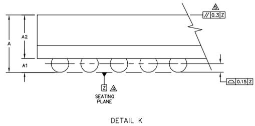
Figure 3-6. DSP56301 Mechanical Information, 252-pin MAP-BGA Package
