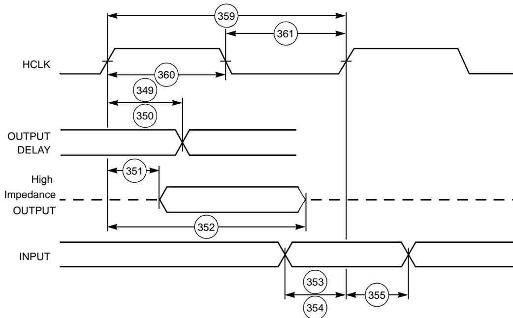
Figure 2-36. PCI Timing
