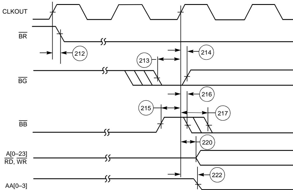
**Note:** Address lines A[0-23] hold their state after a read or write operation. AA[0-3] do not hold their state after a read or write operation.
