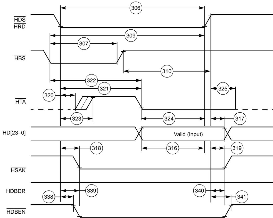
Figure 2-33. Write Timing
