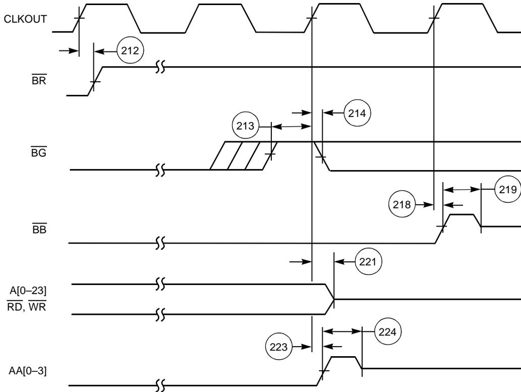
**Note:** Address lines A[0–23] hold their state after a read or write operation. AA[0–3] do not hold their state after a read or write operation.
