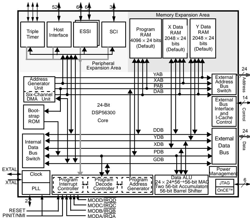
*The DSP56301 is intended for general-purpose digital signal processing, particularly in multimedia and telecommunication applications, such as video conferencing and cellular telephony.*
