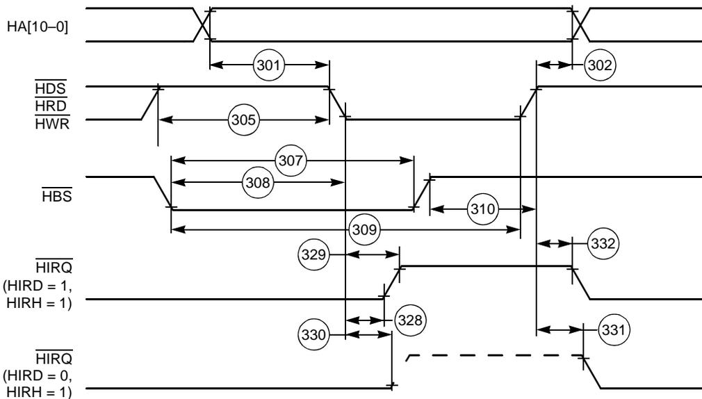
**Figure 2-27.** Universal Bus Mode I/O Access Timing
