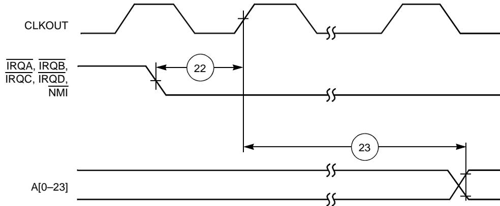
**Figure 2-7.** Synchronous Interrupt from Wait State Timing
