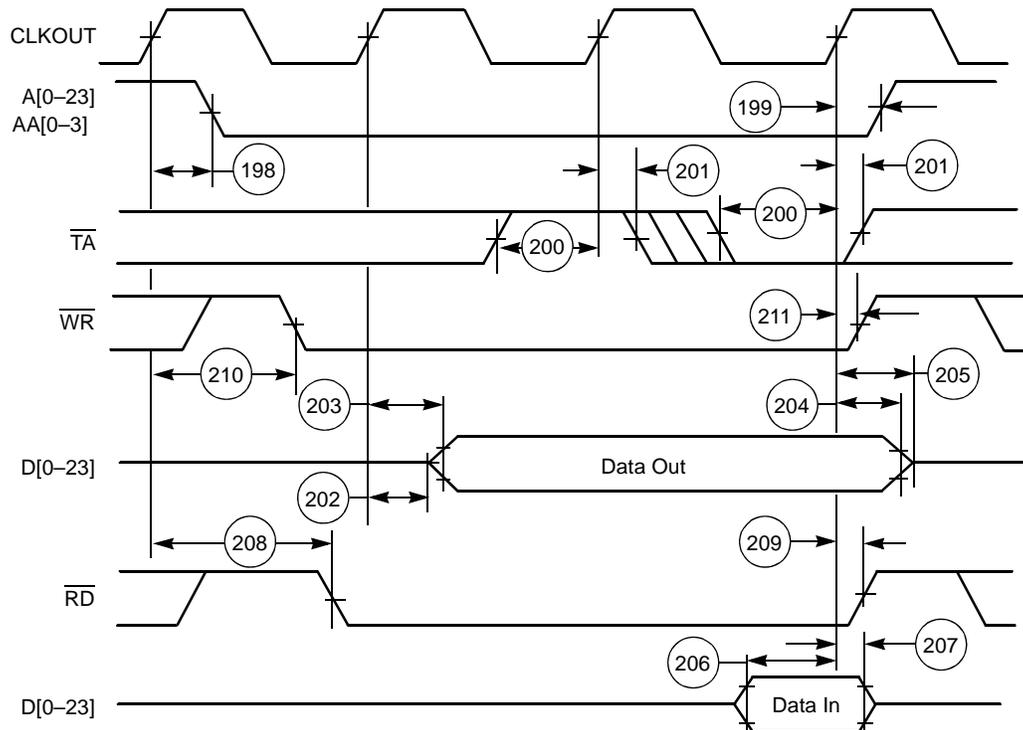
**Note:** Address lines A[0-23] hold their state after a read or write operation. AA[0-3] do not hold their state after a read or write operation.
