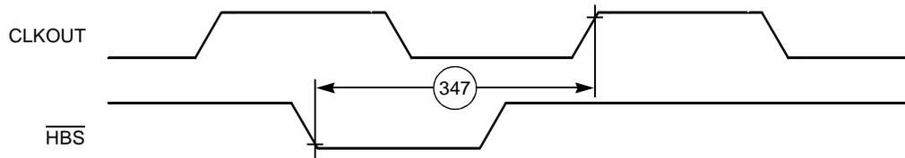
Figure 2-34.  $\overline{\text{HBS}}$  Synchronous Timing
