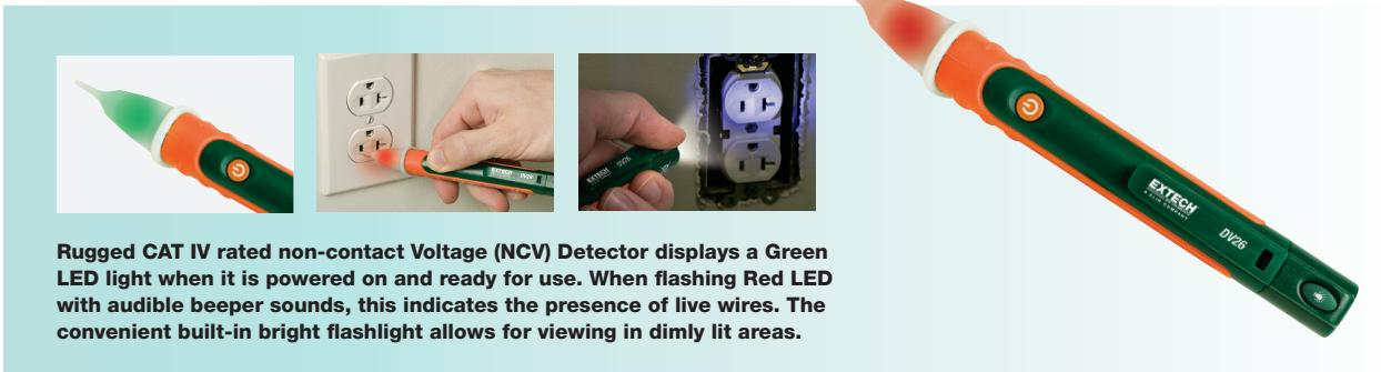
**Rugged CAT IV rated non-contact Voltage (NCV) Detector displays a Green LED light when it is powered on and ready for use. When flashing Red LED with audible beeper sounds, this indicates the presence of live wires. The convenient built-in bright flashlight allows for viewing in dimly lit areas.**
