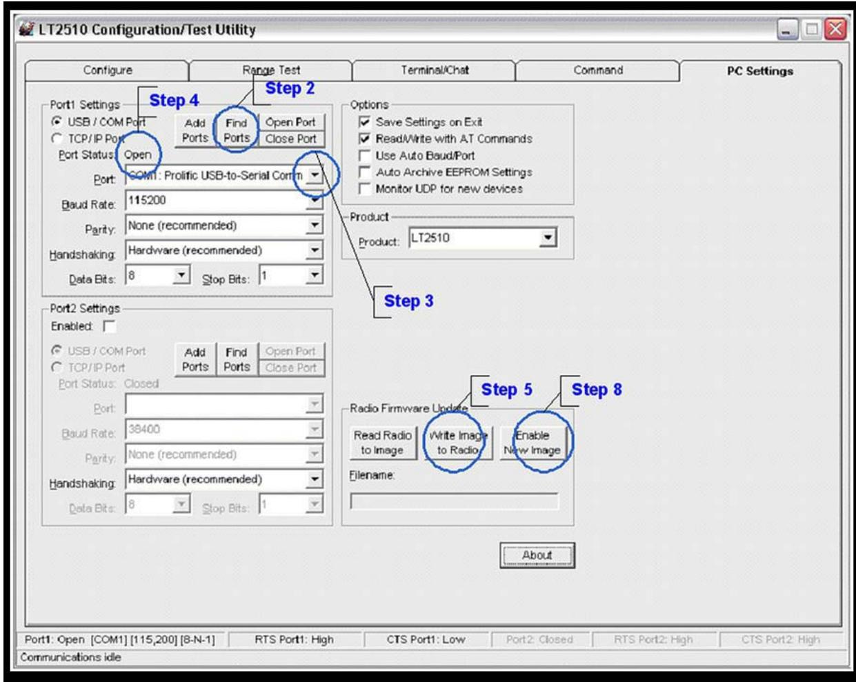
Figure 1: Upgrading firmware in Laird Configuration Utility
