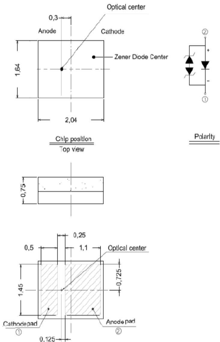
1. Dimensions are in millimeters.
