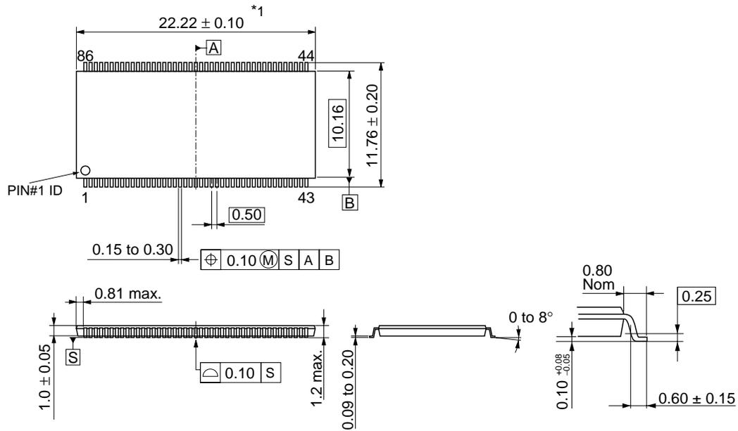
Note: 1. This dimension does not include mold flash, protrusions or gate burrs. Mold flash, protrusions or gate burrs shall not exceed 0.20mm per side.
