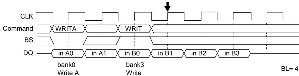
**Write with Auto Precharge to Write Command Interval (Different bank)**
