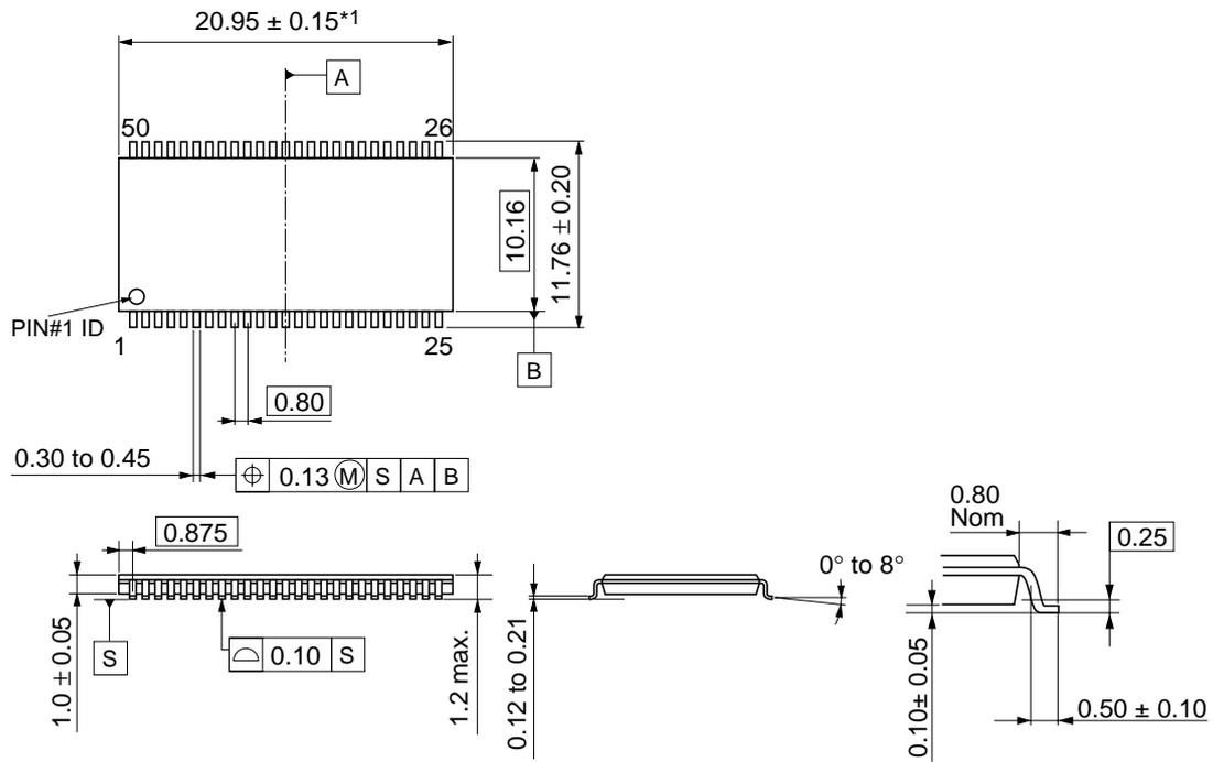
Note: 1. This dimension does not include mold flash, protrusions or gate burrs. Mold flash, protrusions or gate burrs shall not exceed 0.15mm per side.
