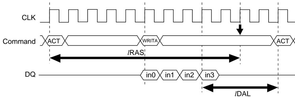
Note: Internal auto-precharge starts at the timing indicated by "↓". and an interval of *tRAS* (*IRAS*) is required between previous active (ACT) command and internal precharge "↓".
