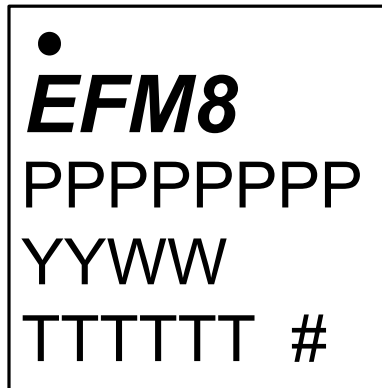
Figure 7.3. QFN32 Package Marking
