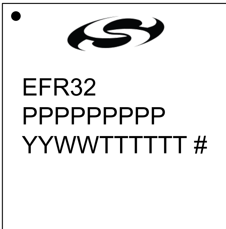
Figure 7.3. QFN48 Package Marking
