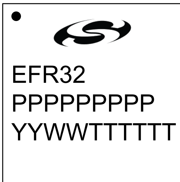
Figure 8.3. QFN32 Package Marking
