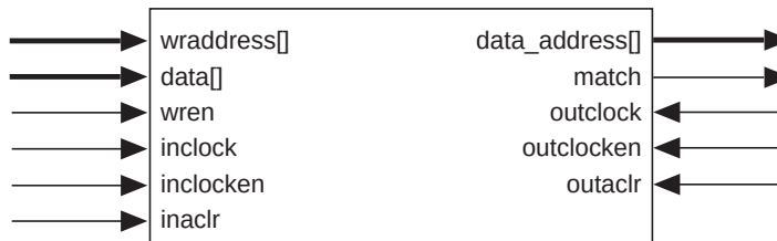
Figure 23. APEX 20KE CAM Block Diagram
